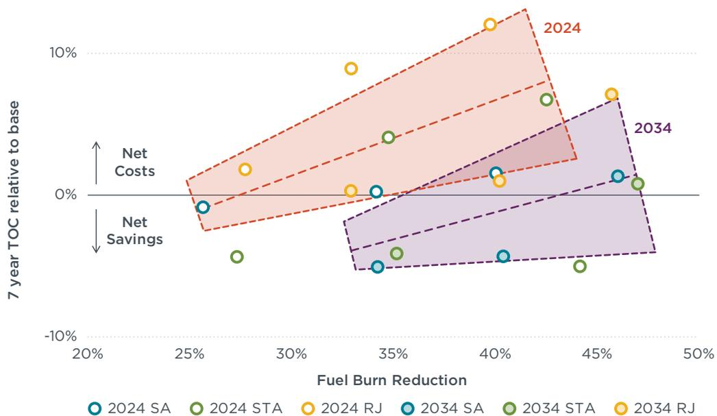
**Figure 8** Seven-year total ownership cost change for all aircraft types and deployment scenarios (Tecolote, 2015)
