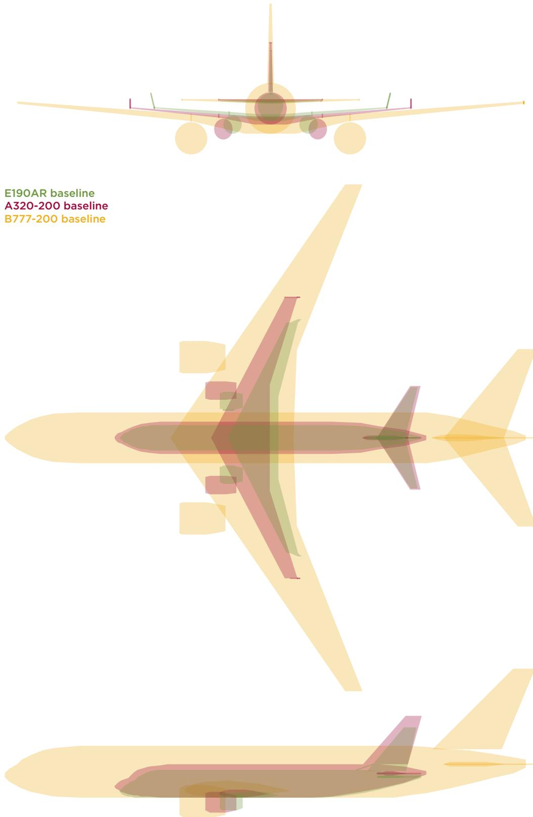
**Figure 2** Piano 5 reference aircraft 3-view
