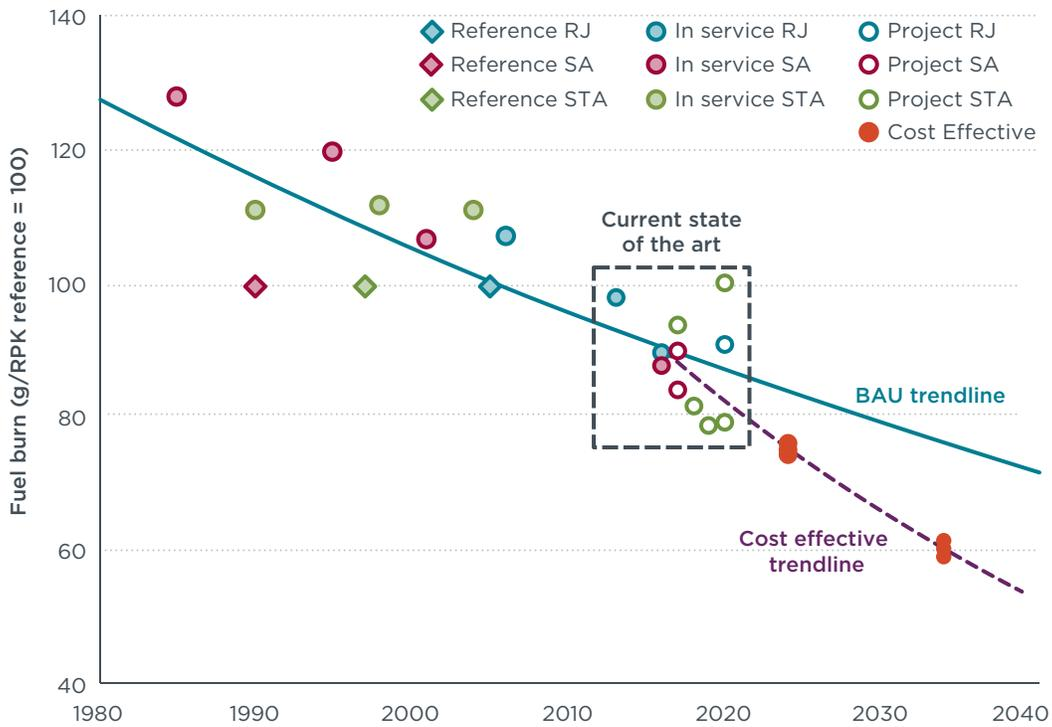
**Figure 9** Trends in new aircraft fuel burn by entry into service year, 1980 to 2040
