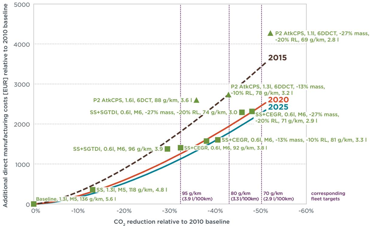
Figure 1. B Class Cost Curve for Petrol Vehicles
