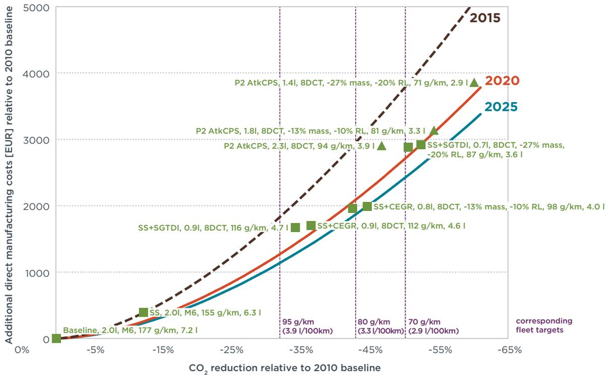
Figure 5. D Class Cost Curve for Petrol Vehicles
