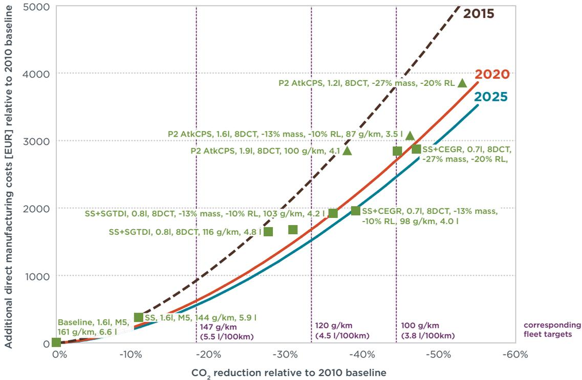
Figure 7. Small N1 Class Cost Curve for Petrol Vehicles
