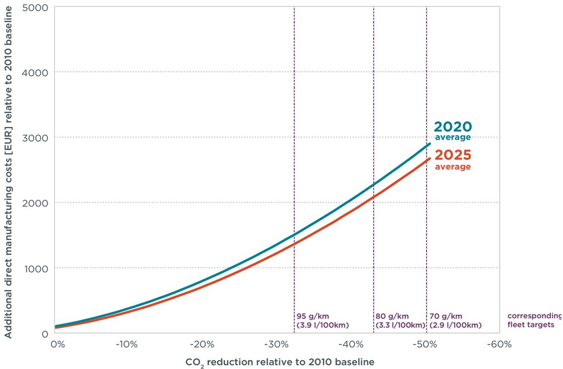
Figure 15. Passenger Vehicle Cost Curves Relative to 2010 EU Baseline
