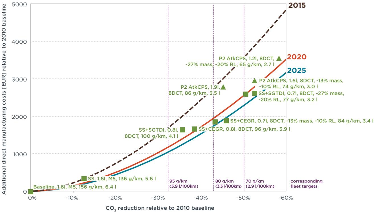
Figure 3. C Class Cost Curve for Petrol Vehicles
