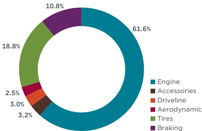
**Figure 5:** Breakdown of energy losses for a tractor truck operating over the WHVC-India cycle
