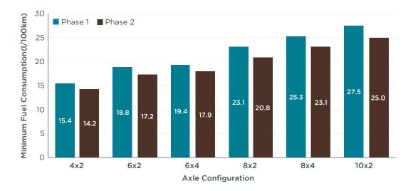
**Figure 1.** Phase 1 and Phase 2 fuel consumption limit values at 40 km/h for N3 rigid trucks by axle configuration
