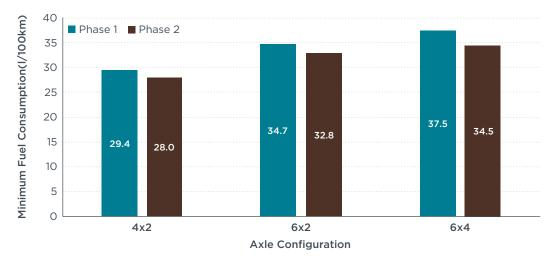
**Figure A2.** Phase 1 and Phase 2 fuel consumption limit values at 40 km/h for N3 tractor-trailers by axle configuration
