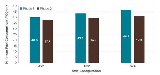
**Figure A3.** Phase 1 and Phase 2 fuel consumption limit values at 60 km/h for N3 tractor-trailers by axle configuration
