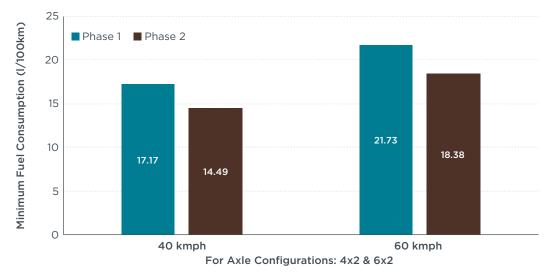
Figure A4. Phase 1 and Phase 2 fuel consumption limit values for M3 buses
