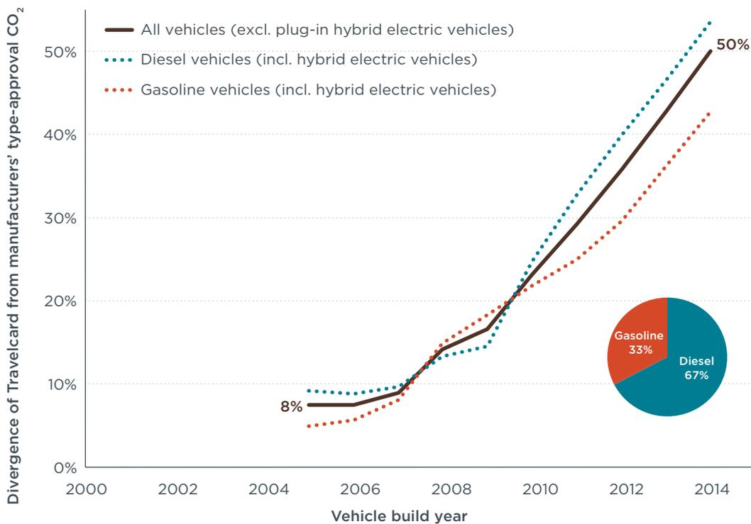
**Figure 11.** Divergence of Travelcard data from manufacturers' type-approval CO<sub>2</sub> emissions by fuel type (pie chart indicates share of vehicles per fuel type in the data set for 2014).
