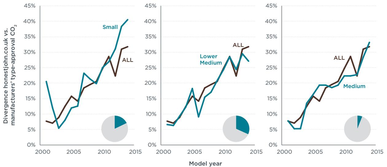
**Figure 17.** Divergence of honestjohn.co.uk data from manufacturers' type-approval CO<sub>2</sub> emissions by vehicle segment (pie chart indicates share of segments in the data set for 2014).
