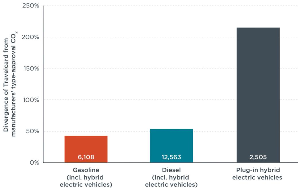
**Figure 12.** Divergence of Travelcard data from manufacturers' type-approval CO<sub>2</sub> emissions for 2014 comparing gasoline and diesel vehicles to plug-in hybrid electric vehicles. Number of Travelcard vehicles per category presented at the base of each bar.
