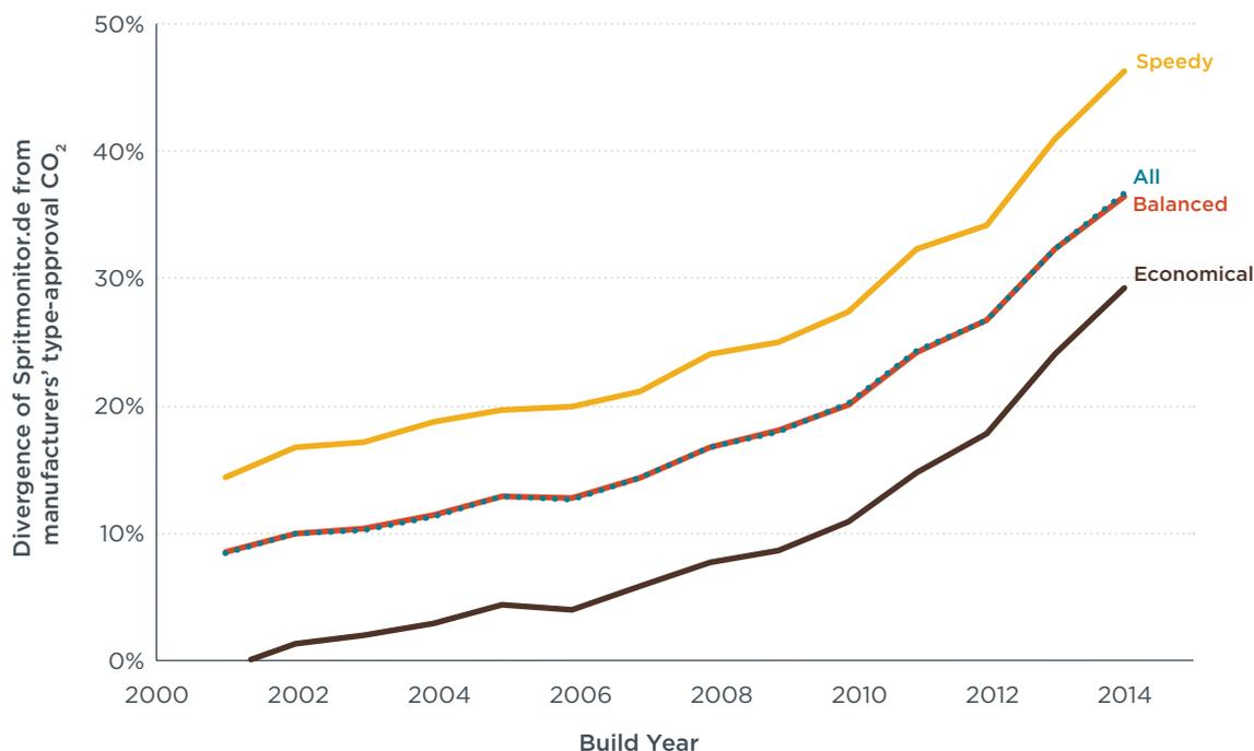
**Figure 28.** Divergence between Spritmonitor.de and type-approval CO<sub>2</sub> values for different driving styles, including *economical*, *balanced*, and *speedy* driving.
