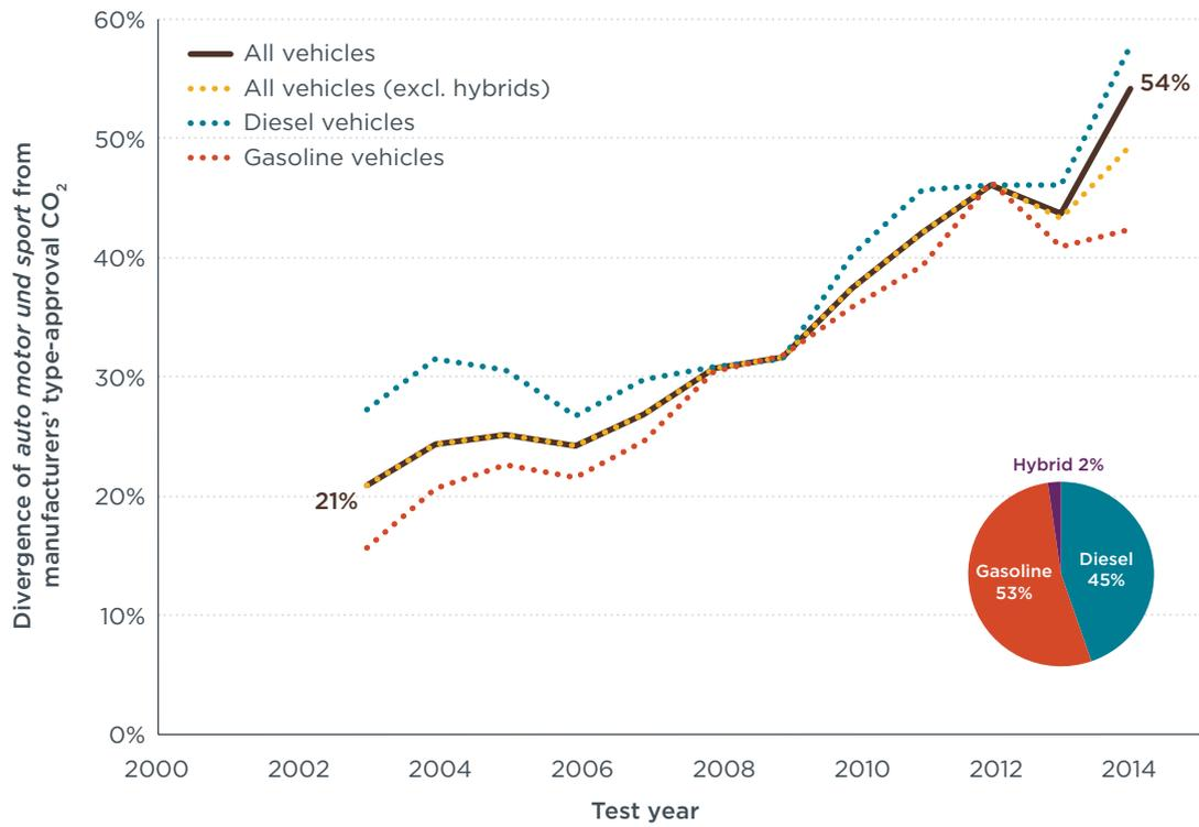
**Figure 21.** Divergence of *auto motor und sport* data from manufacturers' type-approval CO<sub>2</sub> emissions by fuel type (pie chart indicates the share of vehicles per fuel type in the data set for 2014).
