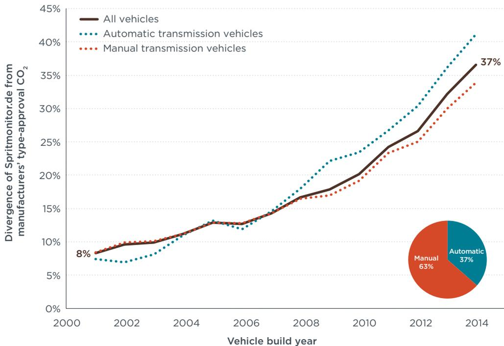
**Figure 6.** Divergence of Spritmonitor.de from manufacturers' type-approval CO<sub>2</sub> emissions by transmission type (pie chart indicates the share of vehicles per transmission type in the data set for 2014).
