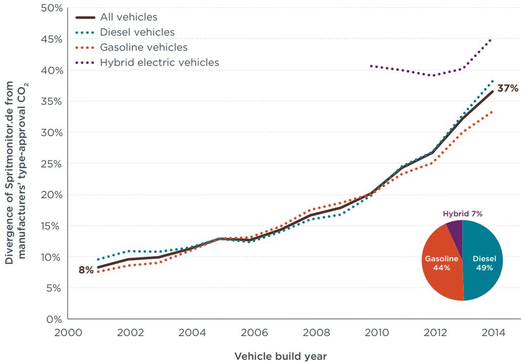
**Figure 5.** Divergence of Spritmonitor.de from manufacturers' type-approval CO<sub>2</sub> emissions by fuel type (pie chart indicates the share of vehicles per fuel type in the data set for 2014).
