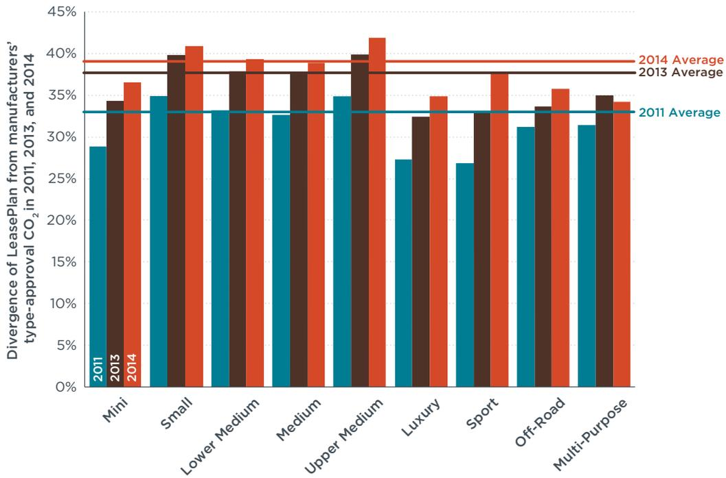
**Figure 14.** Divergence of LeasePlan data from manufacturers' type-approval CO<sub>2</sub> emissions by segments for 2011, 2013, and 2014.
