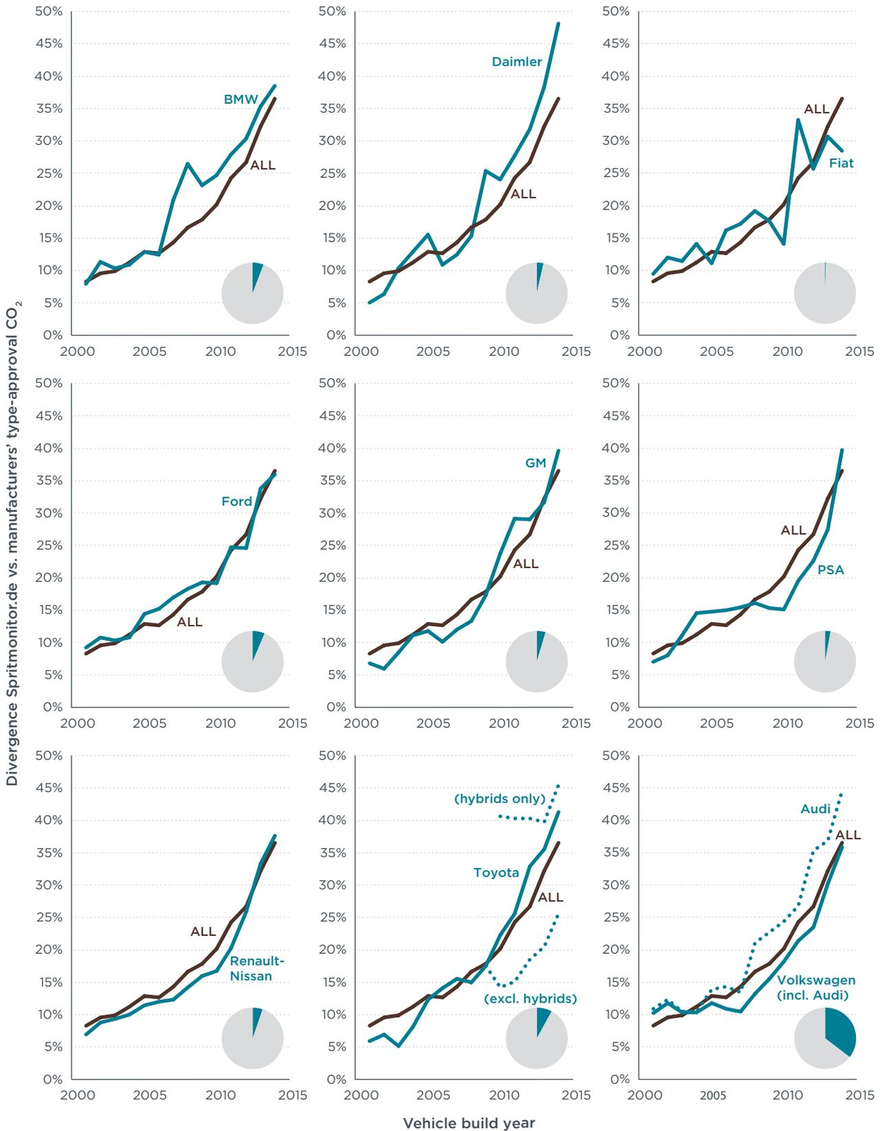
**Figure 8.** Divergence of Spritmonitor.de from manufacturers' type-approval CO<sub>2</sub> emissions by brands/manufacturers (pie chart represents the share of vehicles per manufacturer in the data set for 2014)<sup>11</sup>.
