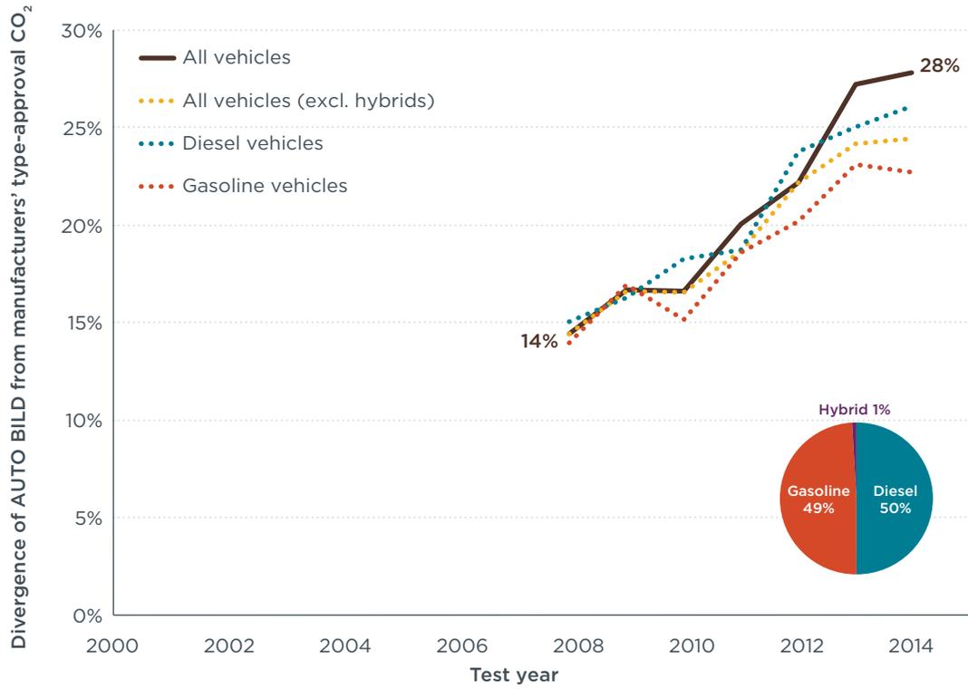
**Figure 19.** Divergence of *AUTO BILD* data from manufacturers' type-approval CO<sub>2</sub> emissions by fuel type (pie chart indicates the share of vehicles per fuel type in the data set for 2014).
