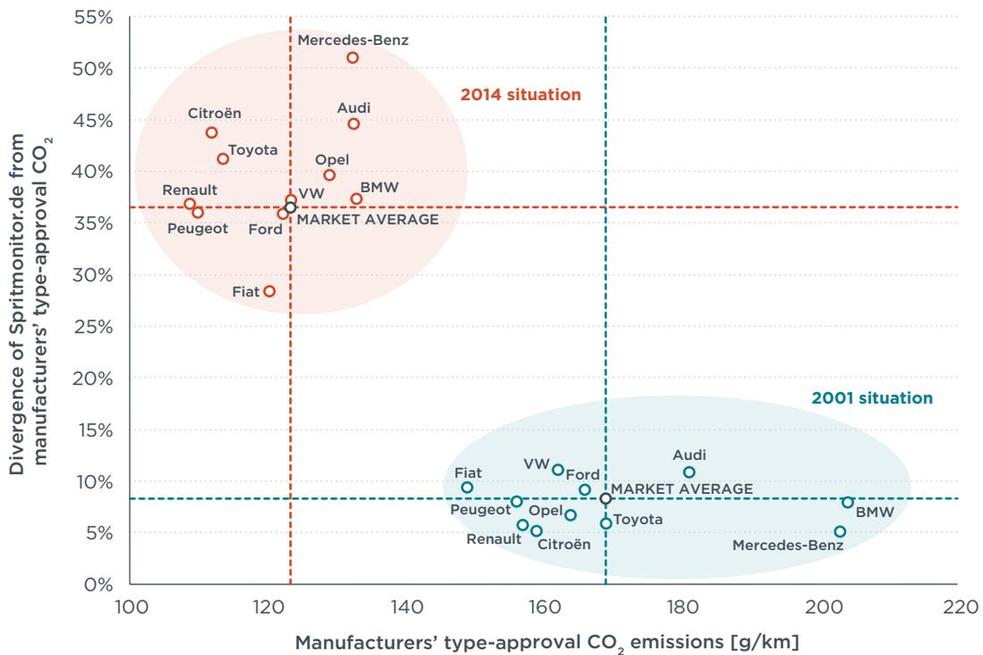
**Figure 32.** Type-approval CO<sub>2</sub> emission values and the corresponding divergence from Spiritmonitor.de for selected brands/manufacturers in 2001 and 2014.
