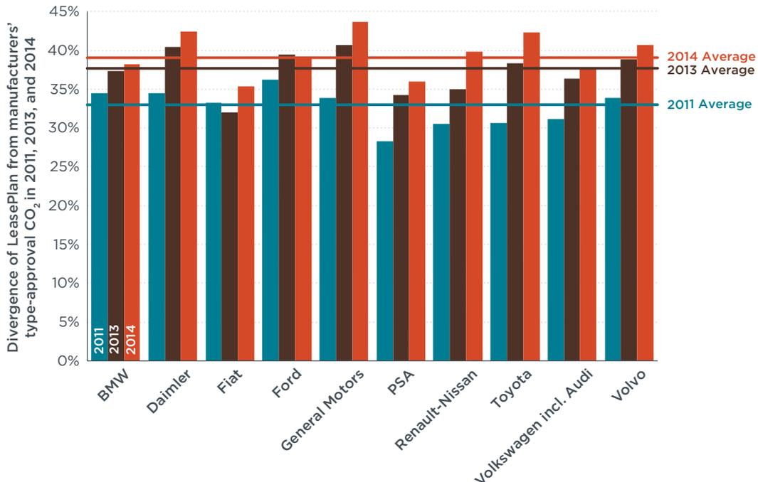
**Figure 15.** Divergence of LeasePlan data from manufacturers' type-approval CO<sub>2</sub> emissions by manufacturer/brand for 2011, 2013, and 2014.<sup>24</sup>
