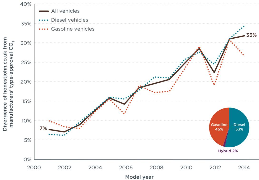
**Figure 16.** Divergence of honestjohn.co.uk data from manufacturers' type-approval CO<sub>2</sub> emissions by fuel type (pie chart indicates share of vehicles per fuel type in the data set for 2014).
