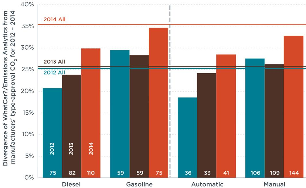
**Figure 20.** Divergence of *WhatCar?*/Emissions Analytics data from official CO<sub>2</sub> emission values for 2012 to 2014 by fuel and transmission type. The number of entries are presented at the base of each column. The average divergence of all vehicles (including hybrids) for each year is also presented.
