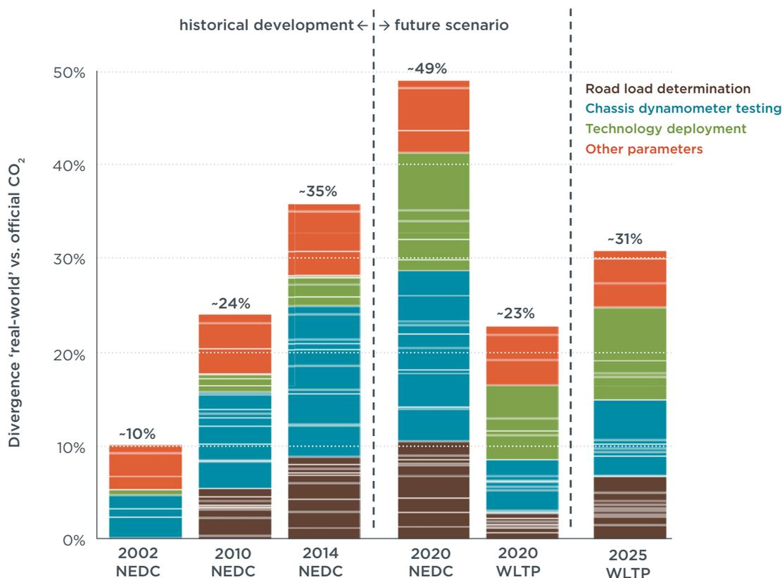
**Figure 29:** Estimate of the reasons for the divergence between type-approval and real-world CO<sub>2</sub> emission levels for new passenger cars in the past as well as in the future, with and without introduction of the WLTP (for details, see Stewart, Hope-Morley, Mock, & Tietge, 2015).
