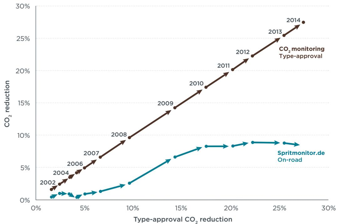
**Figure 31.** Cumulated (2002-2014) real-world vs. type-approval CO<sub>2</sub> reductions in the fleet of new EU passenger cars, based on Spritmonitor.de estimates and EEA type-approval data (European Environment Agency, 2014; European Environment Agency, 2015).
