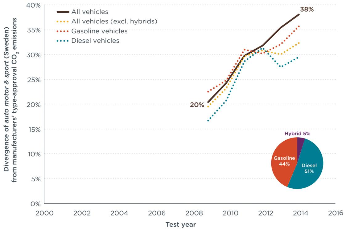
**Figure 22.** Divergence of *auto motor & sport* data from manufacturers' type-approval CO<sub>2</sub> emissions by fuel type (the pie chart presents the share of vehicles per fuel type in the data set for 2014).
