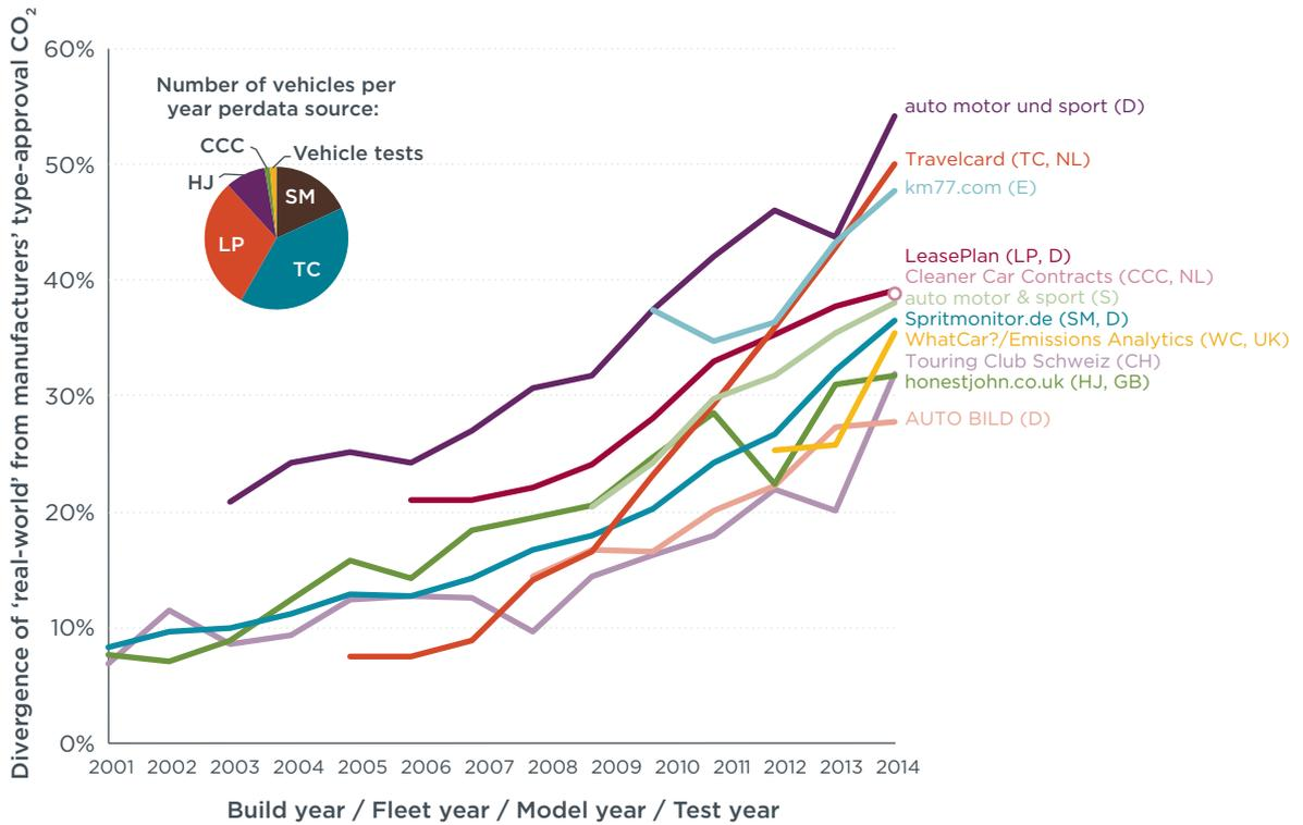
**Figure 25.** Divergence of real-world from manufacturers' type-approval CO<sub>2</sub> emissions for various on-road data sources.
