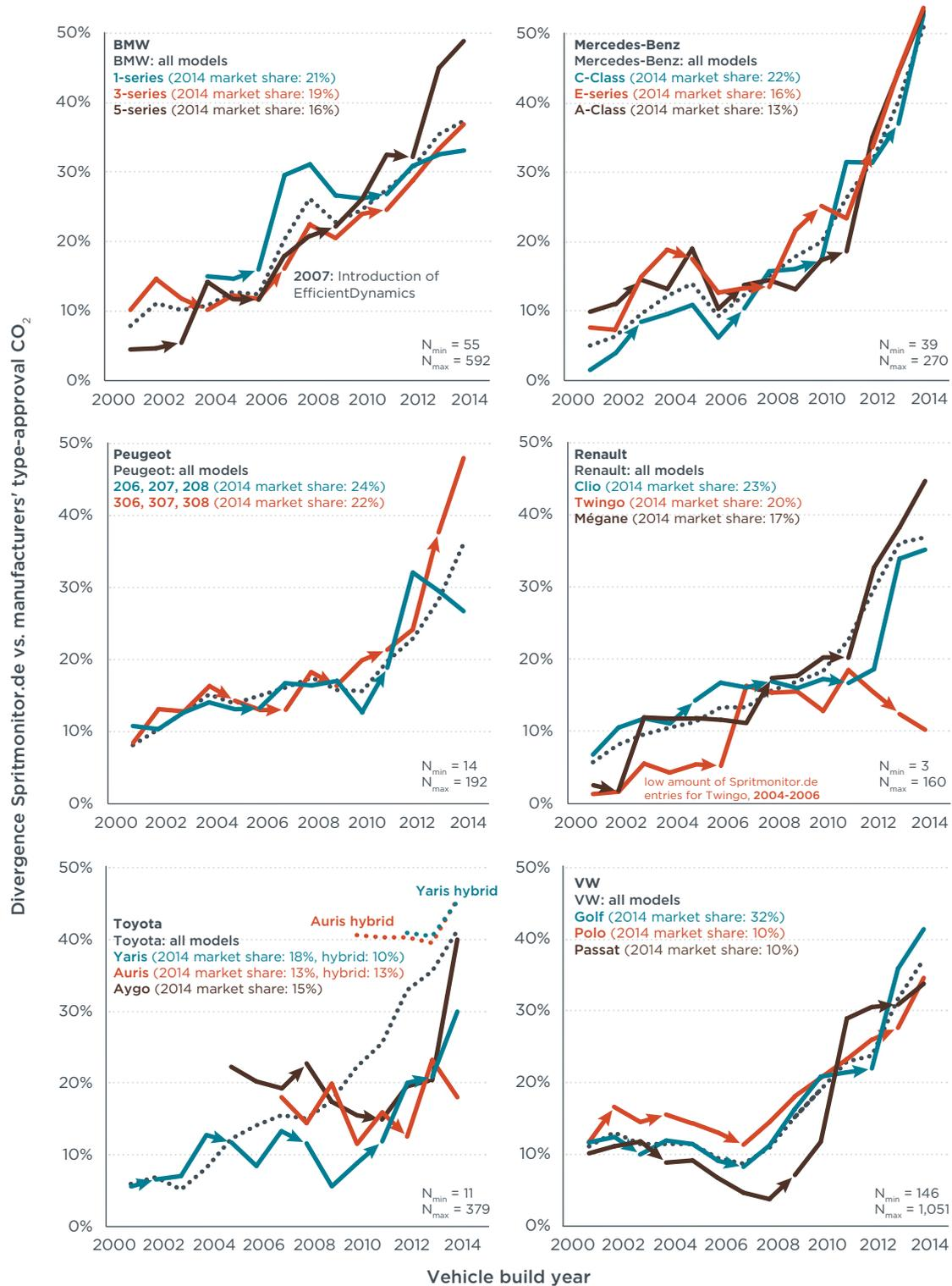
**Figure 9.** Divergence of Spritmonitor.de data from manufacturers' type-approval CO<sub>2</sub> emissions by brand and by top-selling models<sup>14</sup>.
