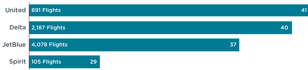
Figure 8. Fuel efficiency in pax-km/L for airlines serving the New York-Santo Domingo routes.
