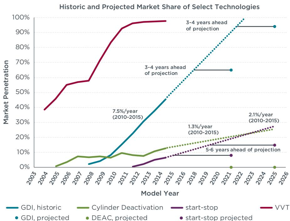
**Figure 4.** Market penetration of select technologies, and extrapolation to rulemaking (RM) projected penetration. Based on U.S. EPA fuel economy trends report for 2015. Note that the 2015 values are estimates.
