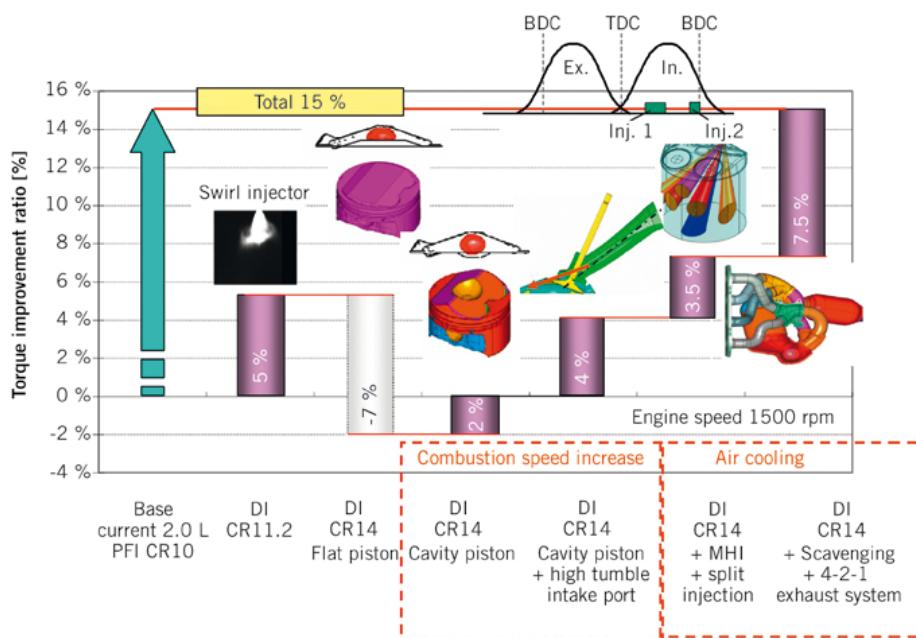
**Figure 1.** Several engine improvements in the Mazda SkyActiv-G lead to a net 15% increase in torque with lower fuel consumption. (Source: Goto et al. "The New Mazda Gasoline Engine Skyactiv-G." MTZ worldwide Issue no.: 2011-06: 40-46.)
