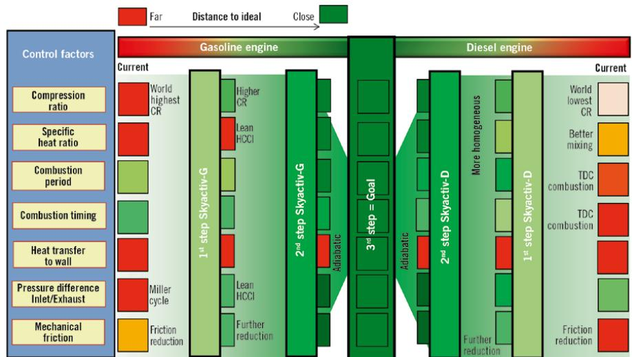
**Figure 3.** Mazda map for incremental improvements in gasoline (and diesel) engines. (Source: Hirose, Ichiro, Hitomi, Mitsuo. "Mazda's Way to More Efficient Internal Combustion Engines.")
