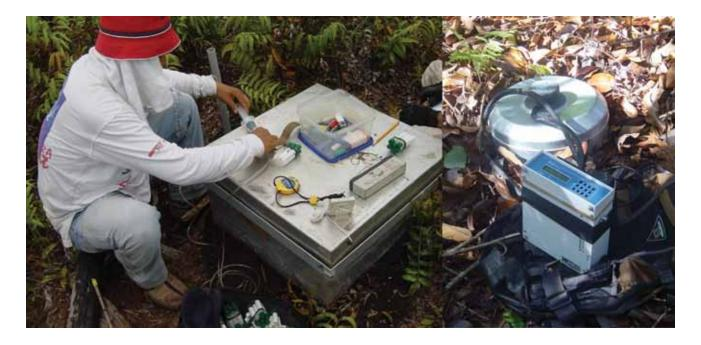
**Figure 7:** Closed chamber measurements being made in the field; large static chamber (left) and dynamic chamber and CO<sub>2</sub> analyzer (right; images: J. Jauhiainen).
