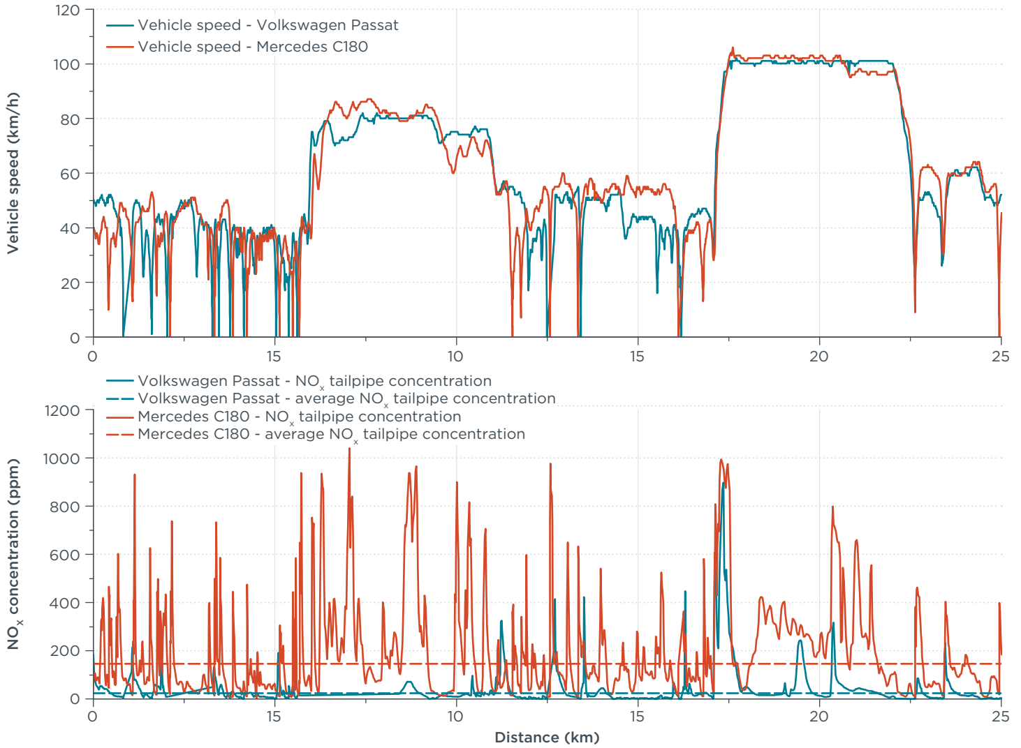
Figure 7: NO x comparison between two Euro 6 diesel vehicles driven on the same route. NO x level measured by installed sensors shows the Mercedes C180 had significantly higher NO x emissions than the Volkswagen Passat.
