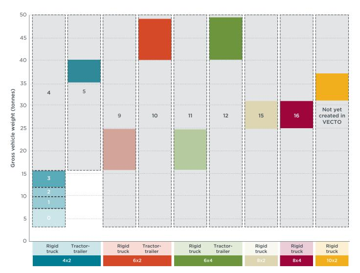
Figure 15. Comparison of the categorization schemes for trucks in VECTO and the current HDV fuel efficiency regulations in India
