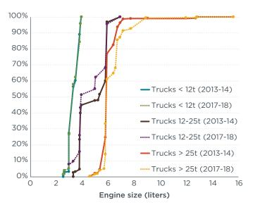
**Figure 8.** Engine size distributions for trucks in the three example vehicle weight categories
