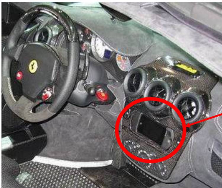
Figure 9.3.1.b: Ferrari iPod Touch integration into the Instrument Panel 27
