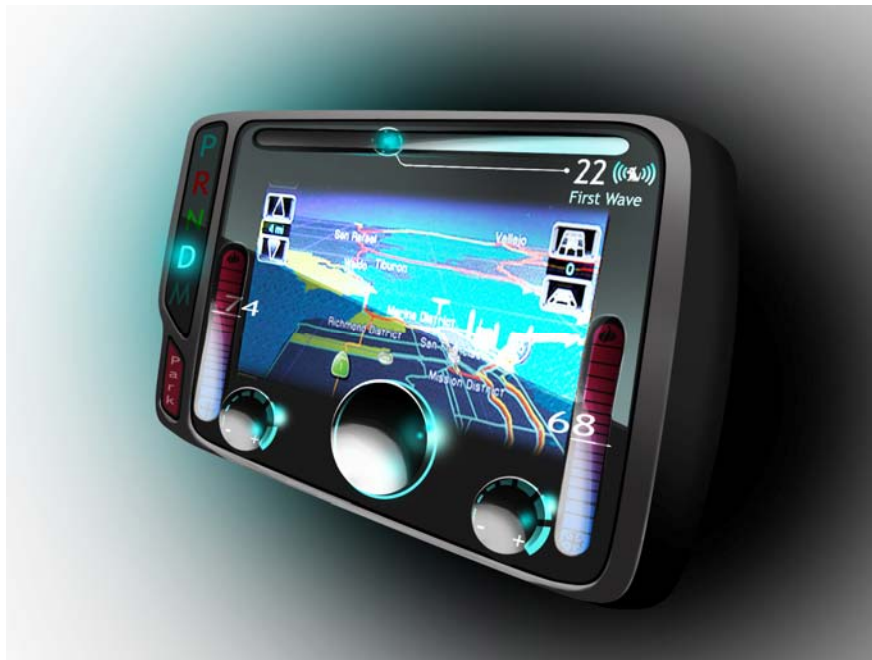
Figure 9.3.3.c: Low Development Central Touch Screen Control Unit
