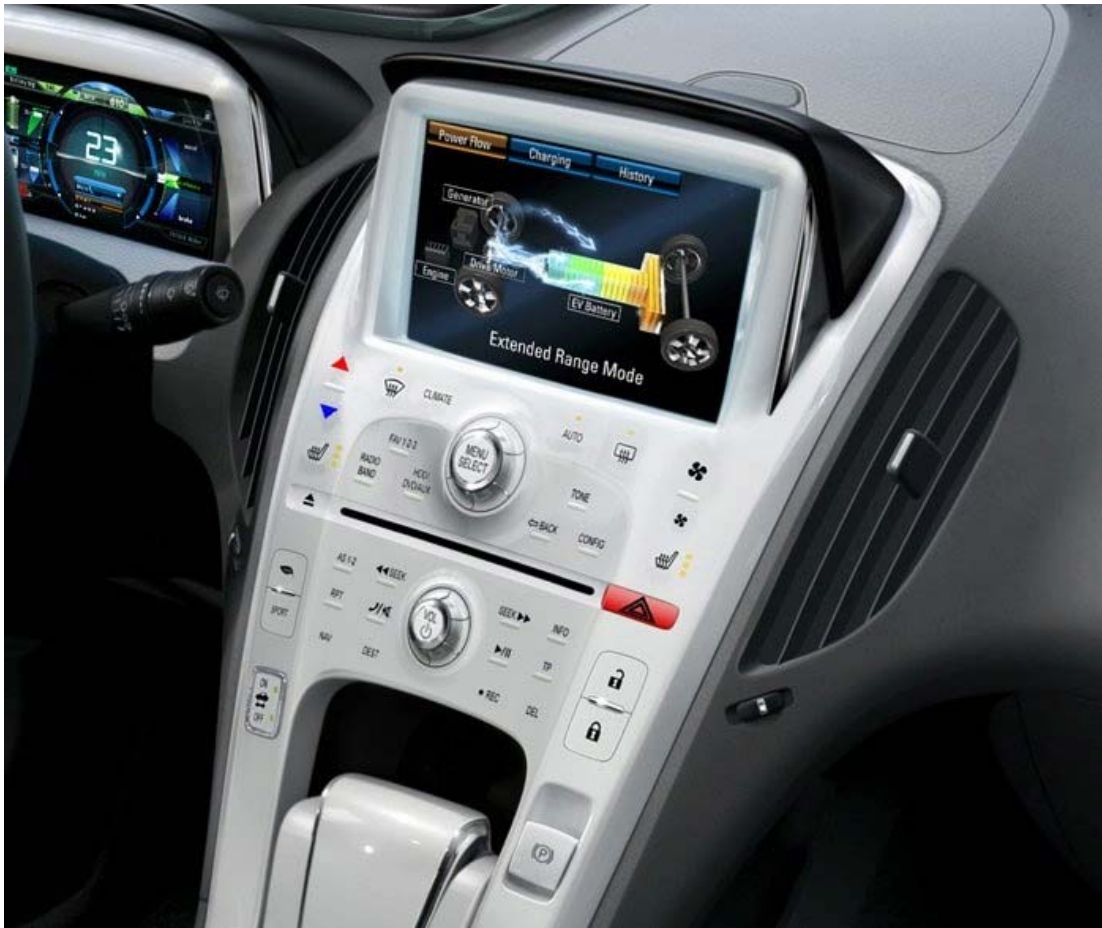
Figure 9.5.1.b: Chevy Volt Capacitive Touch Screen and Center Stack
