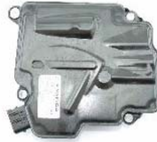
Figure 9.3.1.i: Mercedes S-Class Electronic Shift System
