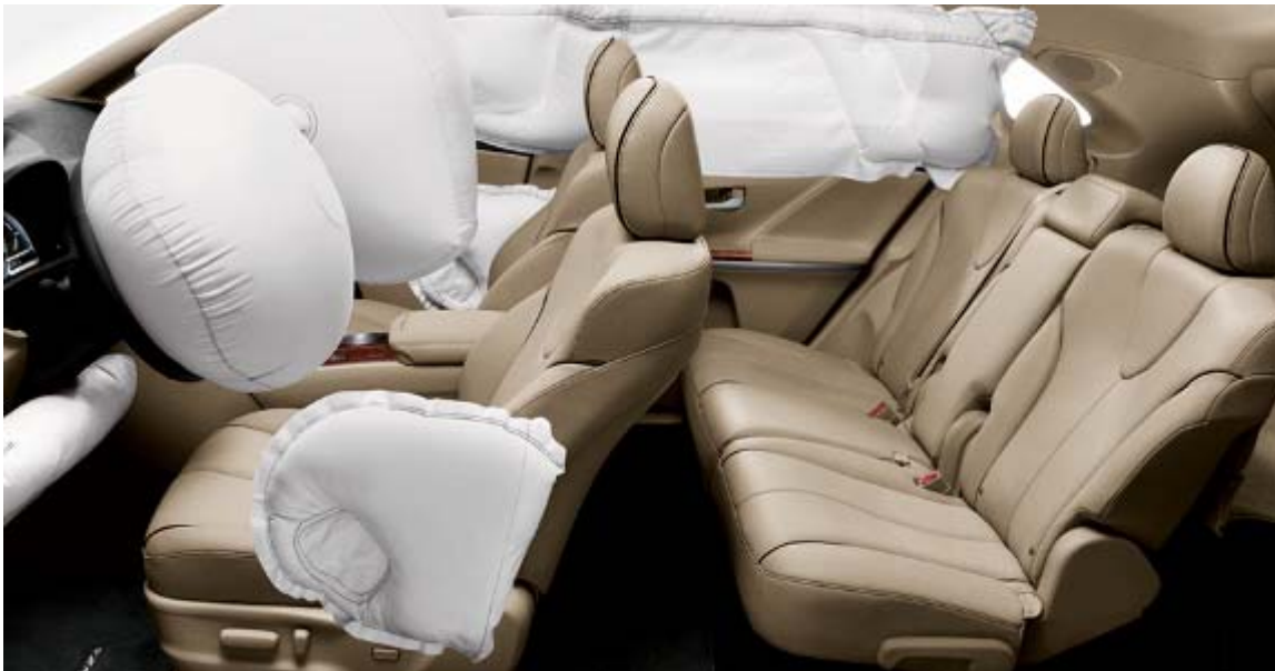
Figure 9.5.4.2.a: Toyota Venza Safety System Coverage
