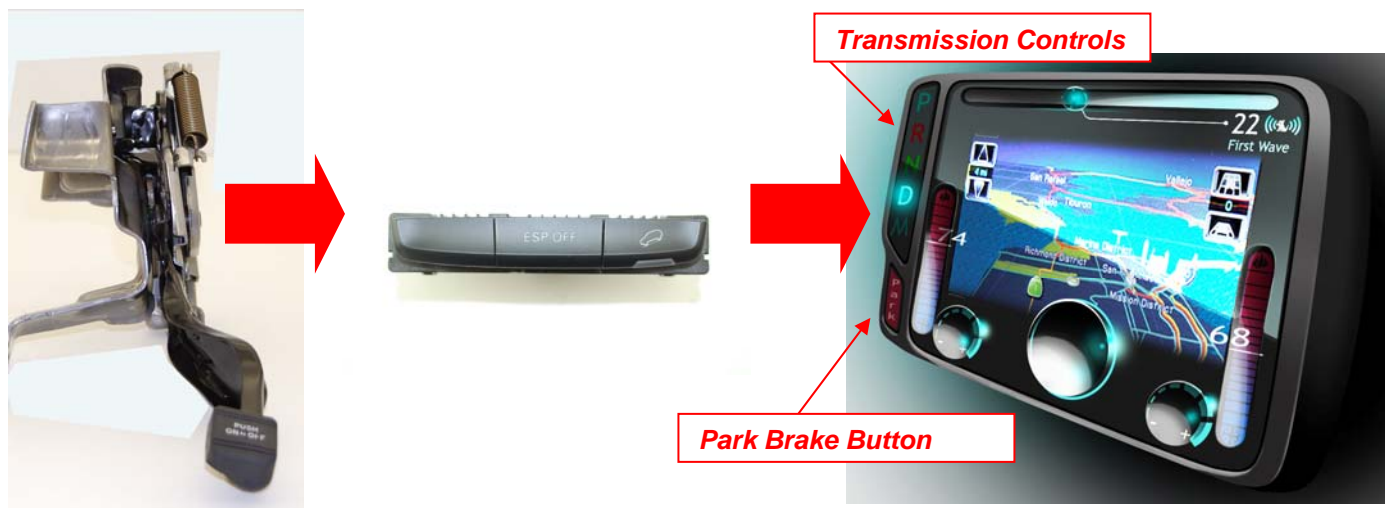
Figure 9.5.3.a Electronic Park Brake Pedal Evolution
