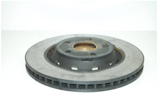
Figure 10.4.2.c.: 2009 Toyota Venza Front Brake Rotor 8.91 kg (Single piece cast iron)
