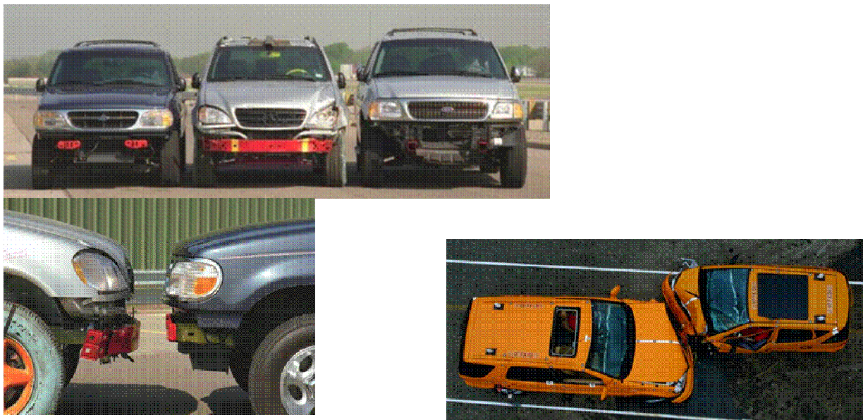
Figure 17.1.t: Vehicle compatibility an important engineering aspect for bumper systems
