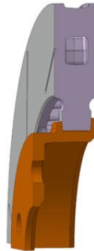
Figure 10.4.2.d.: Brembo Dual Cast Rotor est. 7.15 kg for equivalent design (Cast Aluminum hub with cast iron ring)
