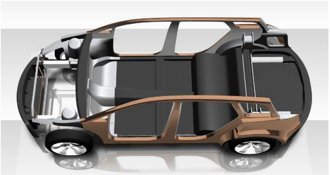
Figure 5.4.3.c: High Development Body In White Structure
