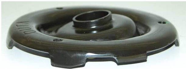
Figure 10.4.1.g.: 2009 Toyota Venza Upper Spring Seat 0.535 kg (Steel)
