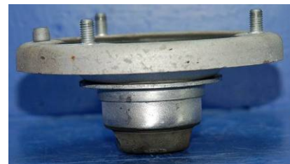
Figure 10.4.1.f.: 2006 BMW 730i Front Mount 0.468 kg/.393 kg normalized (Al shell) 1.20 cost multiplier
