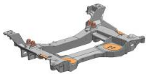
Figure 10.4.1.j.: Cast Magnesium Subframe 15 kg for equivalent part 1.25 cost multiplier
