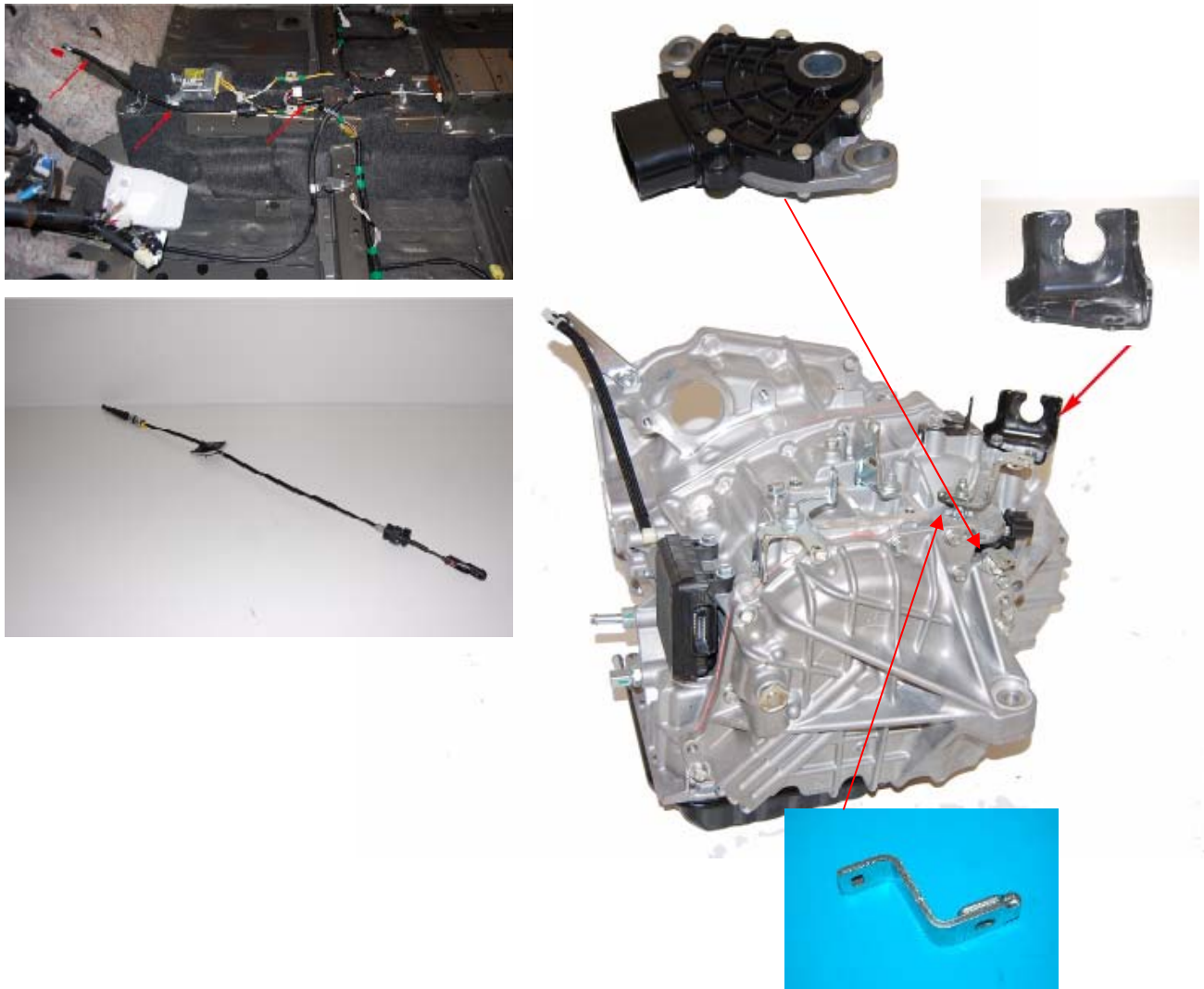
Figure 9.3.3.f: Toyota Venza Transmission Linkages and Actuators
