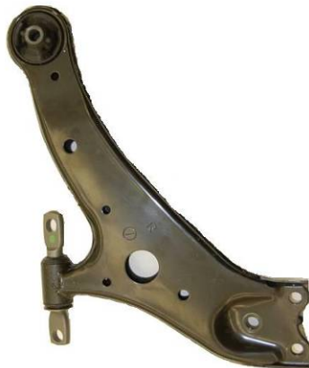
Figure 10.4.2.a.: 2009 Toyota Venza LCA 8.657 kg (Steel)
