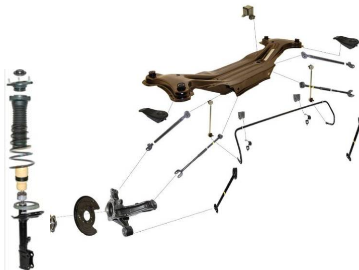
Figure 10.4.1.a.: Front Suspension & Chassis with steering gear
