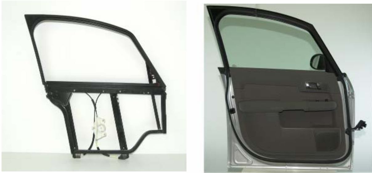
Figure 9.7.1.b Audi A2 Door Module and Upper Trim
