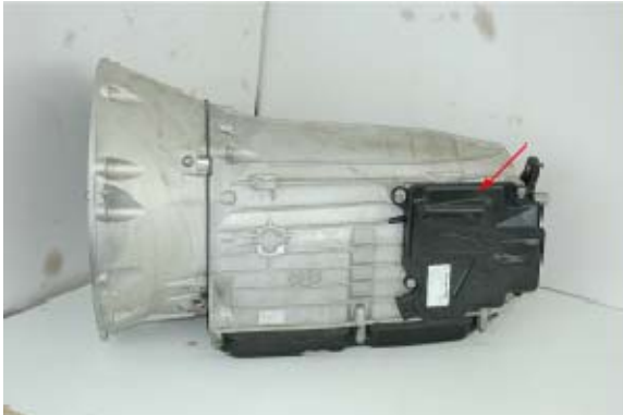
Figure 9.3.1.i: Mercedes S-Class Electronic Shift System
