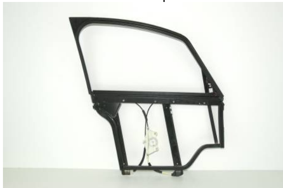
Figure 6.4.2.b: Audi A2 window regulator module
