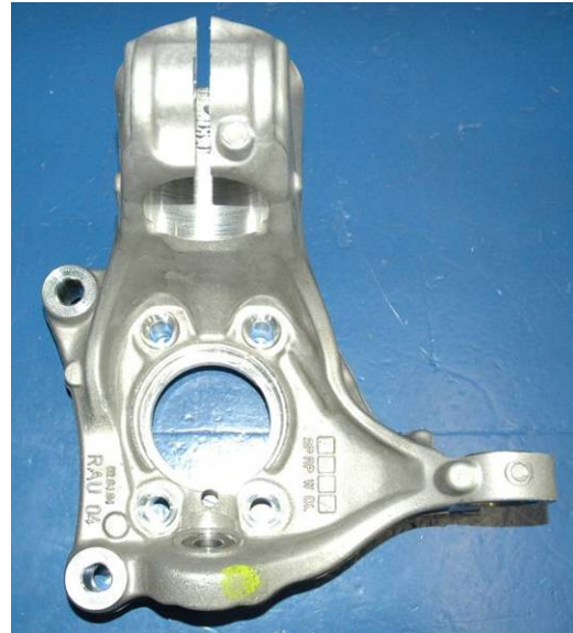
Figure 10.4.1.m.: 2005 Passat Front Knuckle 3.012kg/3.28 kg normalized(Cast Al)
