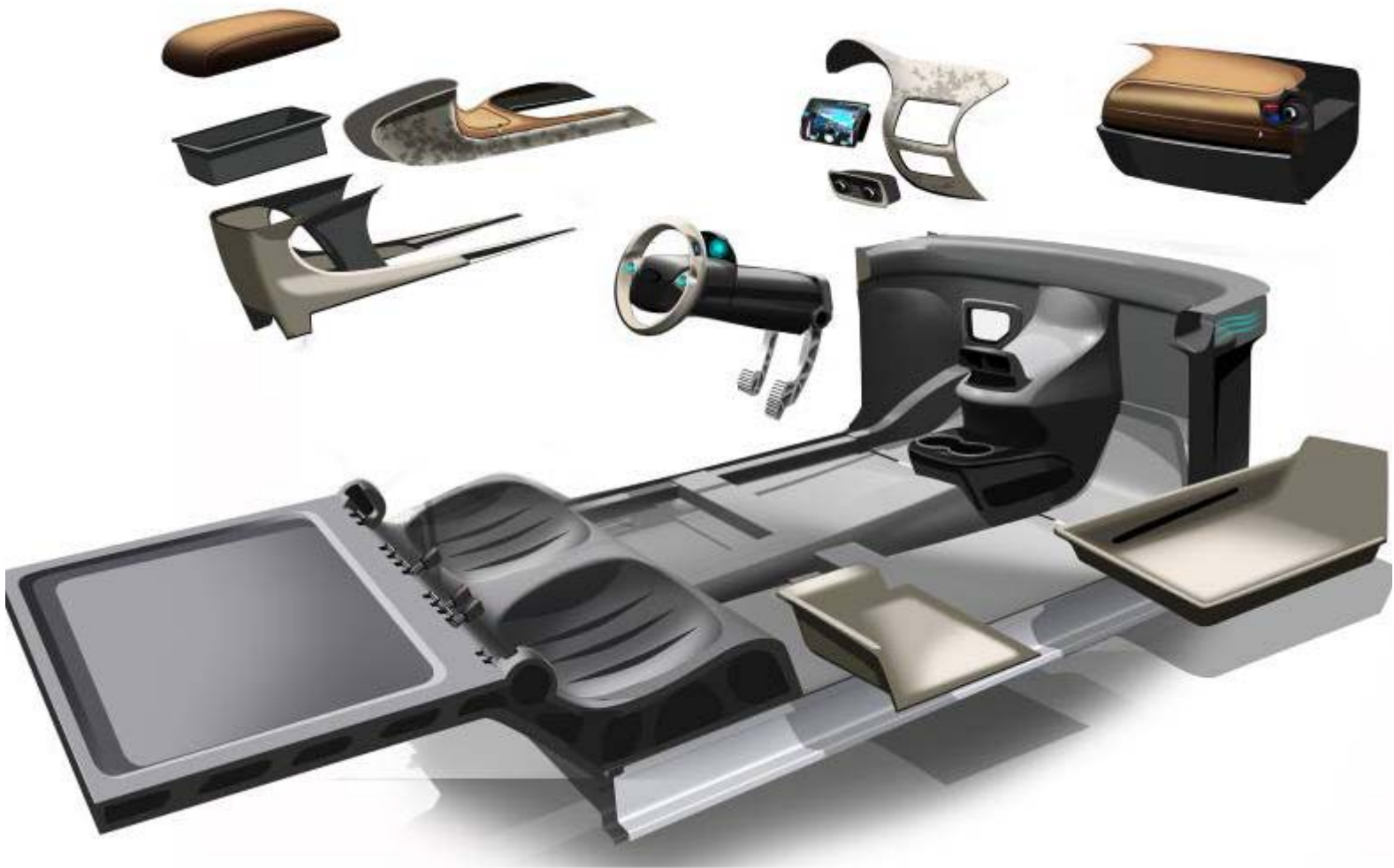
Figure 9.3.4.2.i High Development Instrument Panel Concept Assembly
