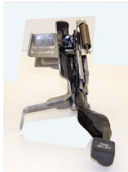
Figure 9.5.2.b: Audi Q5 vs. Toyota Venza Pedal Assemblies
