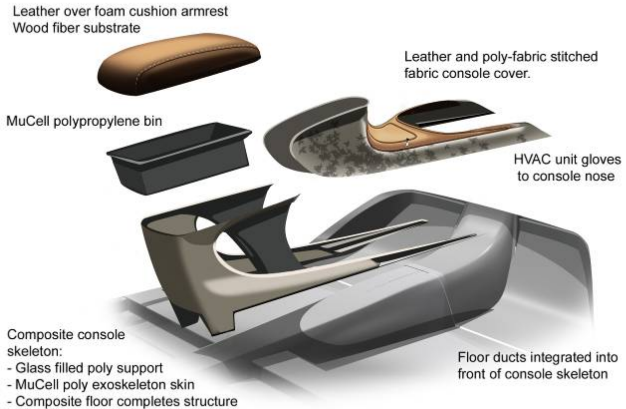
Figure 9.3.3.I High Development Center Console Exploded View
