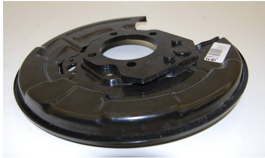
Figure 10.4.1.n.: Toyota Venza Rear Heat shield
