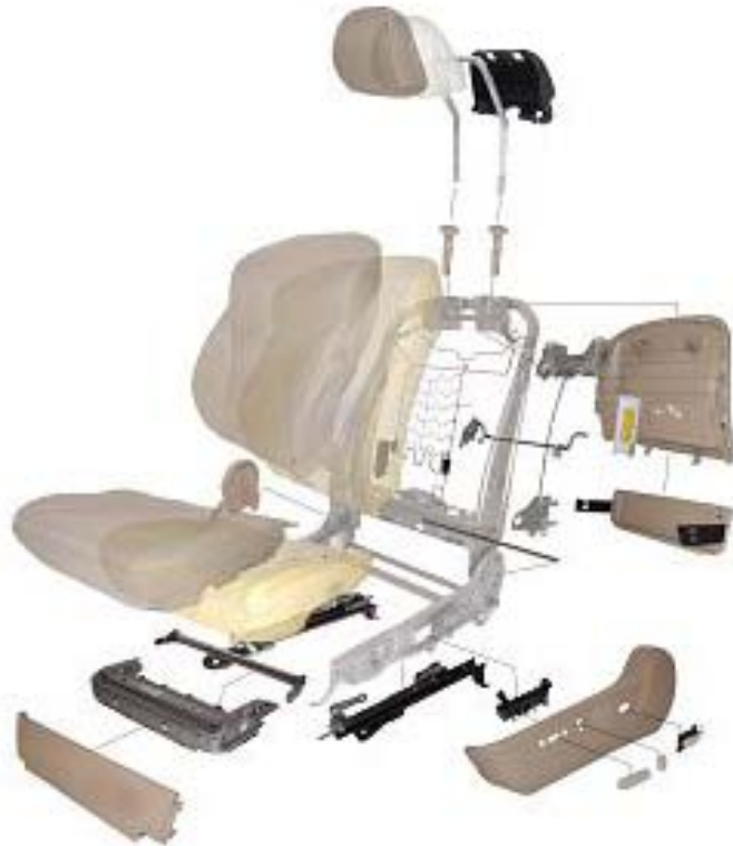
Figure 9.2.4.a: Exploded View of Toyota Venza Driver's Seat
