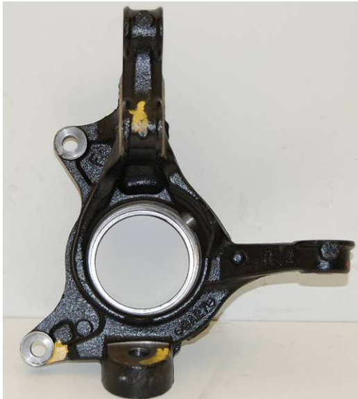
Figure 10.4.1.l.: Venza Front Knuckle 5.945 kg (Cast Iron)
