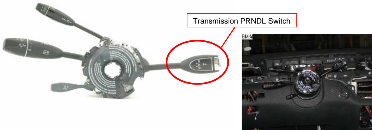
Figure 9.3.1.k Mercedes S-Class Electronic Shift Interior Stalk Switch
