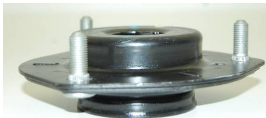
Figure 10.4.1.e.: 2009 Toyota Venza Front Mount 1.233 kg (Steel shell)
