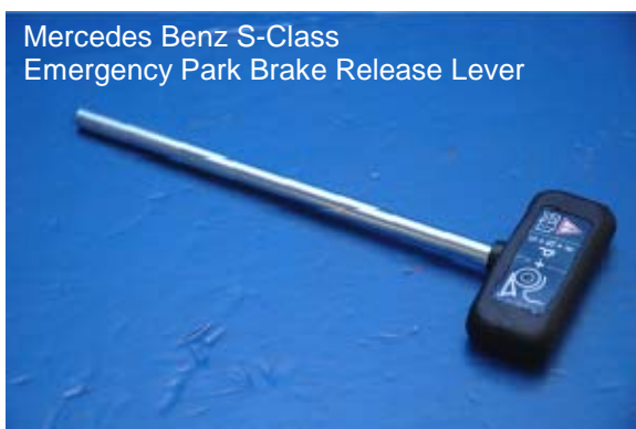
Figure 9.5.2.c: Mercedes-Benz S-Class LCD Control and Emergency Park Brake Release
