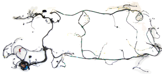
Photograph of Toyota Venza Sub system body harness (not complete)
