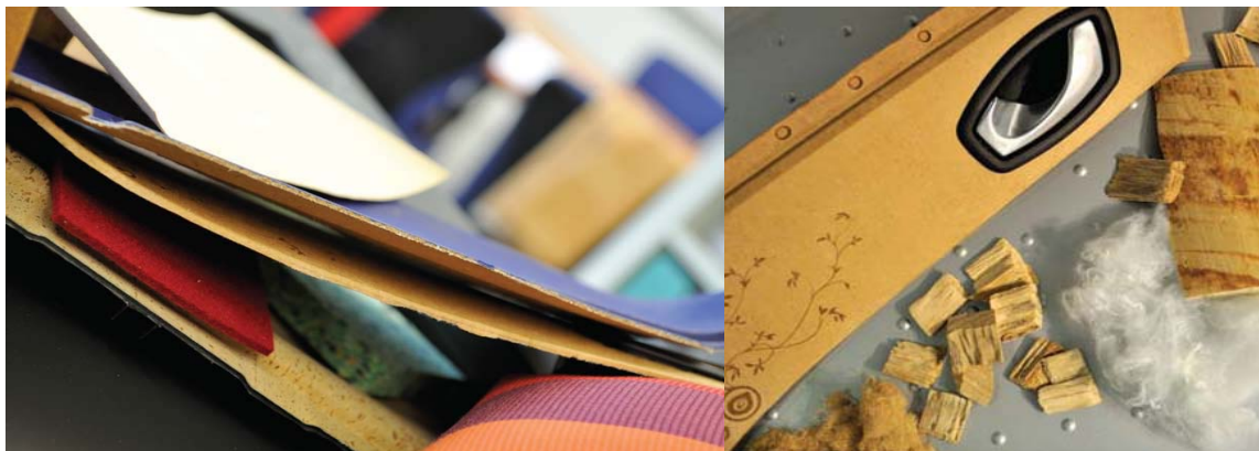
Figure 9.4.1.b: Wood Fiber Hard Trim Examples (From the Faurecia Light Attitude Study Report)
