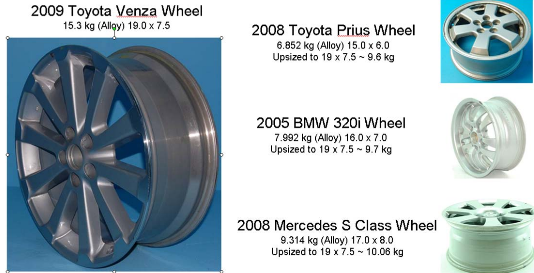
Figure 10.4.1.x.: Venza Wheel shown along with some sample low mass wheel designs.
