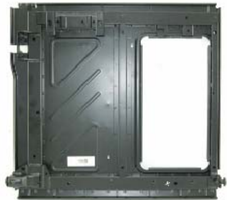
Figure 9.2.2.i: Audi A6 Stamped Steel Seat Frame
