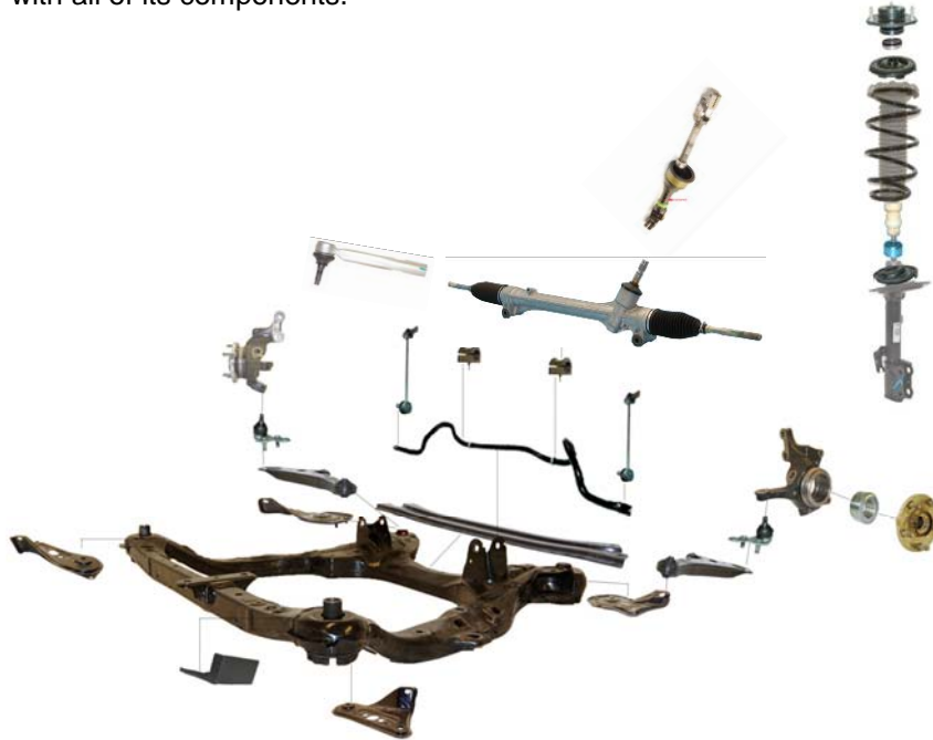
Figure 10.4.1.a.: Front Suspension & Chassis with steering gear
