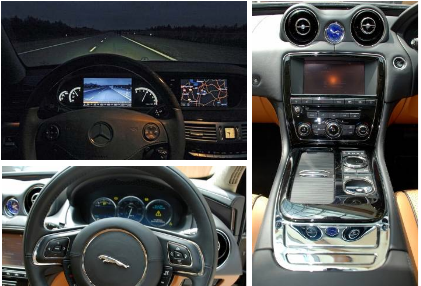
Figure 9.3.1.c: Mercedes-Benz S-Class (2006) and Jaguar XJ (2010) LCD Cluster, Touch Screen and Information systems 28
