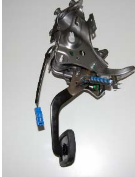
Toyota Venza Park Brake 3.191 kg -- Park Brake Pedal Assembly
