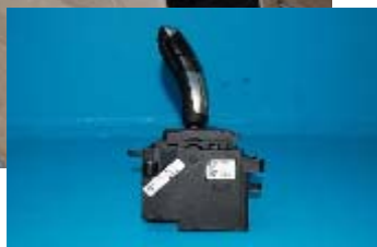
Figure 9.3.1.h: BMW 7-Series Mechanical-Electrical Shift System
