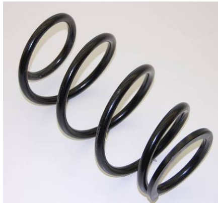
Figure 10.4.1.c.: 2009 Toyota Venza Front Spring 3.26 kg
