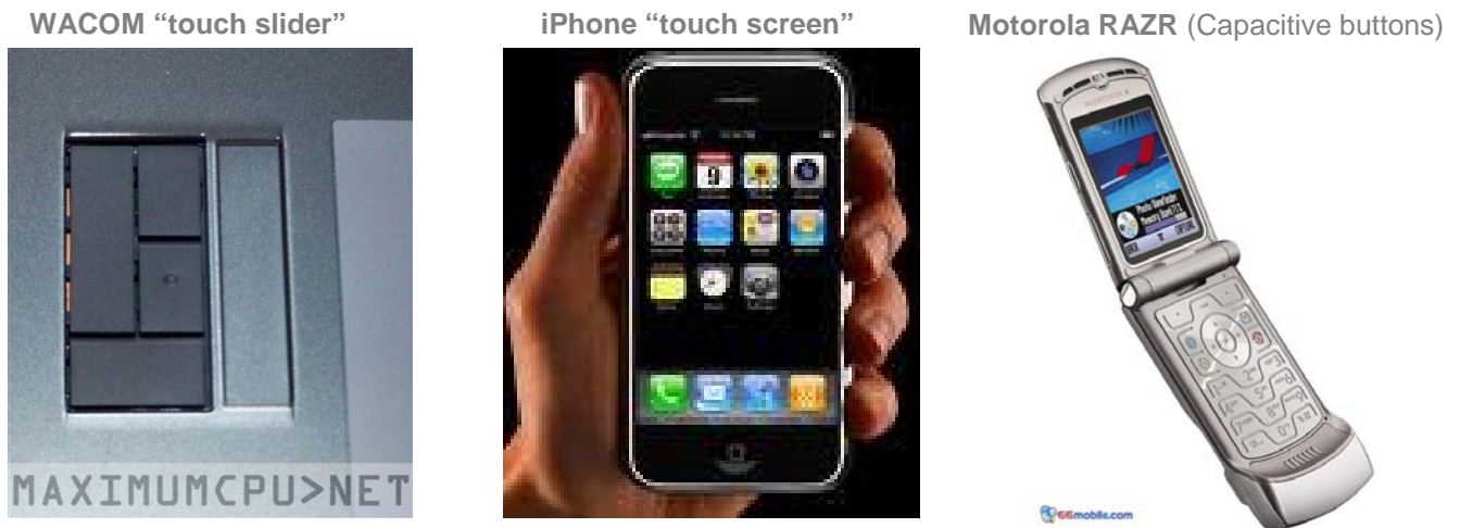
Figure 9.5.1.a: WACOM Tablet (Capacitive Slider Switch), iPhone (touch screen) and RAZR Phone
