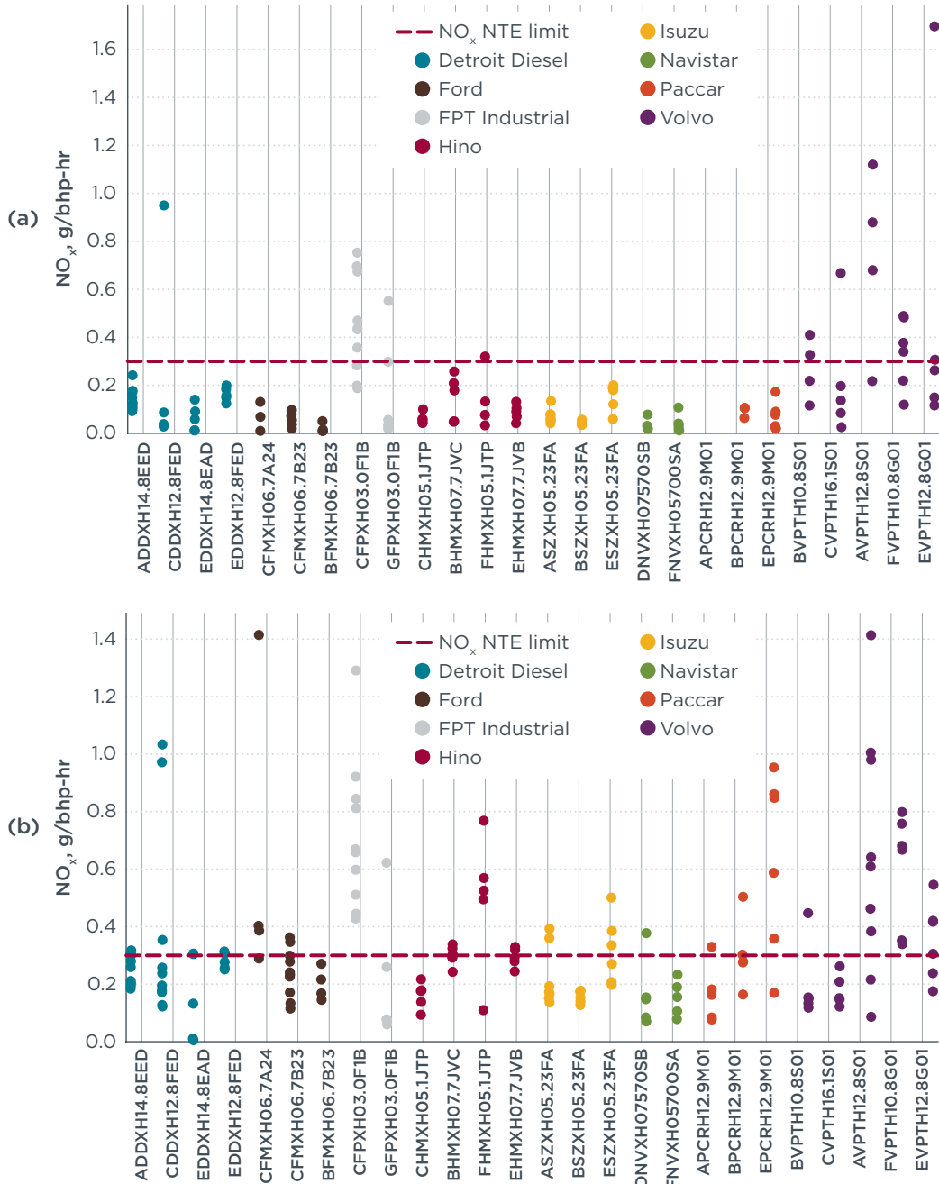
Figure 5 Engine family NO x emissions reported from (a) NTE data from HDIUT, and (b) calculated from route analysis (no data exclusions) of PEMS tests
