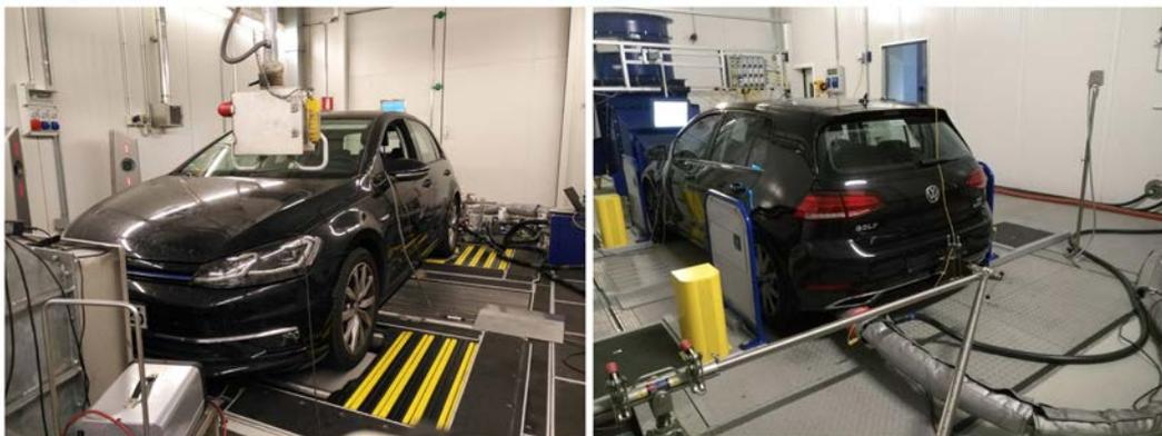
**Figure 1.** Volkswagen Golf 1.5 TSI ACT BlueMotion on JRC's chassis dynamometer
