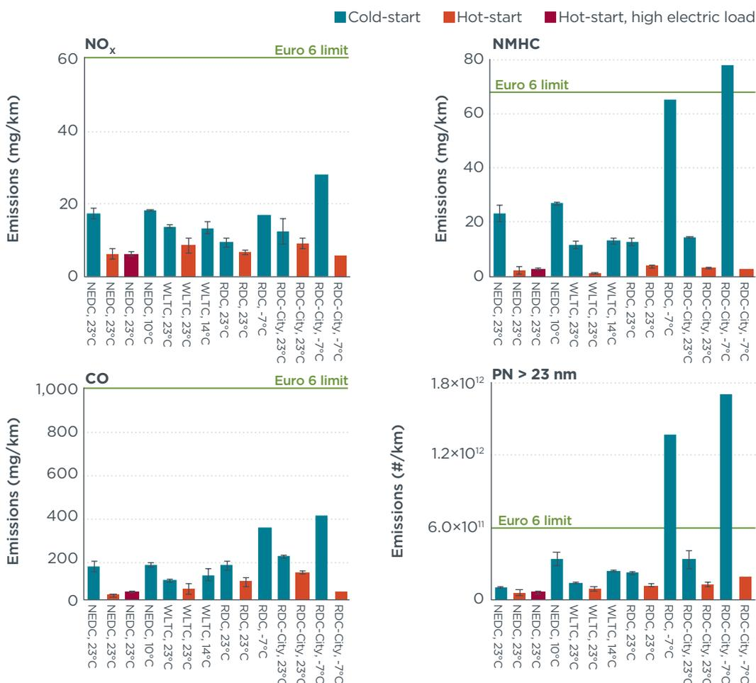
**Figure 4.** Tailpipe emission factors over the tested cycles for the regulated pollutants
