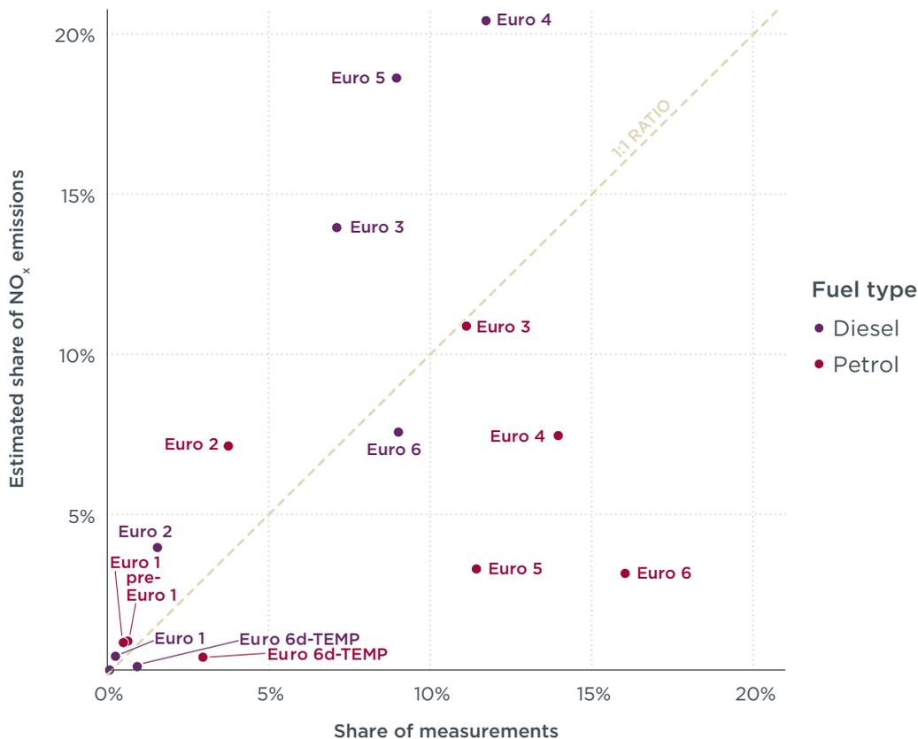
**Figure 8.** Share of measurements and estimated share of total NO<sub>x</sub> emissions in Krakow from passenger cars by emissions standard and fuel type. The share of remote sensing measurements is considered as a crude proxy of vehicle-kilometers travelled by each group of vehicles
