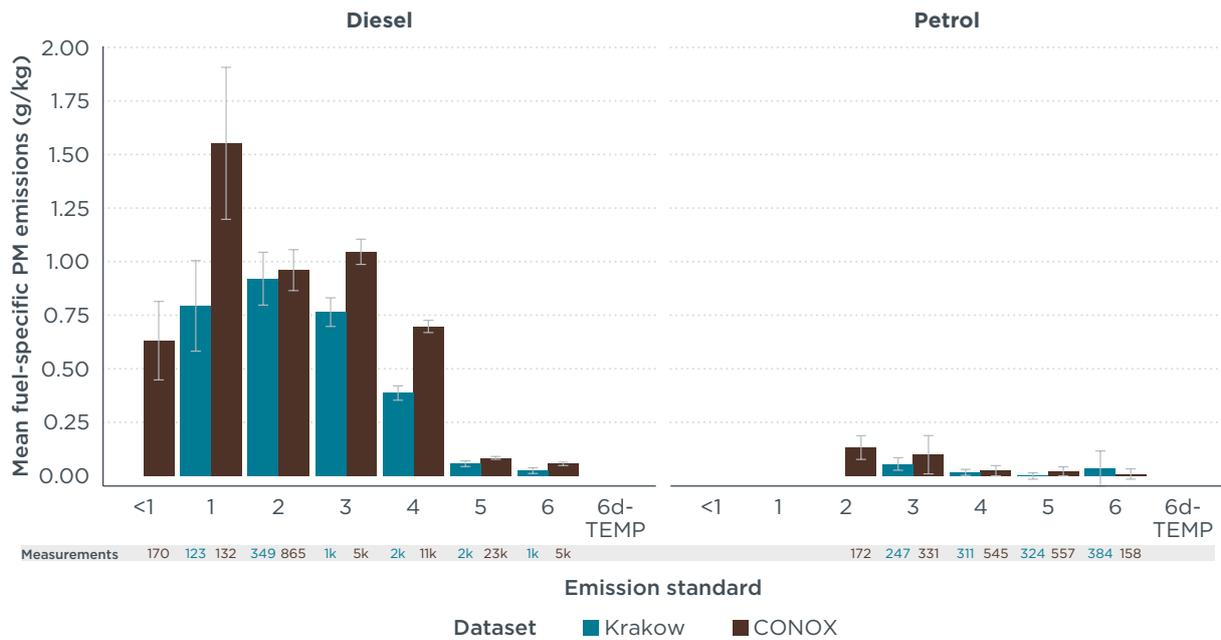
**Figure 13.** Mean fuel-specific PM emissions from diesel and petrol light commercial vehicles, grouped by Euro standard, for Krakow and CONOX remote sensing data. The number of measurements is presented at the bottom of each bar. Whiskers represent the 95% confidence interval of the mean. Results are only shown for groups with at least 100 measurements.
