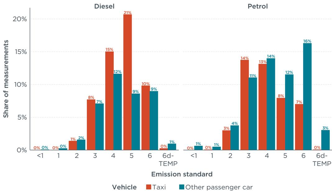
**Figure 15.** Comparison of Krakow taxi and other passenger car measurements in terms of fuel type and emission standard.
