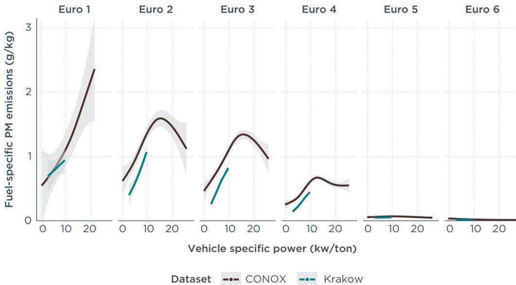
**Figure 14.** Comparison of fuel-specific PM emissions from Euro 1 through Euro 6 diesel passenger cars as a function of VSP in Krakow (blue) and CONOX (brown). The relationship between PM emissions and VSP is represented using generalized additive models with 95% confidence intervals. Round markers represent mean PM emissions and VSP.
