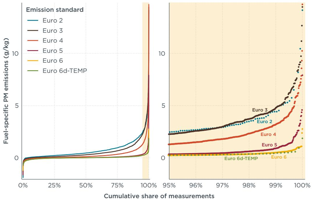
**Figure 19.** Cumulative distribution of diesel passenger car fuel-specific PM emissions by emissions standard. Left panel: Full range. Right panel: 95<sup>th</sup> to 100<sup>th</sup> percentile.
