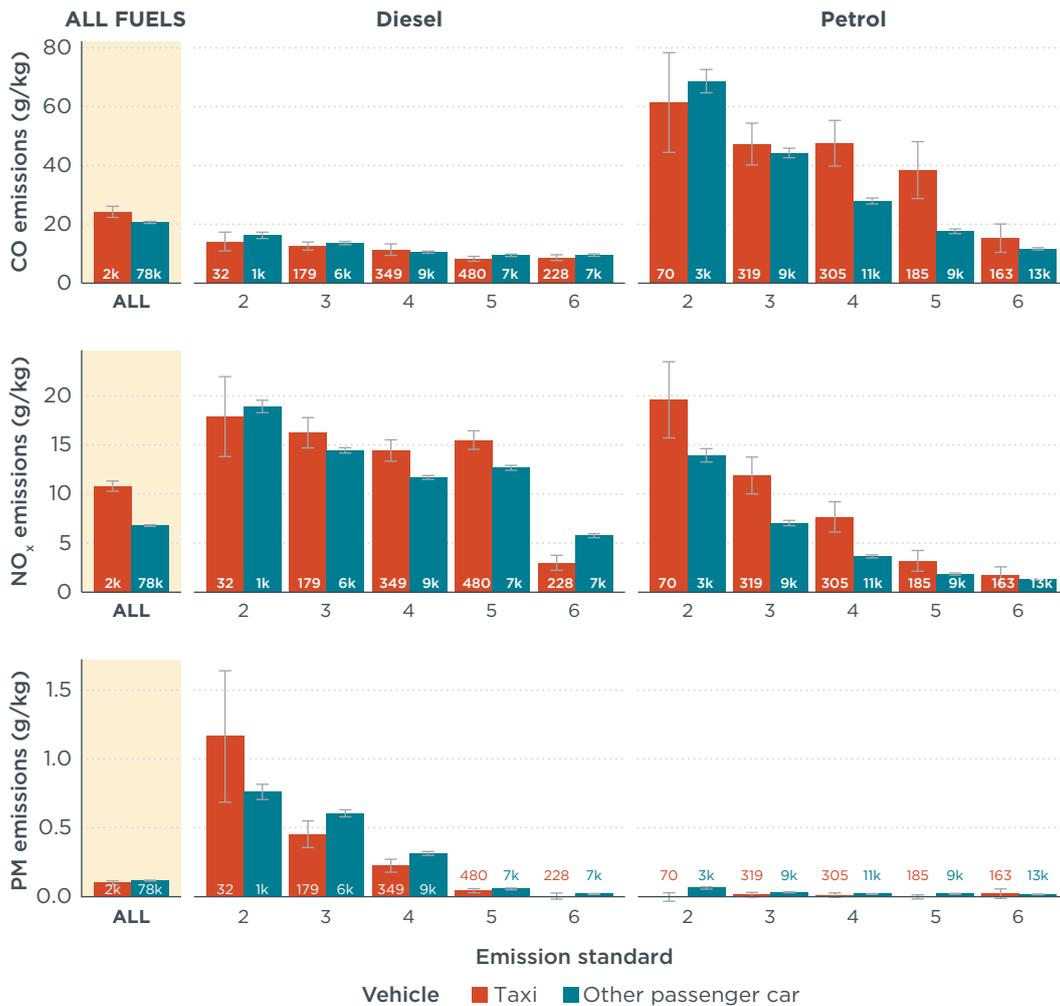
**Figure 16.** Mean fuel-specific CO, NO<sub>x</sub>, and PM emissions from Krakow taxis and other passenger cars in total and by fuel type and emissions standard. The number of measurements is presented at the bottom of each bar. Whiskers represent the 95% confidence interval of the mean.
