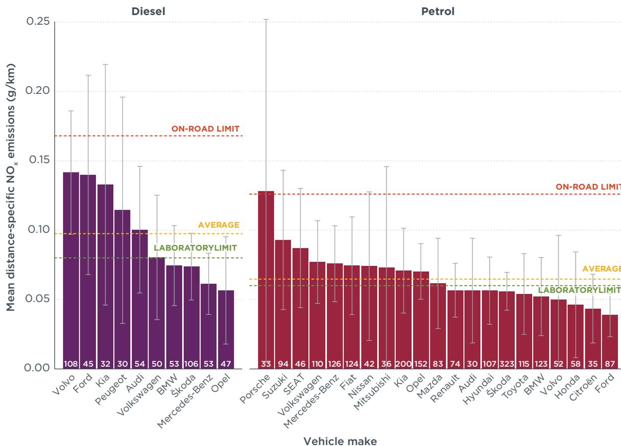
**Figure 7.** Mean distance-specific NO<sub>x</sub> emissions from Euro 6d-TEMP passenger cars, grouped by fuel type and make, for Krakow remote sensing data. The number of measurements is presented at the bottom of each bar. Whiskers represent the 95% confidence interval of the mean. Results are only shown for groups with at least 30 measurements.
