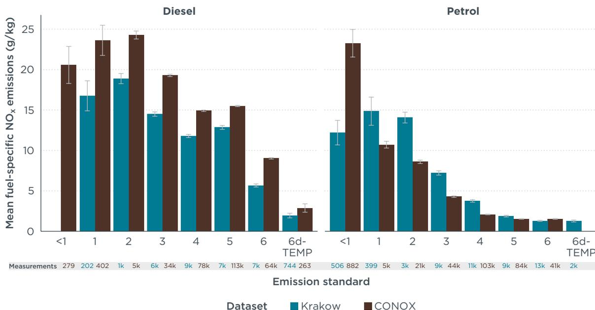
**Figure 4.** Mean fuel-specific NO<sub>x</sub> emissions from diesel and petrol passenger cars, grouped by emission standard, for Krakow and CONOX remote sensing data. The number of measurements is presented below each bar. Whiskers represent the 95% confidence interval of the mean. Results are only shown for groups with at least 100 measurements.
