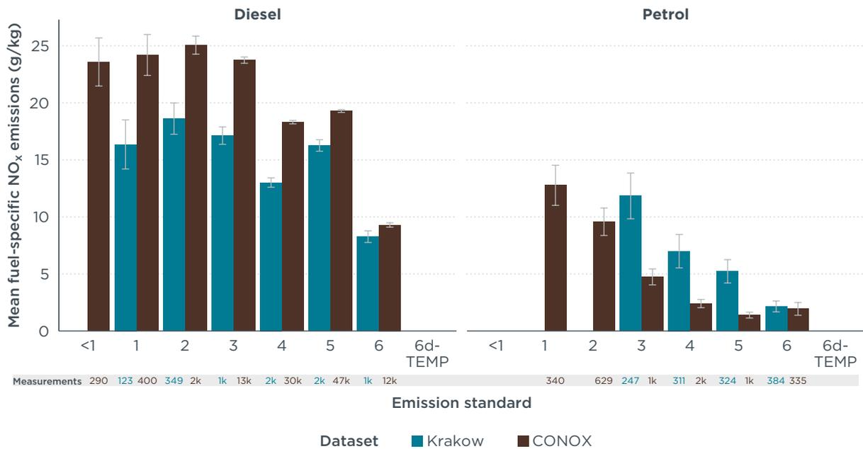
**Figure 9.** Mean fuel-specific NO<sub>x</sub> emissions from diesel and petrol light commercial vehicles, grouped by emissions standard, for Krakow and CONOX remote sensing data. The number of measurements is presented below each bar. Whiskers represent the 95% confidence interval of the mean. Results are only shown for groups with at least 100 measurements.
