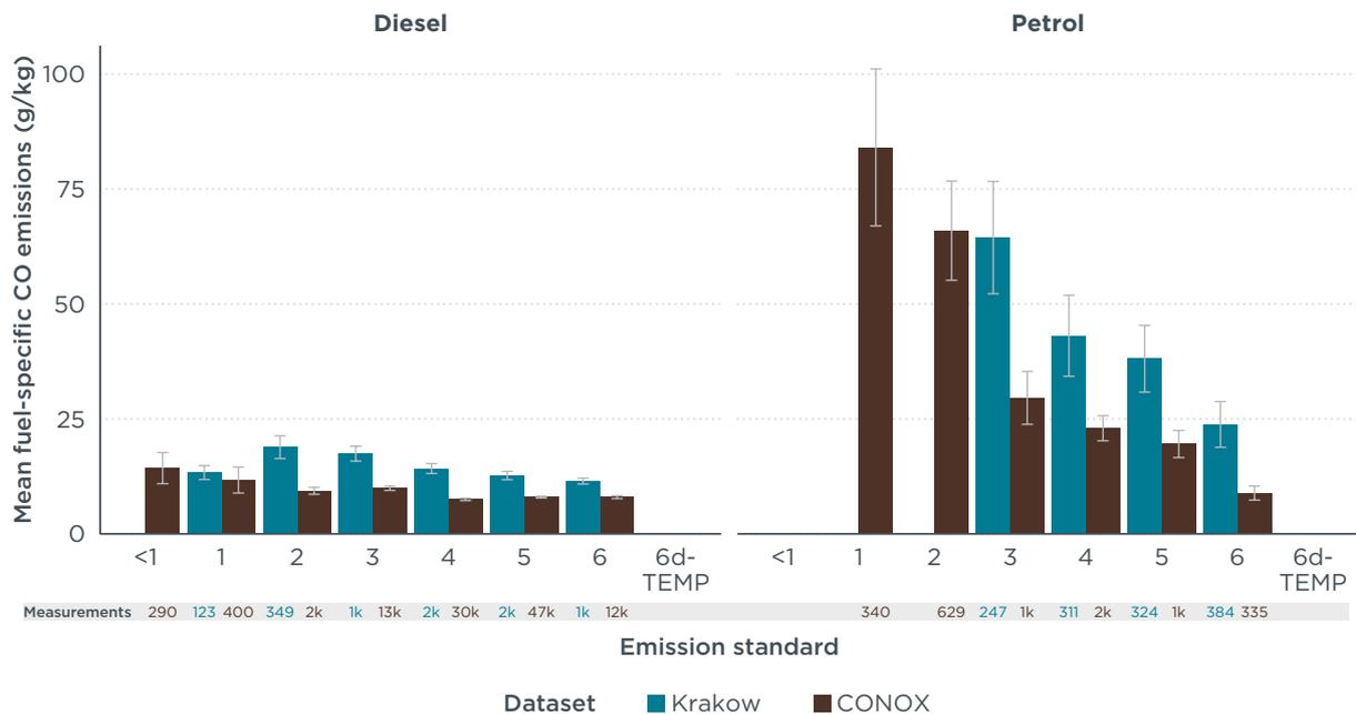
**Figure 11.** Mean fuel-specific CO emissions from diesel and petrol light commercial vehicles, grouped by emissions standard, for Krakow and CONOX remote sensing data. The number of measurements is presented at the bottom of each bar. Whiskers represent the 95% confidence interval of the mean. Results are only shown for groups with at least 100 measurements.
