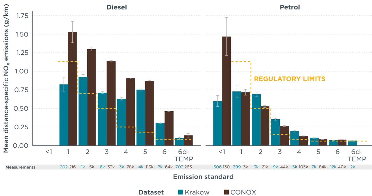
**Figure 6.** Mean estimated distance-specific NO<sub>x</sub> emissions from diesel and petrol passenger cars, grouped by emissions standard, for Krakow and CONOX remote sensing data. The number of measurements is presented below each bar. Whiskers represent the 95% confidence interval of the mean. Results are only shown for groups with at least 100 measurements.
