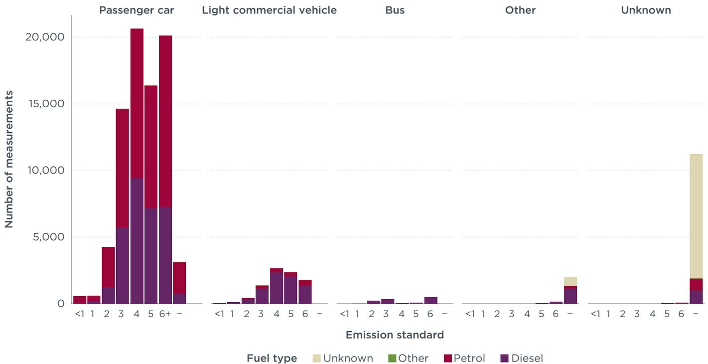
**Figure 3.** Number of remote sensing measurements by vehicle category, estimated emissions standard, and fuel type. Euro <1 refers to vehicle predating Euro standards; 6+ refers to the Euro 6 and 6d-TEMP emission standard; dashes (-) represent unknown values.
