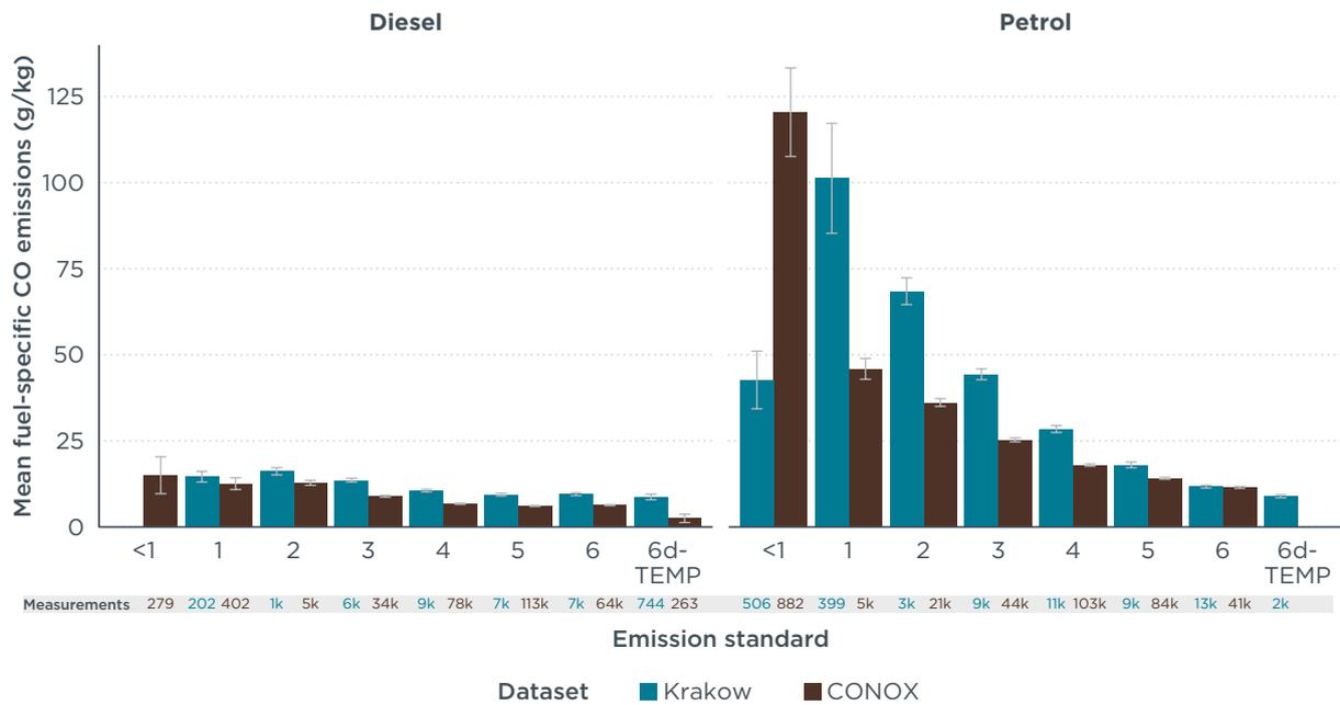
**Figure 10.** Mean fuel-specific CO emissions from diesel and petrol passenger cars, grouped by emissions standard, for Krakow and CONOX remote sensing data. The number of measurements is presented at the bottom of each bar. Whiskers represent the 95% confidence interval of the mean. Results are only shown for groups with at least 100 measurements.
