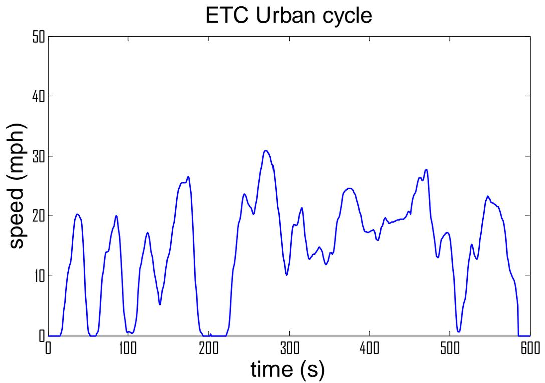
Figure 46. European Test Cycle Urban cycle.
