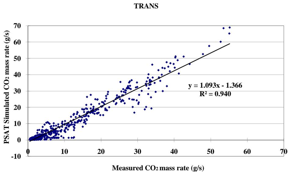
Figure 31. CO<sub>2</sub> mass rate prediction results for Transient cycle. Predicted mass rate: 9.30 g/s; Measured mass rate: 9.76 g/s; Prediction error 4.68%. Coefficient of rolling resistance 0.0136.
