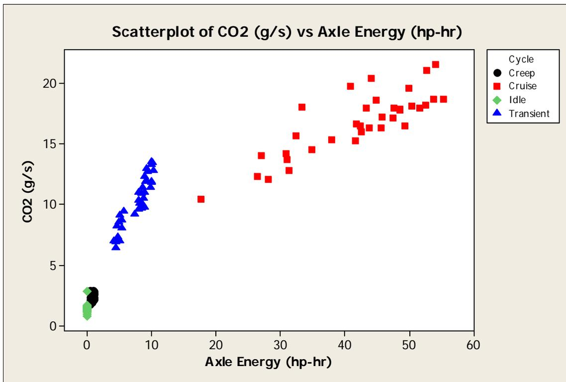
Figure 34. Variation of  $CO_2$  emissions with axle power (test weight) for the Creep, Transient, and Cruise cycles.
