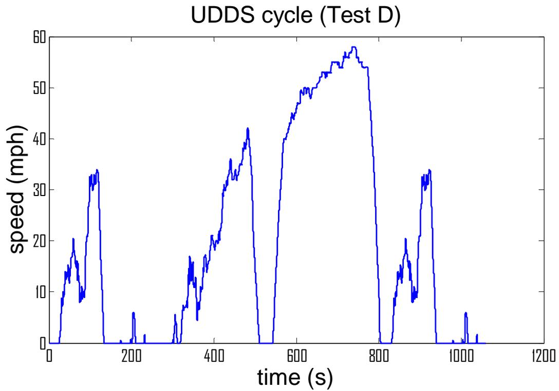
Figure 48. Urban Dynamometer Driving Schedule (Test\_D cycle).
