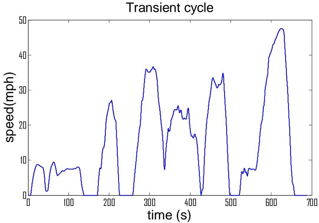
Figure 47. CARB Transient cycle.
