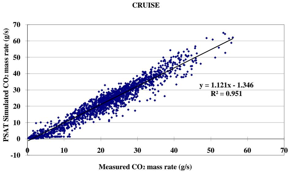
Figure 32. CO<sub>2</sub> mass rate prediction results for Cruise cycle. Predicted mass rate: 19.00g/s; Measured mass rate: 18.14g/s; Prediction error 4.69%. Aerodynamic drag coefficient 0.37.
