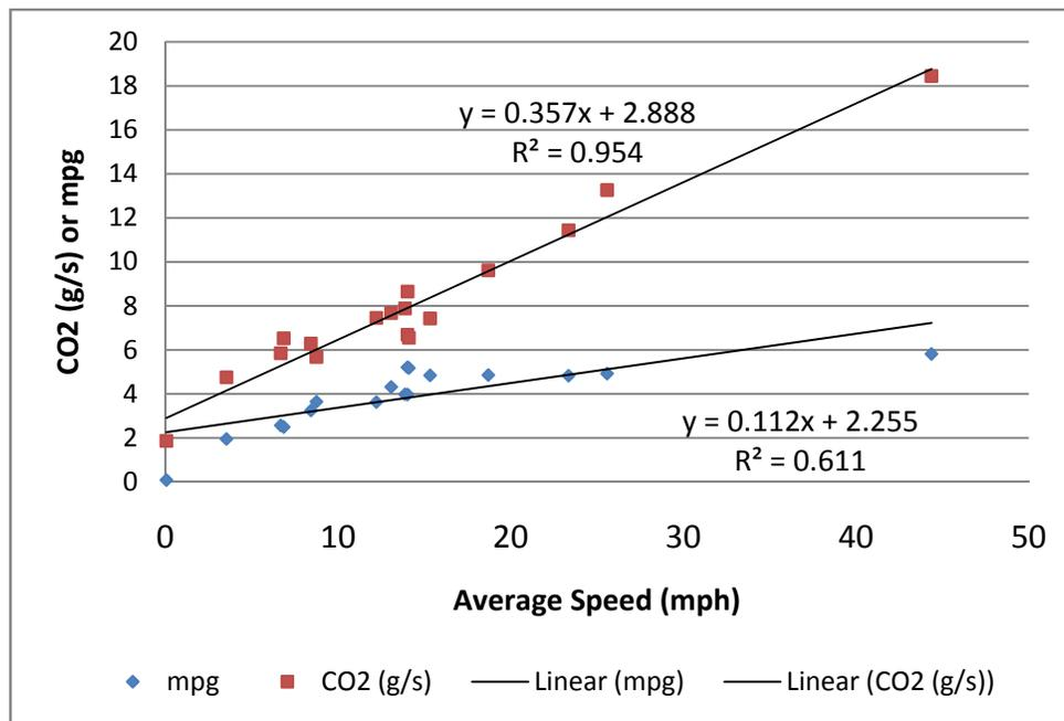
Figure 20. CO<sub>2</sub> mass rate and fuel economy as functions of average speed.
