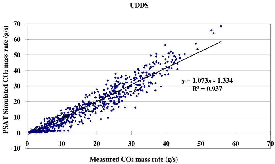
Figure 33. CO<sub>2</sub> mass rate prediction results for UDDS cycle. Predicted mass rate: 11.68 g/s; Measured mass rate: 12.13 g/s; Prediction error 3.69%.
