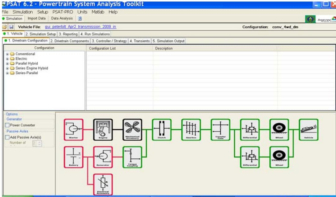
**Figure 30. The PSAT graphical user interface.**
