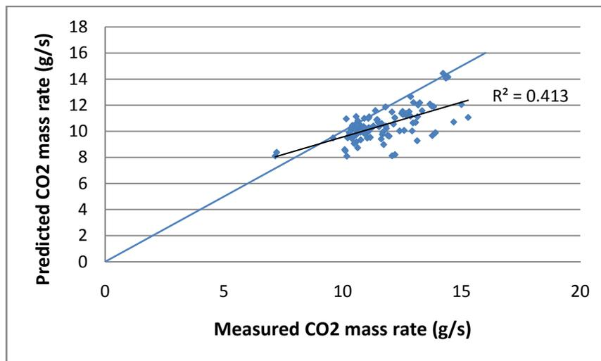
Figure 29. Summary of neural network prediction of CO<sub>2</sub> mass rate (g/s). Prediction error 10.24%.
