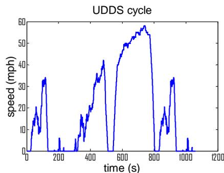
Figure 3. Validation cycle used with truck data set.
