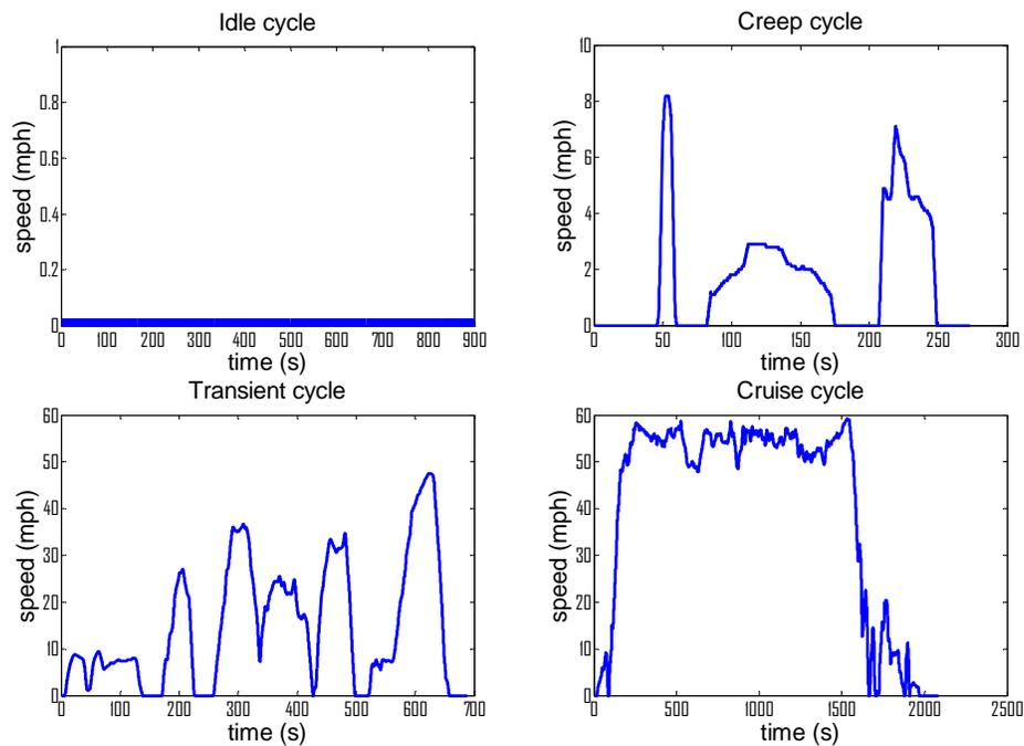
Figure 2. Baseline cycles used with truck data set.
