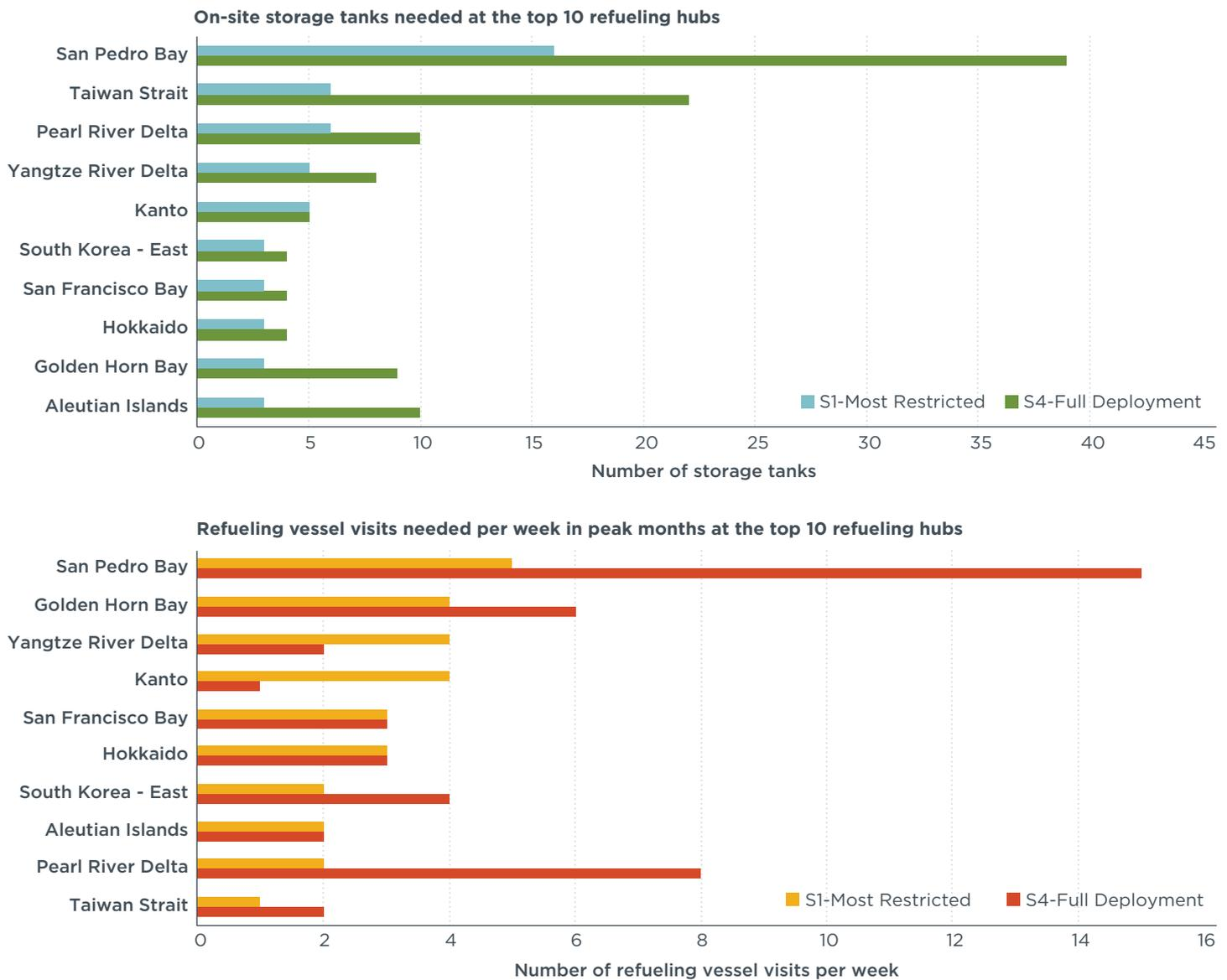
**Figure 7.** Infrastructure need for top 10 refueling hubs
