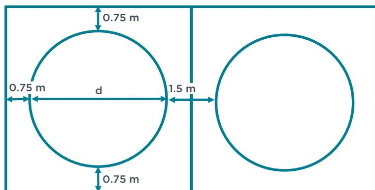
**Figure 3.** Hypothetical arrangement of multiple storage tanks sitting on platforms with safety distance
