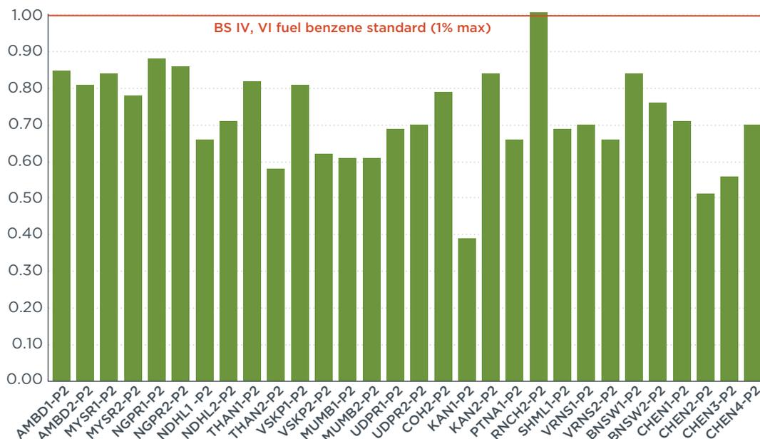
**Figure 7.** Benzene content analyzed in all gasoline samples.
