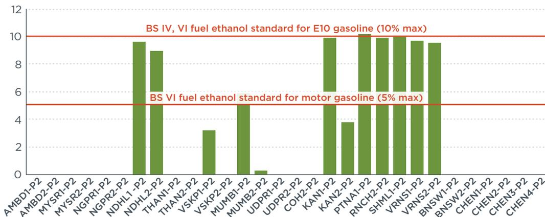
**Figure 8.** Ethanol content analyzed in all ethanol samples.
