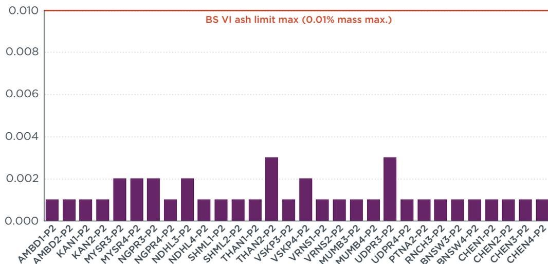
Figure 13. Ash content analyzed in all diesel samples.
