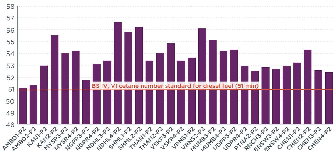
**Figure 11.** Cetane number analyzed in all diesel samples.
