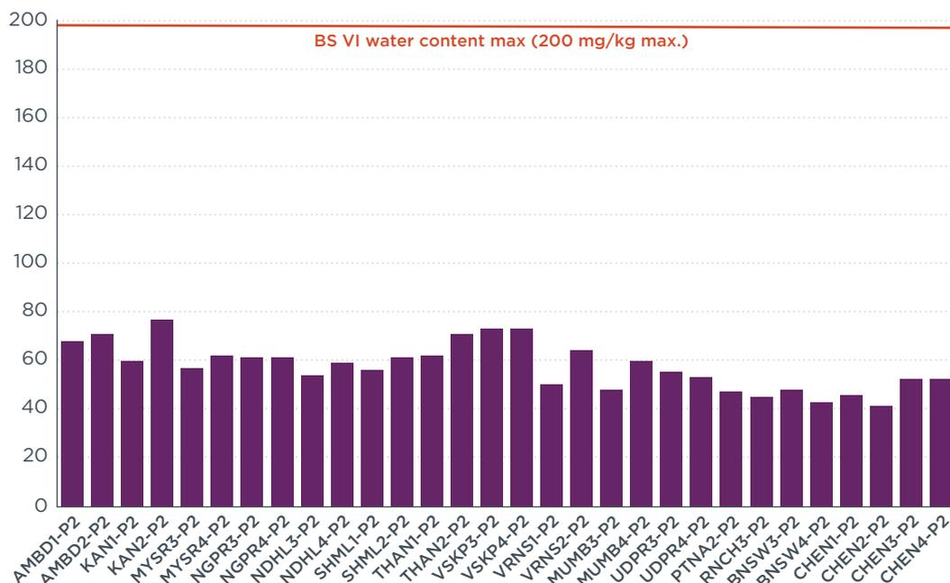
Figure 14. Water content analyzed in all diesel samples.
