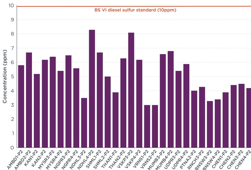
Figure 10. Sulfur content analyzed in all diesel samples.
