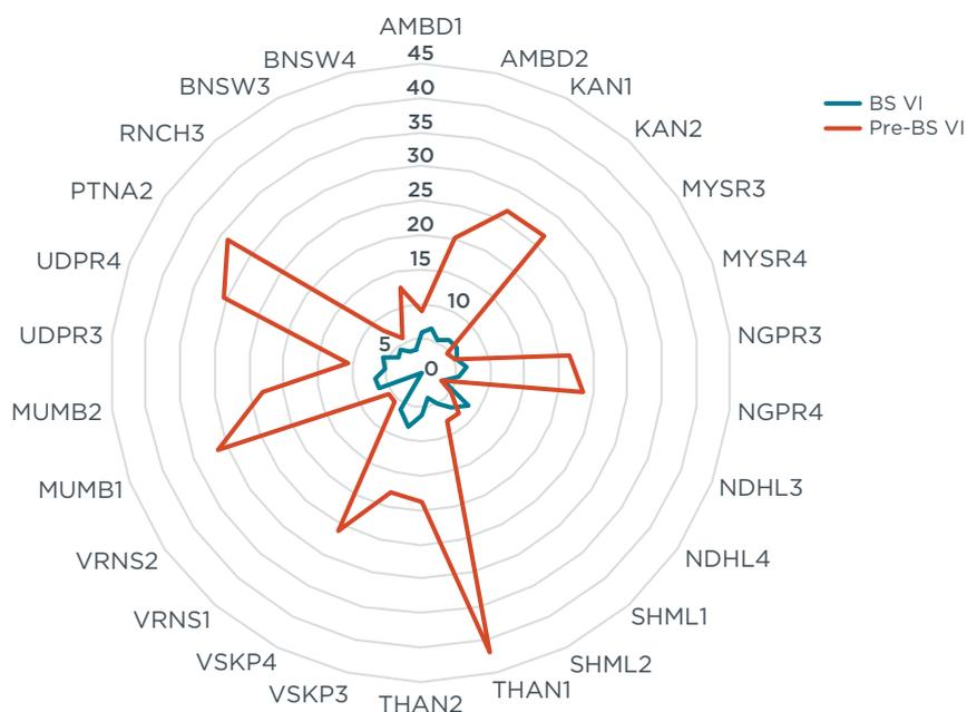
**Figure 26.** Sulfur comparison between pre-BS VI and post-BS VI diesel samples.
