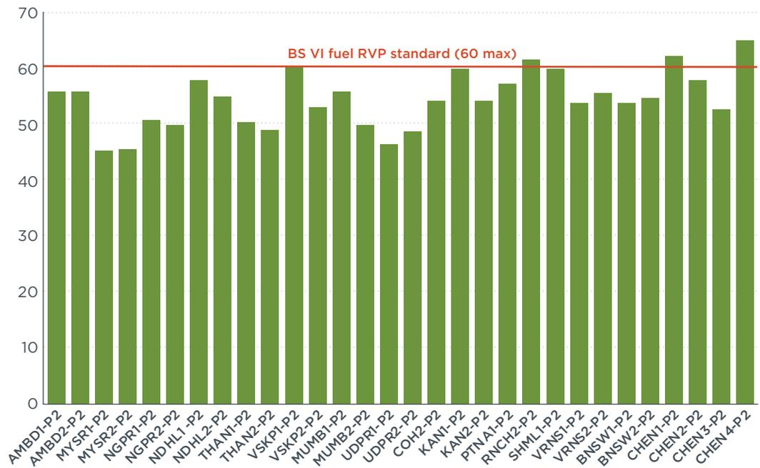
**Figure 2.** RVP analyzed in all gasoline samples.
