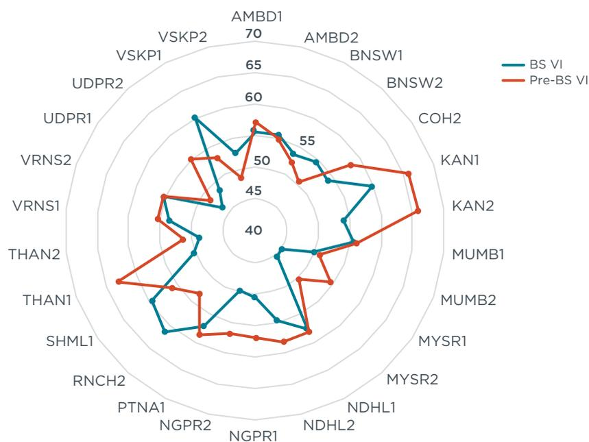
**Figure 17.** RVP comparison between pre-BS VI and post-BS VI samples.
