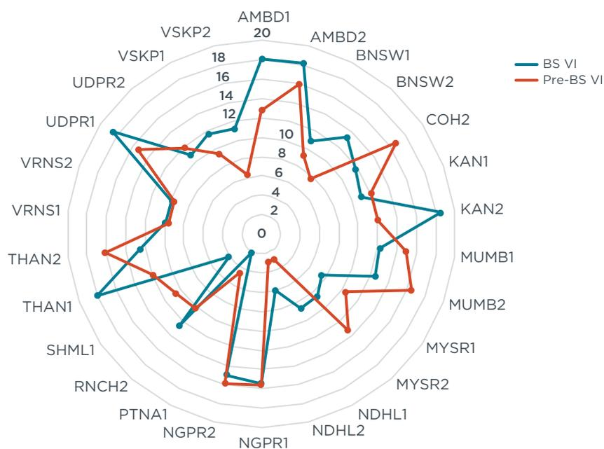
**Figure 19.** Olefins comparison between pre-BS VI and post-BS VI samples.
