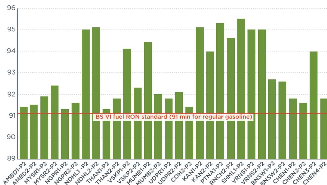
Figure 3. RON analyzed in all gasoline samples.
