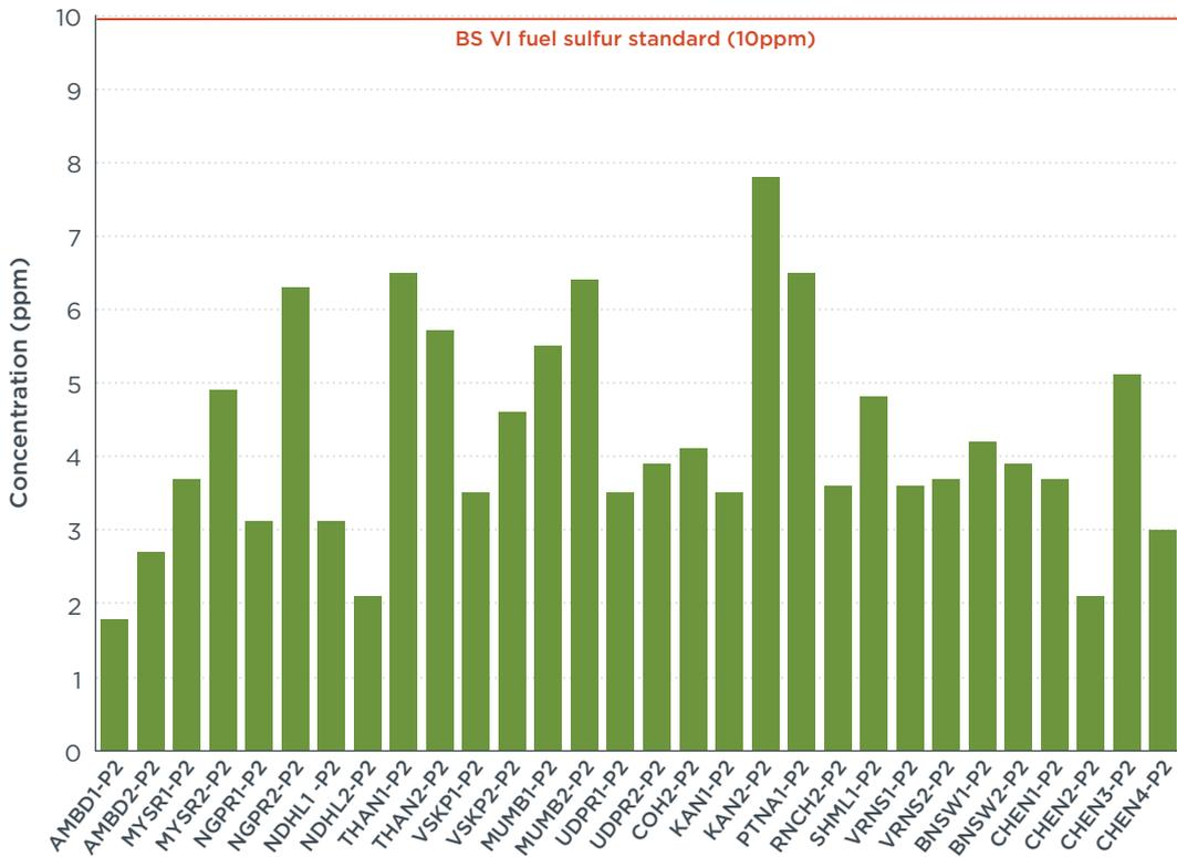
**Figure 1.** Sulfur content of all gasoline samples.
