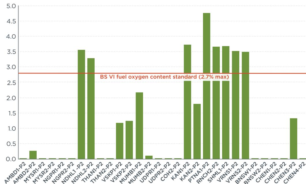
Figure 9. Oxygen content analyzed in all samples.
