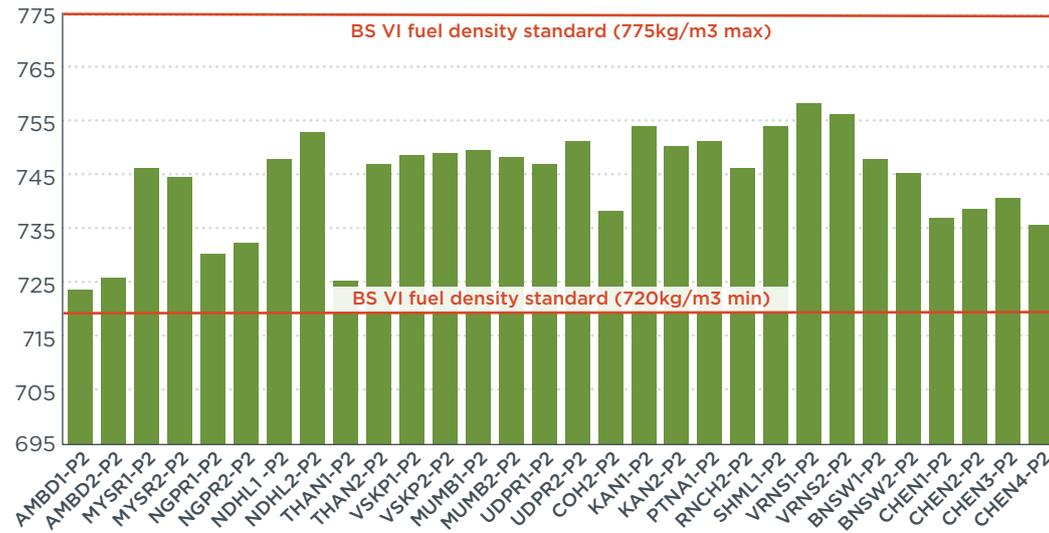
**Figure 5.** Density analyzed in all gasoline samples.
