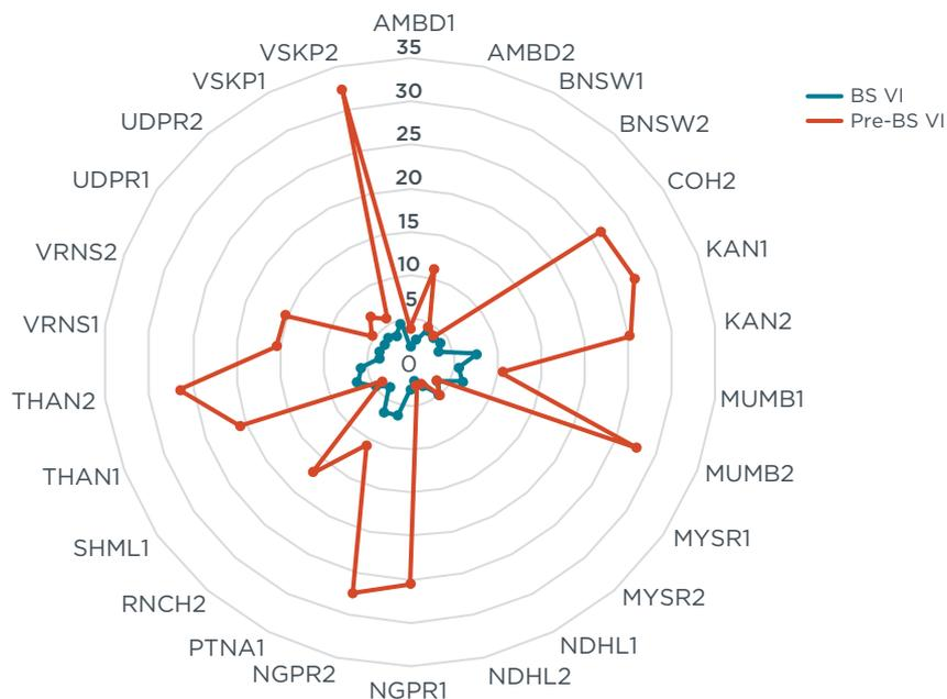
**Figure 21.** Sulfur comparison between pre-BS VI and post-BS VI gasoline samples.
