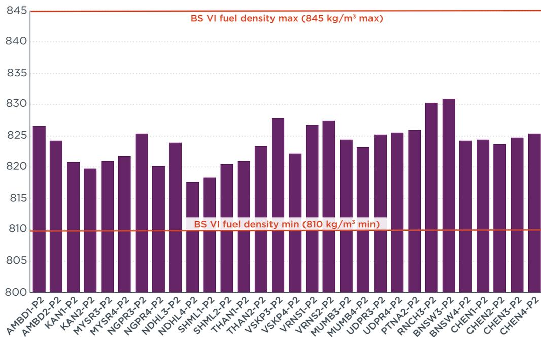
**Figure 12.** Density analyzed in all diesel samples.
