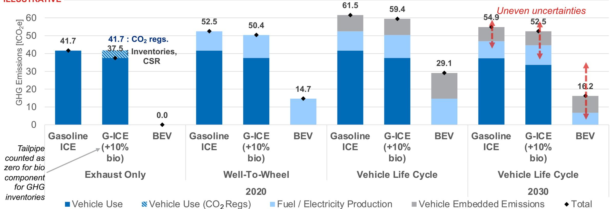
Source: Ricardo Vehicle LCA analysis (June 2020) for average EU lower-medium passenger car. Assumes lifetime 225,000 km, real-world fuel consumption. GHG from fuel/electricity consumption is based on the average fuel/grid electricity factor over the life of the vehicle (Baseline scenario); Calculated 89.0 kgCO<sub>2</sub>e/kWh battery in 2020, 30.0 kgCO<sub>2</sub>e/kWh in 2030. Includes EoL recycling credits
