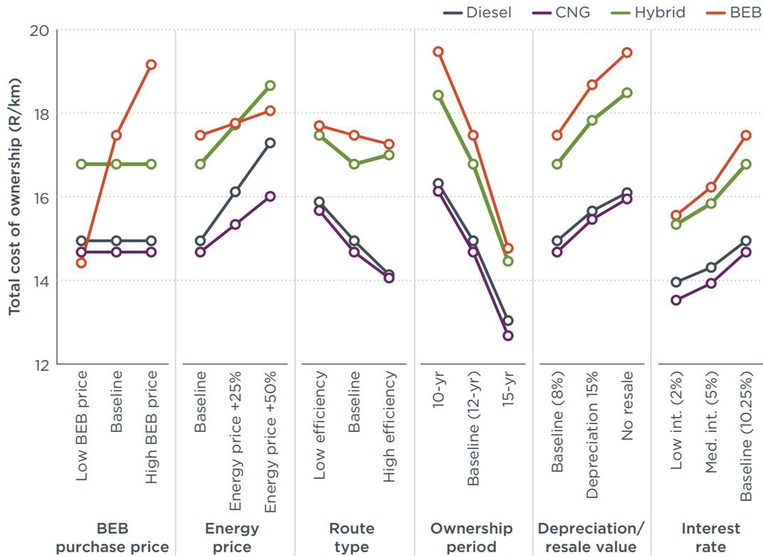
**Figure 15.** Sensitivity analysis for total cost of ownership of a standard (12 m) type bus.
