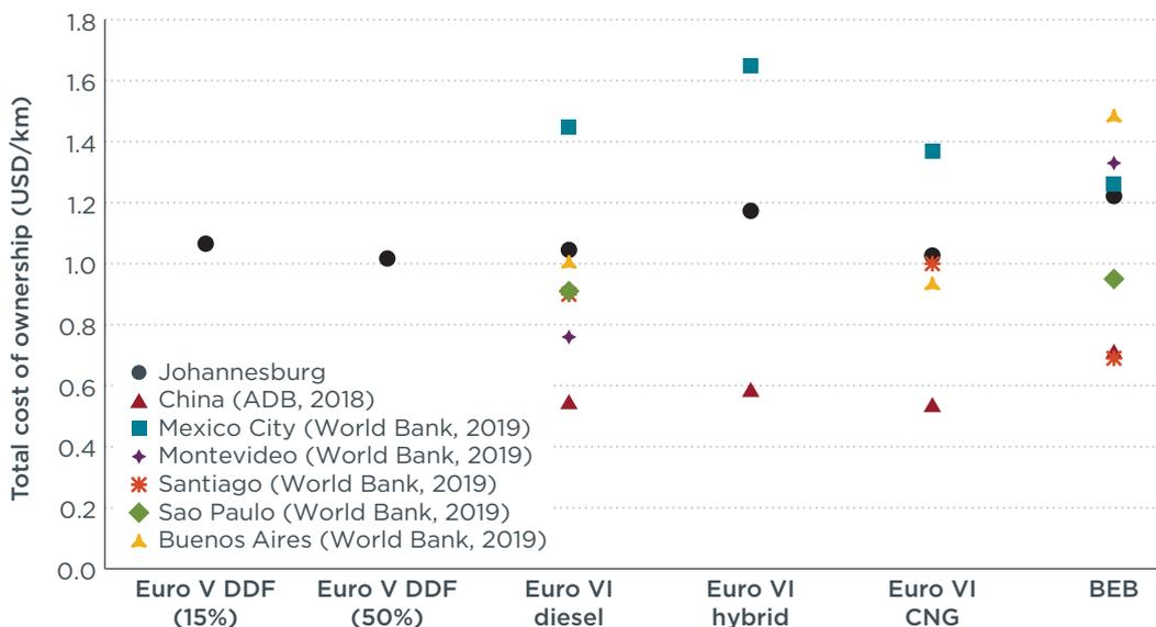
**Figure 14.** International TCO comparison. Note that estimates for China diesel, hybrid, and CNG buses are for pre-Euro VI technologies.
