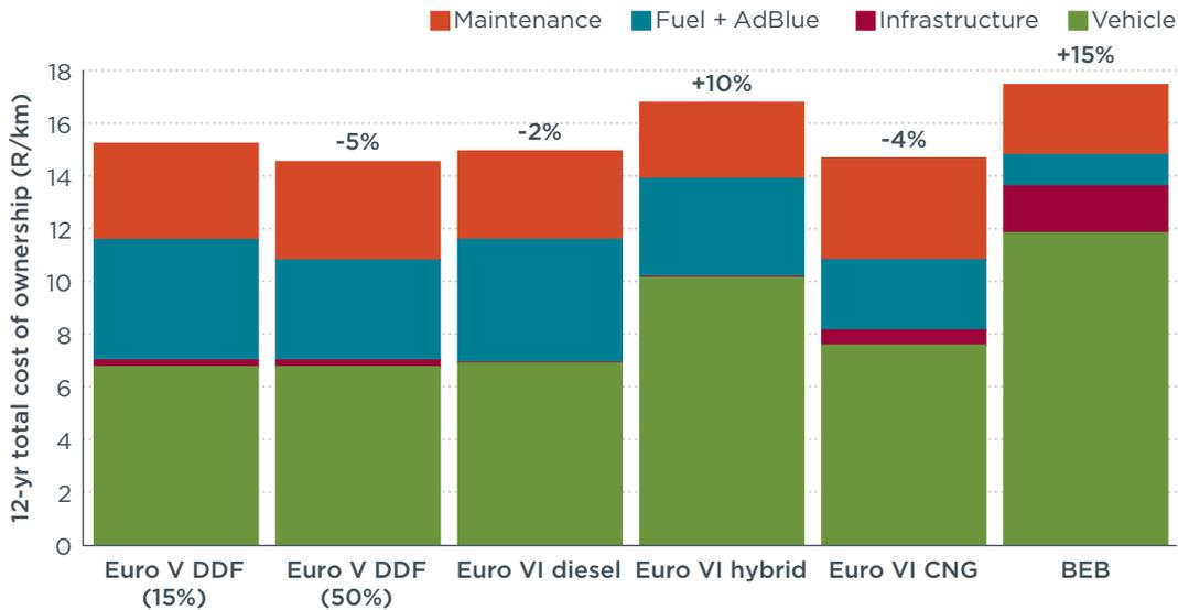
**Figure 13.** Total cost of ownership over 12 years for baseline and alternative technology standard (12 m) type buses in Johannesburg. Percentages show the change in TCO relative to the baseline Euro V DDF technology with a 15% diesel substitution rate. Acquisition costs include down payment and loan payments minus any bus resale value at the end of the ownership term.
