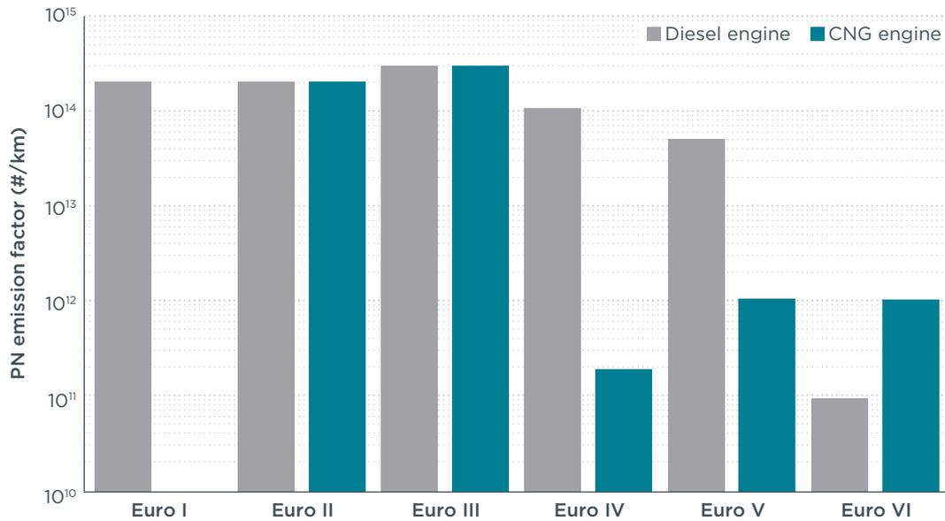
**Figure 9.** Particle number emission factors for standard-sized diesel urban buses by emissions control level and engine technology. Data sourced from HBEFA (2019).
