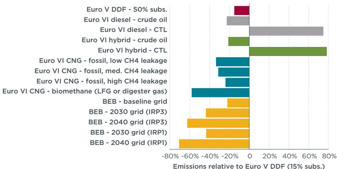
**Figure 5.** WTW GHG emissions relative to the Euro V DDF baseline for buses operating in commuter/suburban driving conditions. Battery electric buses are abbreviated as BEB.
