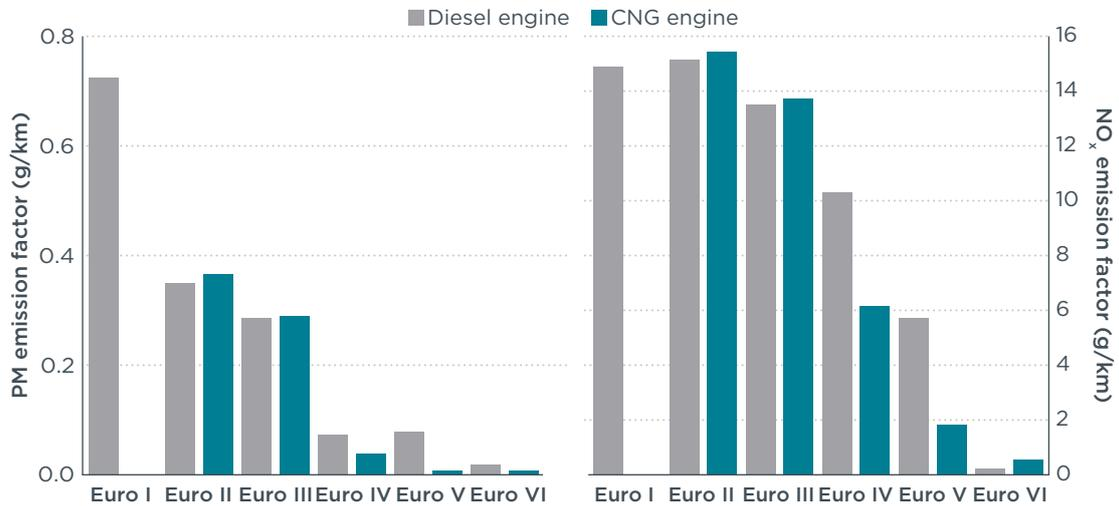
**Figure 8.** PM and  $\text{NO}_x$  emission factors for standard-sized diesel urban buses by emissions control level and engine technology. Data sourced from HBEFA (2019).
