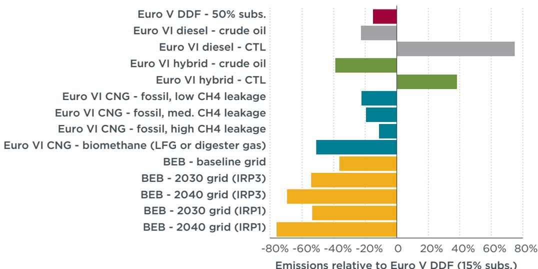
**Figure 7.** WTW GHG emissions relative to Euro V DDF baseline for buses operating in low-speed urban driving conditions.
