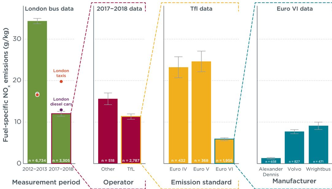
**Figure 11.** Average emission factors for London buses measured using remote sensing technology. Emission factors are presented on a fuel-specific basis with units of grams  $\text{NO}_x$  emitted per kilogram of fuel burned (Dallmann et al., 2018).
