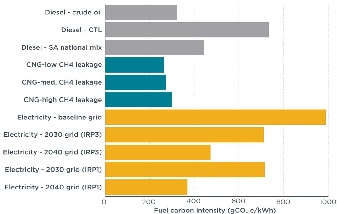
**Figure 3.** Fuel life cycle carbon intensities for fossil diesel, fossil CNG, and electricity.
