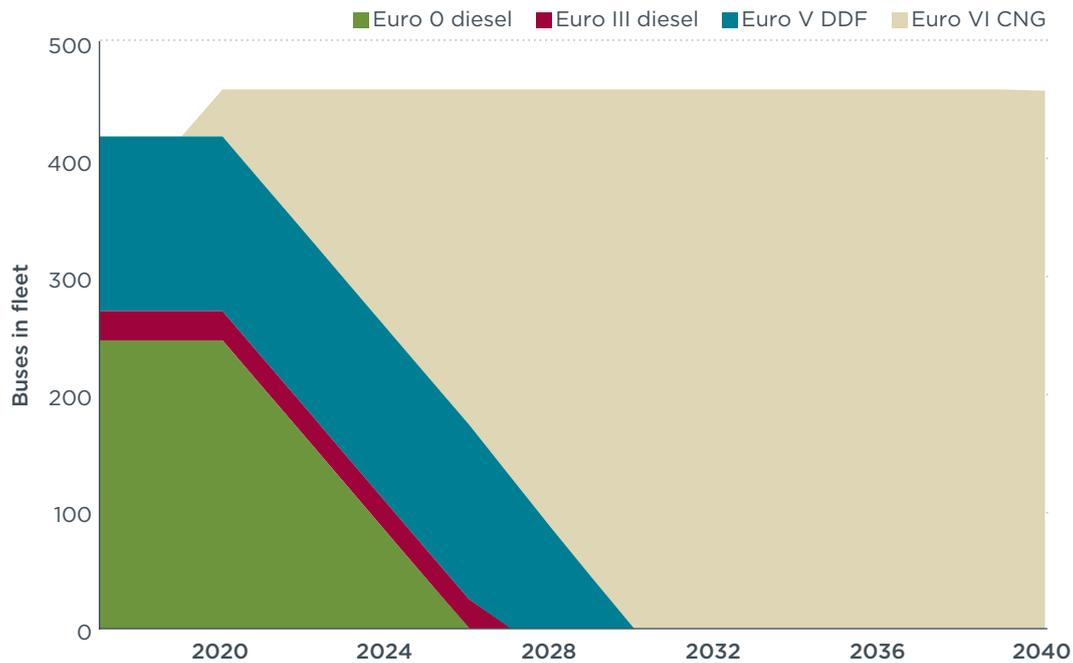
**Figure 21.** Fleet technology evolution under Euro VI CNG procurement pathway.
