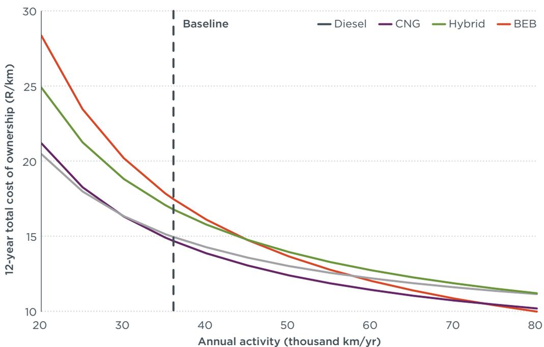
**Figure 16.** Sensitivity of TCO for a standard type bus to annual activity
