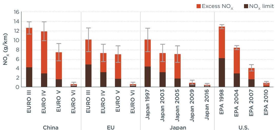
**Figure 10.** Real-world  $\text{NO}_x$  emission factors for buses by vehicle emissions standard (Anenberg et al., 2017).
