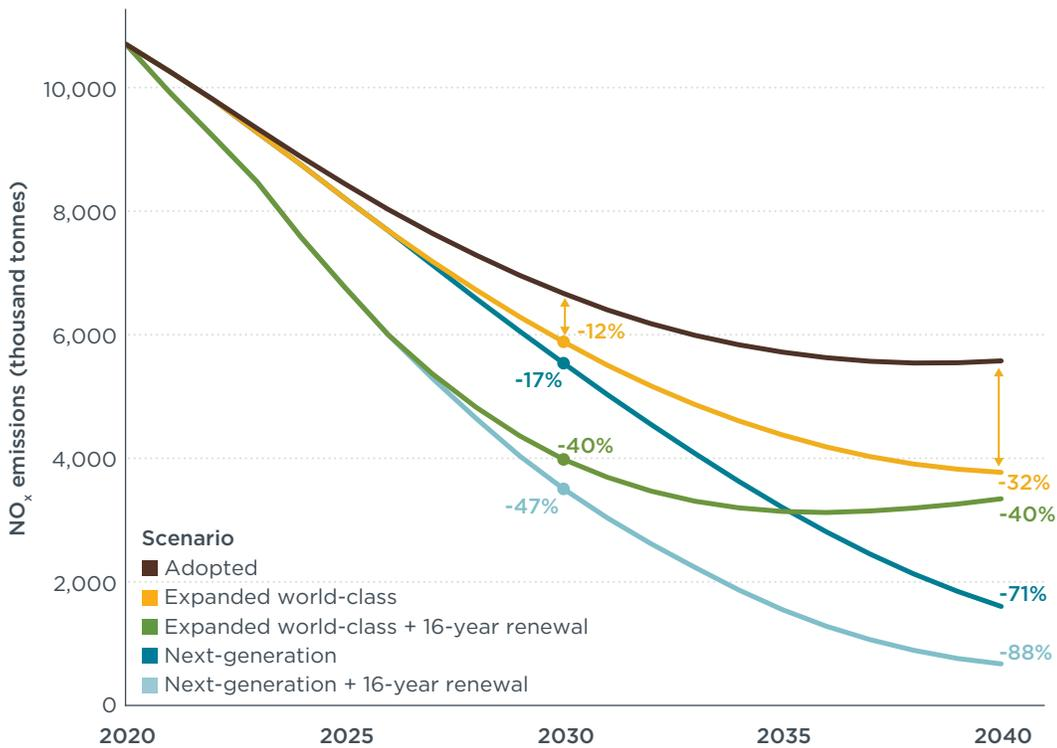
**Figure 5.** Diesel HDV exhaust NO<sub>x</sub> emissions from 2020 to 2040 in G20 economies. Data labels show the percent change in NO<sub>x</sub> emissions compared with adopted policies in 2030 and 2040.
