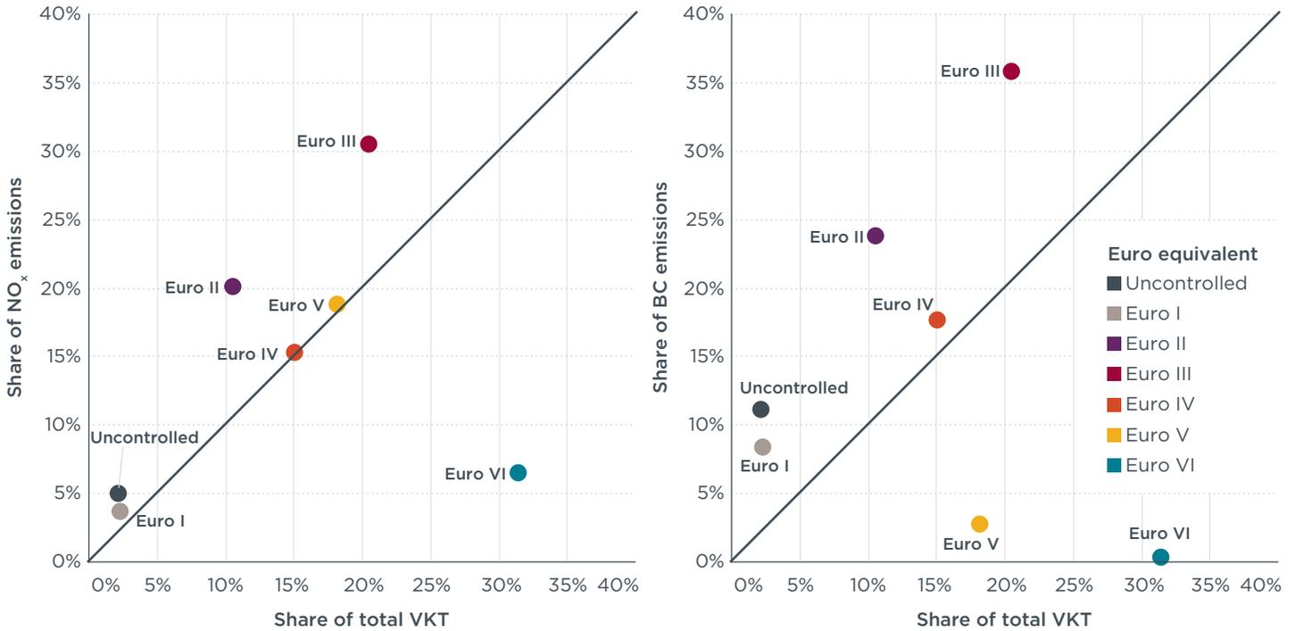
**Figure 4.** Share of total VKT (x-axis) and pollutant emissions (y-axis) by Euro-equivalent emissions standard, 2020. Points above the diagonal line indicate that vehicles of this standard have an outsized impact on emissions relative to their vehicle activity.
