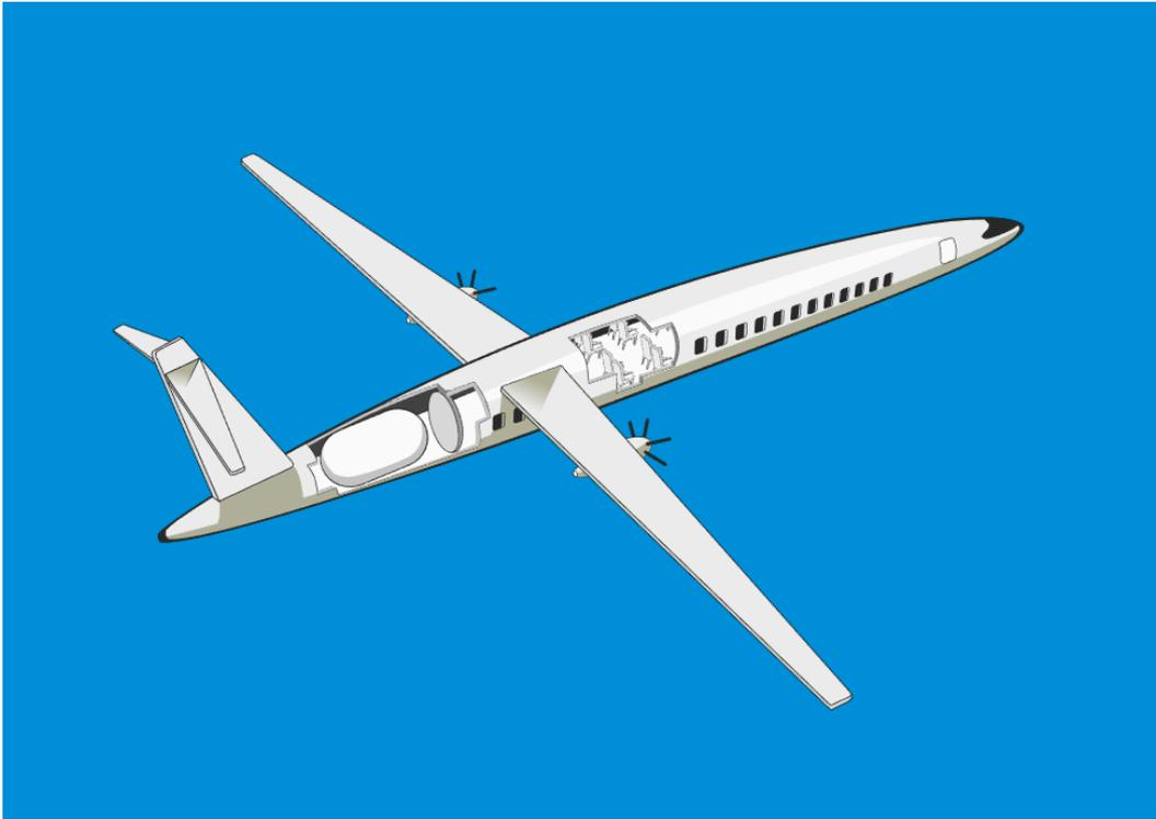
**Figure 3.** Representation of the tank and passenger cabin layout for the LH<sub>2</sub>-powered turboprop
