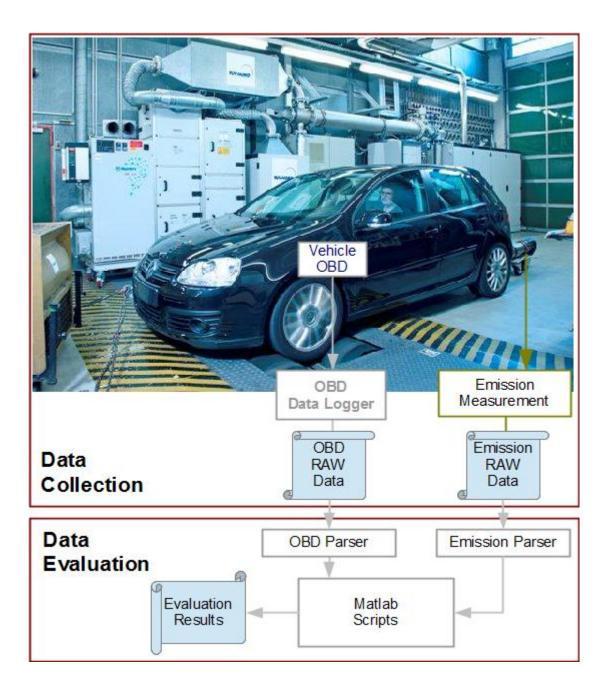
The measurement equipment delivers a record-file containing masses of the vehicle emission pollutants (HC,  $HC_{Diesel}$ ,  $CH_4$ , NOX, NO, CO,  $CO_2$ ) given in milligram per second as well as the corresponding vehicle speed in kilometers per hour and the power given in Newton. Based on these measurement values the vehicle fuel consumption was calculated according to the equations given in [ECE\_R101]:
