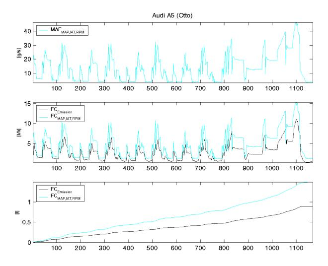
The experiment to improve the  $FC_{MAP,IAT,RPM}$  results with consideration of the long term and short term fuel trim values are visualized in the following diagrams. SFT and LFT modify the air-to-fuel ratio over time, which is set to the constant value of 14.7:1. The plots of the FC<sub>OBD</sub> values with different combinations of SFT and LFT show only marginal improvements compared to the deviation to the FC<sub>Dyno</sub> curve.
