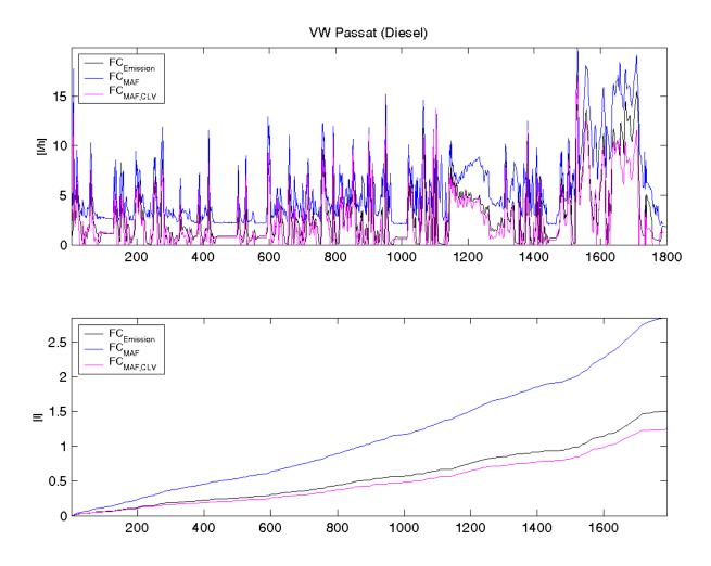
The following diagrams show the emission based calculation of the fuel consumption  $FC_{Dyno}$  against the calculated load value and the manifold air pressure values provided by the vehicle OBD system. Subsequently to the initial experiments of this study, the investigation of further methods for estimating the vehicle fuel consumption based on the CLV could show if the accuracy could be improved, in particular if the vehicle does not support the MAF sensor data.
