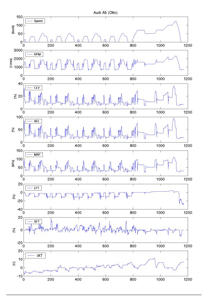
The following plot shows the vehicle speed measured by the OBD interface and the dynamometer test stand. The synchronization of data in time shows that both data flows are relatively close together. The subtraction of the OBD speed from the Dyno speed shows that the OBD speed is a bit below the Dyno speed in positive acceleration phases and a bit higher at constant speed and during negative acceleration phases.
