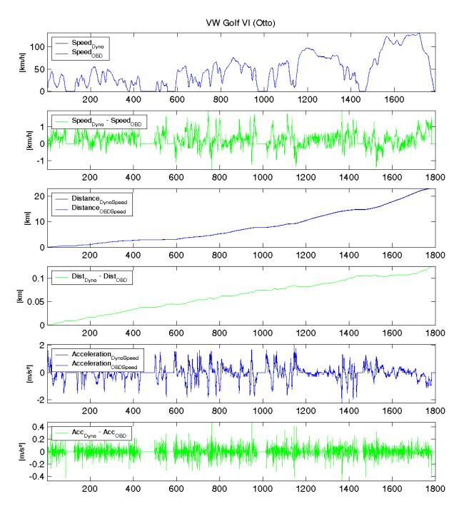
Similar to the AUDI A5, the tested VW Golf does not provide MAF sensor data via the OBD interface. Therefore, the fuel consumption was calculated with an estimation of the air flow rate based on the MAP sensor data. The plots show parallels of the OBD and Dyno data but also a large offset between both curves.
