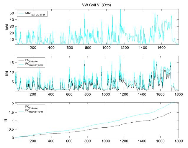
If the long term fuel trim data and short term fuel trim data are applied to the FC calculation, the results are similar to the results from the experiment with the AUDI vehicle. Applying the fuel trim data show no considerable improvement in view of the deviation to  $FC_{Dyno}$ , although the fuel trim values show different characteristics over the driving cycle.
