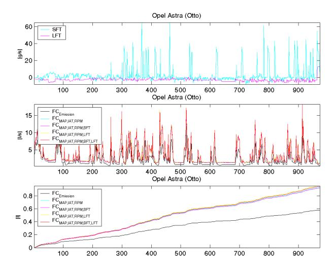
Contrary to the two other Otto engine vehicles that were tested, the Opel Astra provides the MAF sensor data via the OBD interface.
