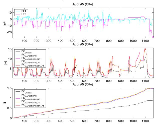
The following diagrams show the emission based calculation of the fuel consumption  $FC_{Dyno}$  against the calculated load value and the manifold air pressure values provided by the vehicle OBD system. Subsequently to the initial experiments of this study, the investigation of further methods for estimating the vehicle fuel consumption based on the CLV could show if the accuracy could be improved, in particular if the vehicle does not support the MAF sensor data.
