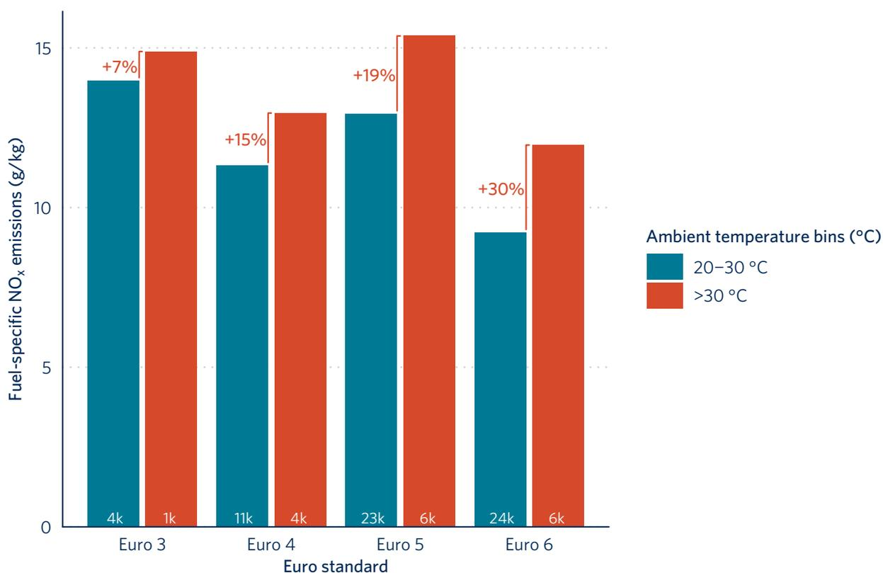
Average NO<sub>x</sub> emissions from diesel cars, in grams per kilo of fuel consumed. In hot weather, NO<sub>x</sub> emissions from Euro 6 cars were worse than emissions from Euro 4 cars at milder temperatures. The gap between in-use NO<sub>x</sub> emissions measured at ambient temperatures between 20 and 30 °C, which is the type-approval test range, and above 30 °C increases with every Euro standard, as type-approval NO<sub>x</sub> limits become more stringent.
