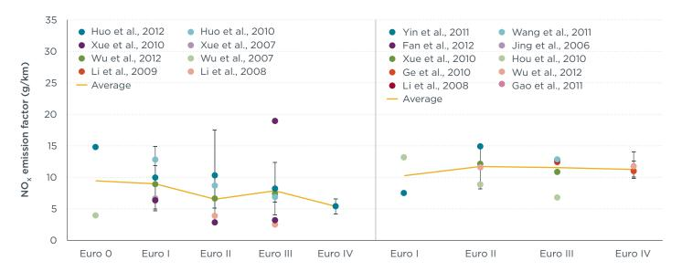
Summary of Chinese PEMS testing results for NO, emissions from heavy-duty diesel trucks (left) and buses (right). Note lack of significant reductions in average NO<sub>x</sub> emission factors, especially from Euro 0 to Euro III, even as emission standards have become more stringent.
