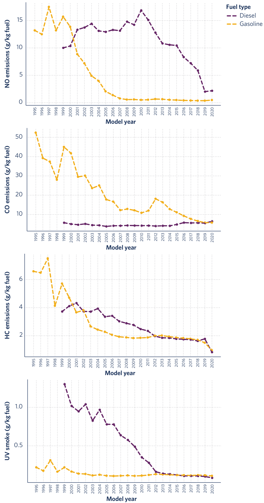
Figure 11. Average NO, CO, HC, and UV smoke from light-duty passenger vehicles, by fuel type and model year.
