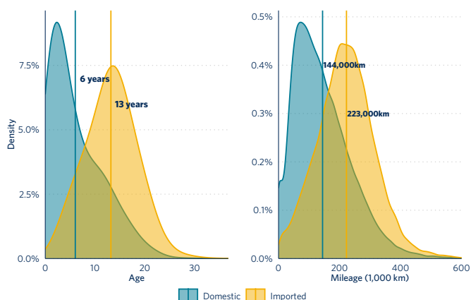
Distribution of ages and mileages (left panel) and average fuel-specific NO x , PM, CO, and HC emissions (right panel) of domestic and imported vehicles measured in Warsaw in 2020. Vertical lines (left panel) indicate the average ages and mileages of the two vehicle groups.
