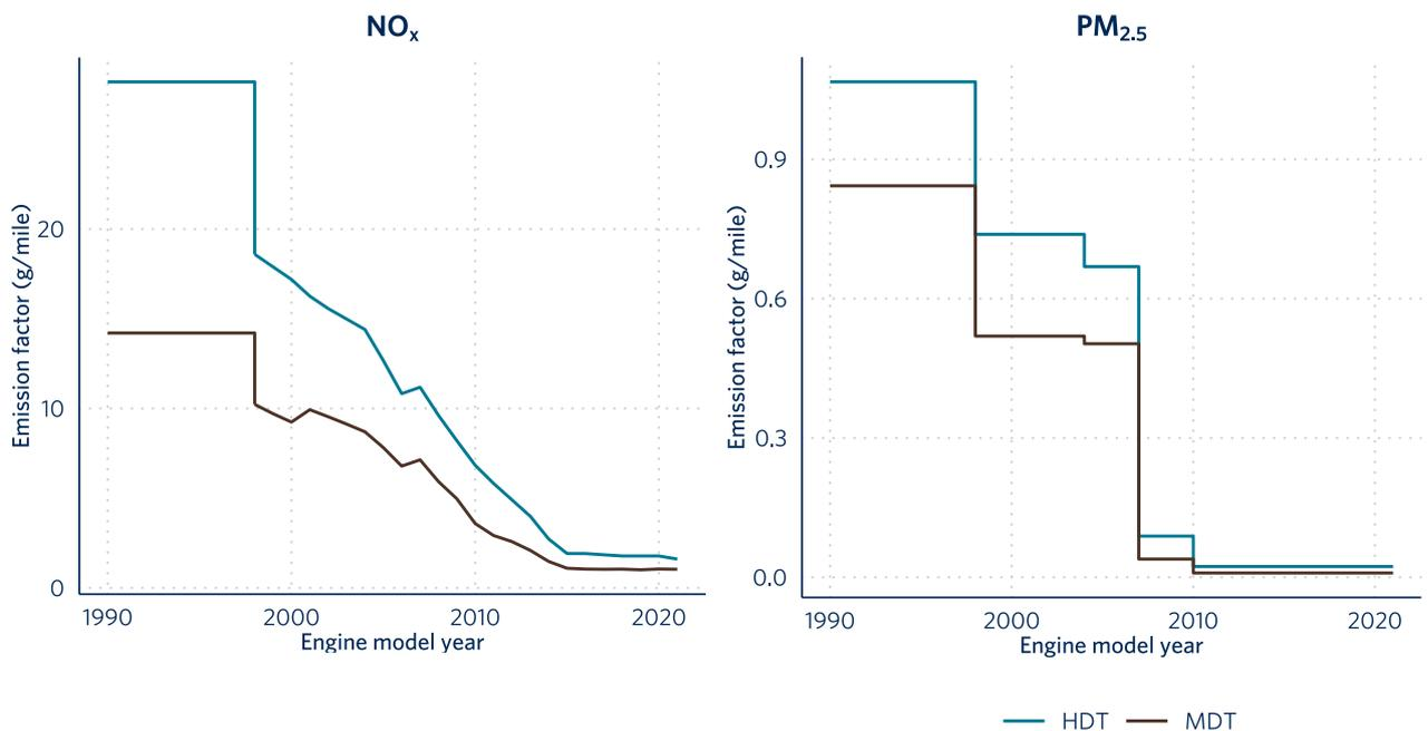
**Figure A2.** NO<sub>x</sub> and PM<sub>2.5</sub> emission factors by engine model year.
