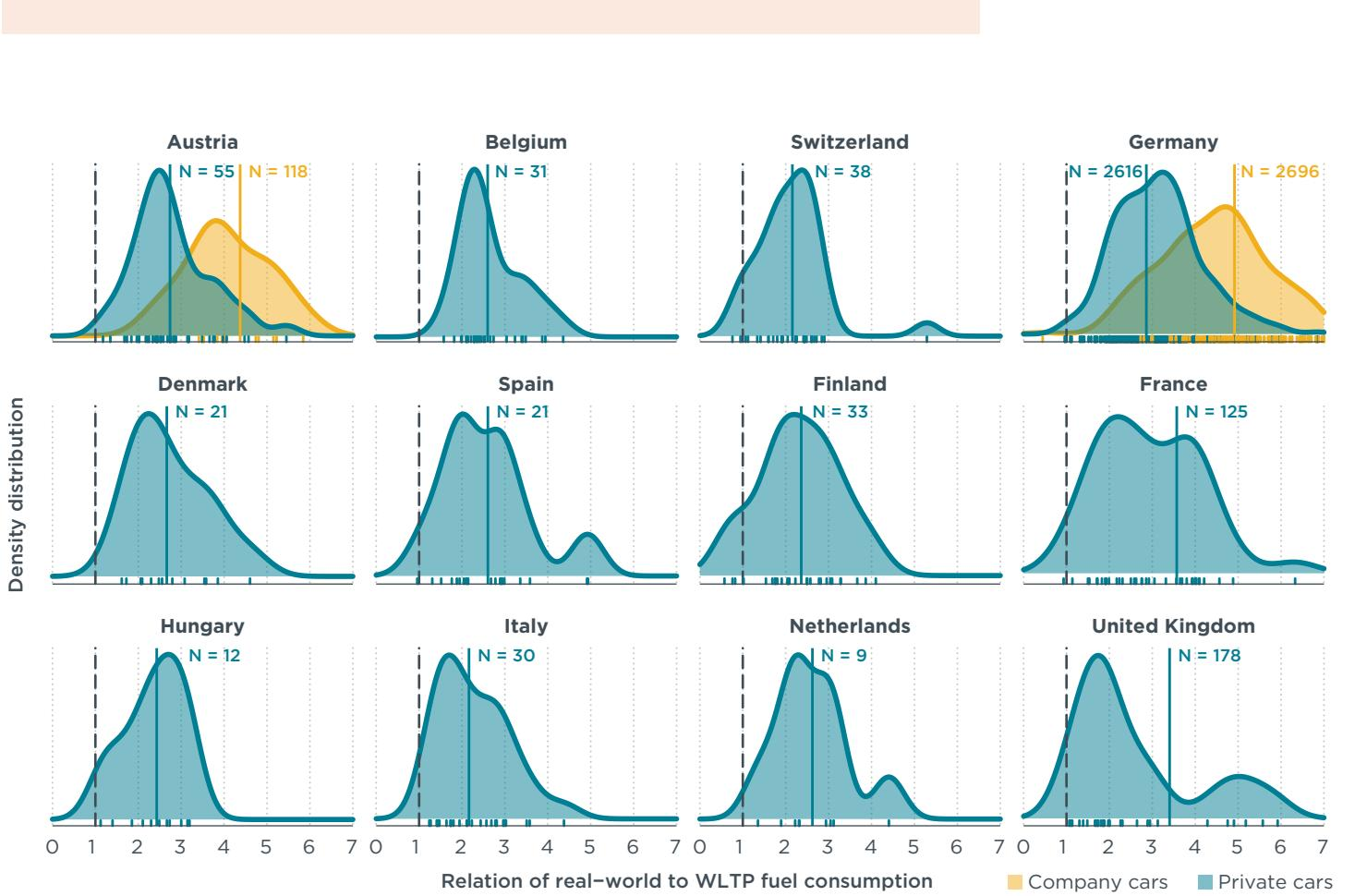
**Figure ES2.** Distribution of real-world fuel consumption values in relation to WLTP type-approval fuel consumption values for PHEVs across Europe. 'N' indicates the number of vehicles included in the respective sample. Solid vertical bars indicate country specific (sample size-weighted) mean, dashed vertical lines correspond to where the real-world and type-approval values are the same.
