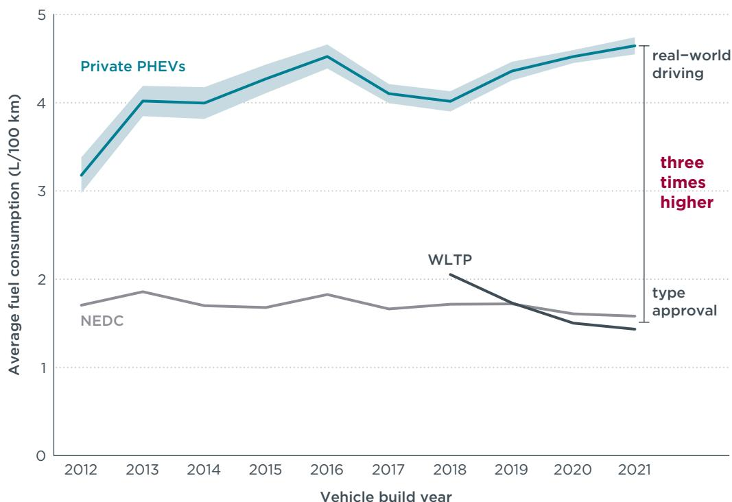
**Figure 1.** Development of the average real-world and type-approval fuel consumption of private PHEVs in Europe over vehicle build year. Shaded area indicates 95% confidence intervals for the mean.
