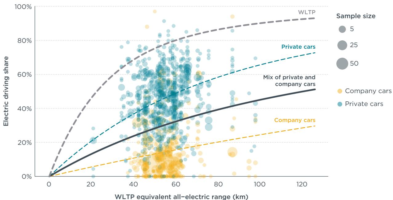
**Figure ES3.** Real-world electric driving share compared to WLTP assumption on charge-depleting mode driving share.
