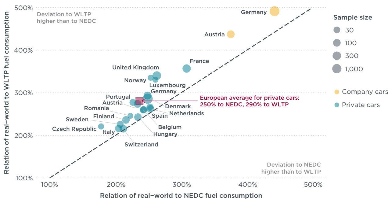
**Figure 5.** Mean relation of real-world to NEDC and WLTP type-approval fuel consumption by country sample.
