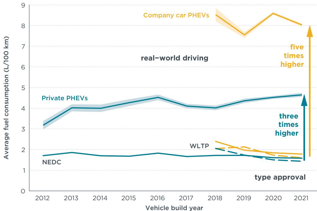
**Figure ES1.** Development of the average real-world and type-approval fuel consumption of private and company car PHEVs in Europe over vehicle build year. Shaded areas represent 95% confidence interval from sample size uncertainty.
