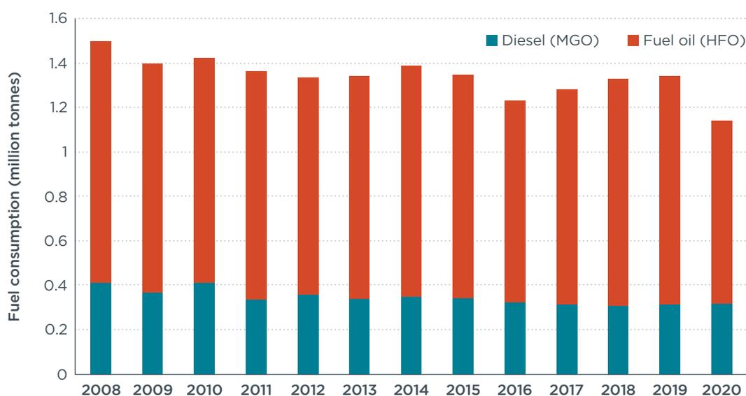
**Figure 9.** Estimated fuel consumption in cabotage activities between 2008 and 2020
