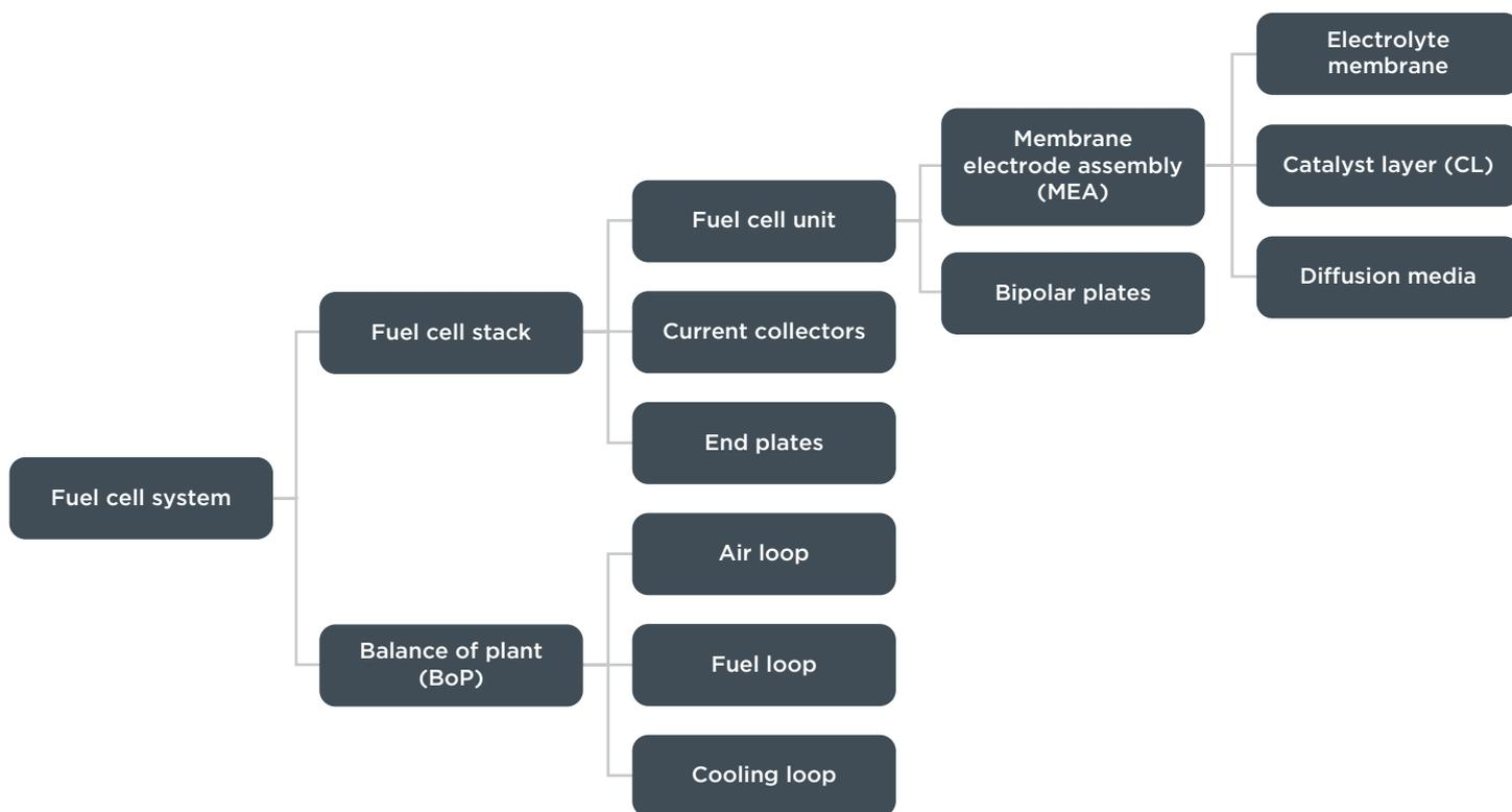
**Figure 2.** Fuel cell system components
