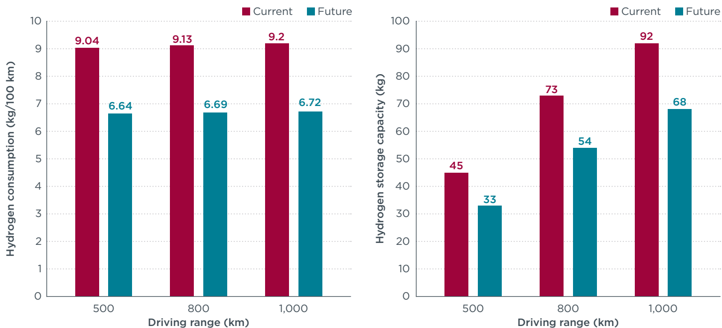
Figure 10. Fuel cell electric truck hydrogen fuel consumption (left) and required hydrogen tank size (right) for different driving ranges simulated over the VECTO long-haul drive cycle at a reference payload of 19,300 kg and 15°C ambient temperature for current and future vehicle technologies.
