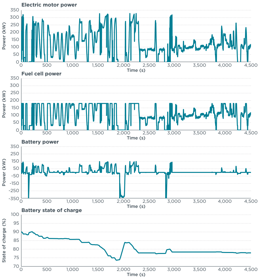
Figure A2. Electric motor, fuel cell system, and battery power profiles and state of charge as a function of time simulated over the VECTO long-haul drive cycle at a reference payload of 19,300
