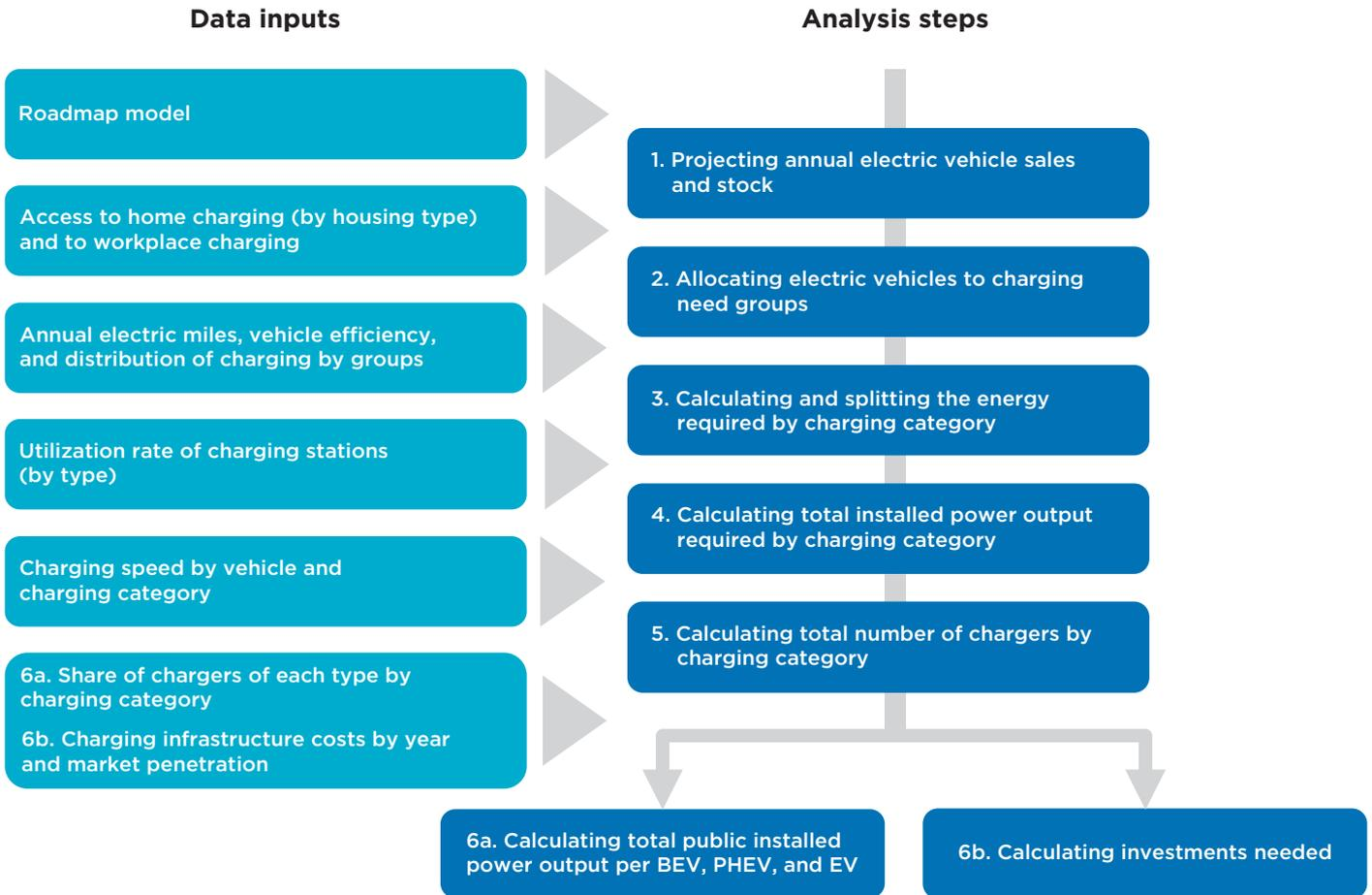
**Figure A1.** Charging infrastructure modeling for light-duty vehicles.
