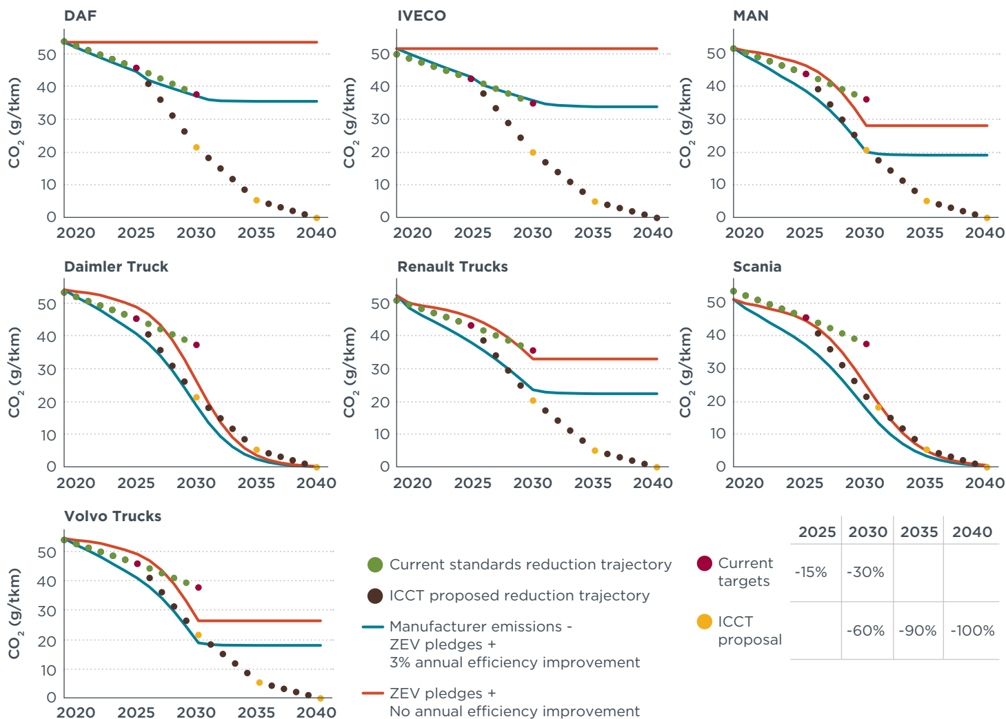
Figure 1. Manufacturer CO 2 emission trajectories based on announced pledges towards zero-emission vehicles and assuming a 3% annual efficiency improvement. The ICCT proposed trajectory reflects emissions reductions of 60% in 2030, 90% in 2035, and 100% in 2040.
