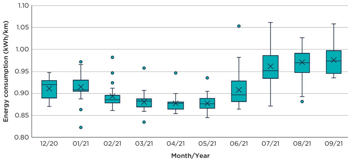
**Figure 7.** Box diagram of energy consumption per kilometer traveled
