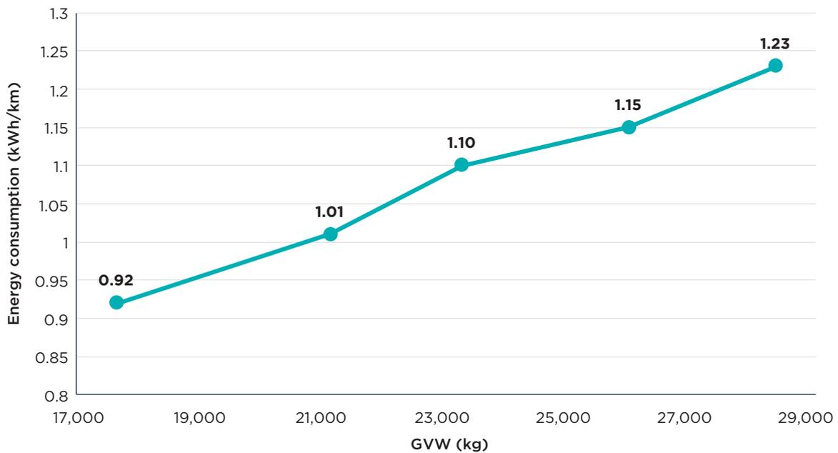
**Figure 13.** Measured energy consumption for each load scenario
