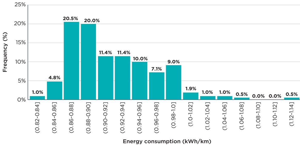
**Figure 6.** Histogram of energy consumption per kilometer traveled
