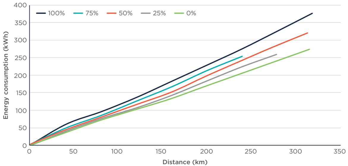
**Figure 12.** Energy consumption (kWh) vs distance for each load scenario
