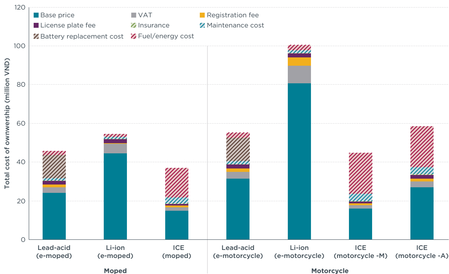
Figure 4. TCO of 7 selected models at 5 years of operation (with batteries purchased for E2W models)
