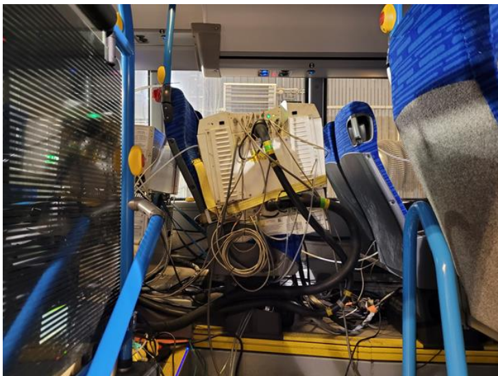
Figure 3-10 PEMS-installation in vehicle 2
