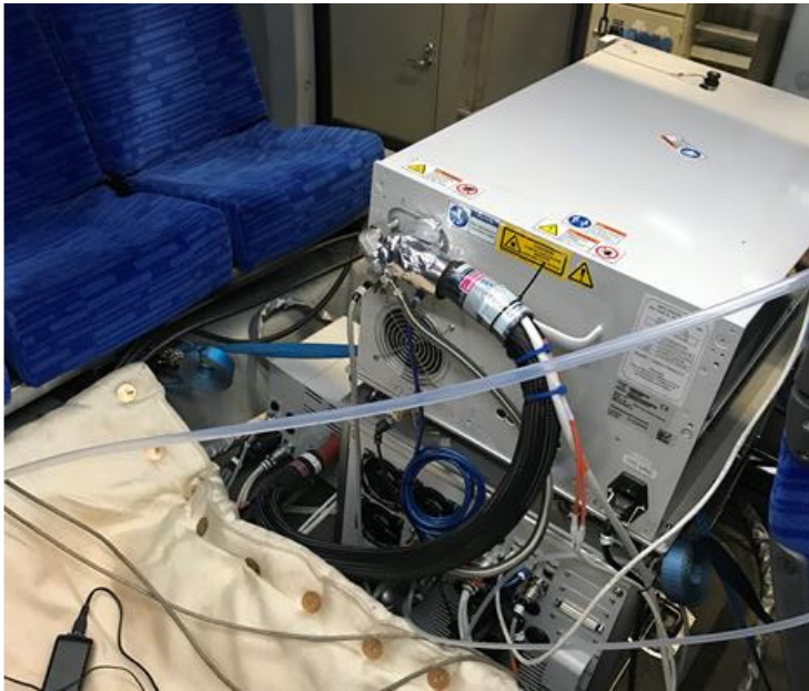
Figure 3-11 FTIR-installation in vehicle 2
