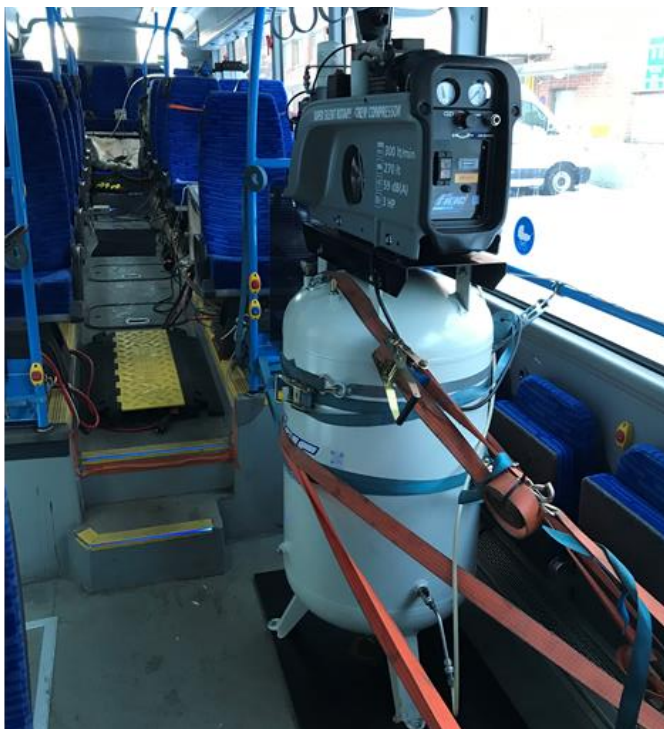
Figure 3-12 Air compressor for CPC dilution air
