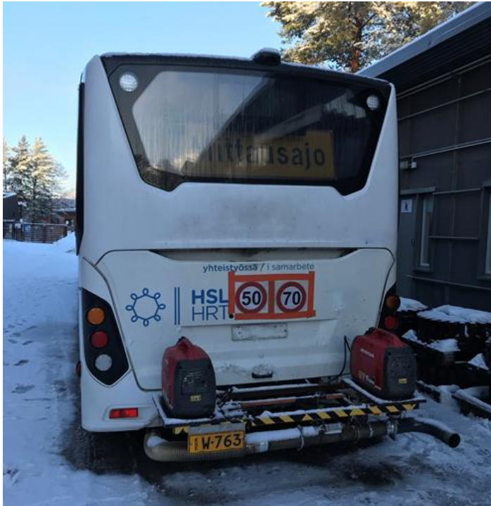
Figure 3-15 Generator assembly in vehicle 2 for supplying electric power for the measurement equipment
