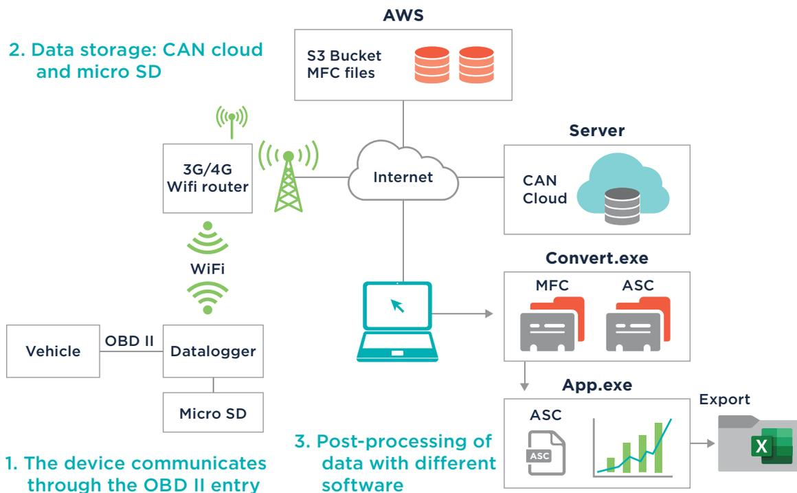
**Figure 17.** Data collection and storage structure for monitored electric vehicles
