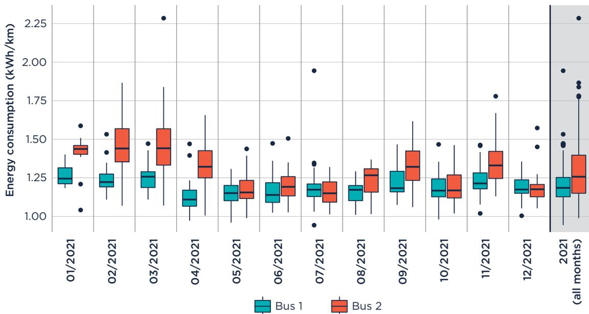
**Figure 6.** Daily energy consumption per kilometer over the monitored months, aggregated for 2021
