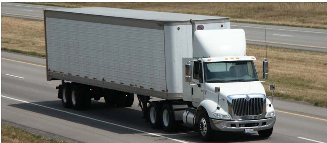
Figure 14. A short-haul tractor truck with a trailer attached
