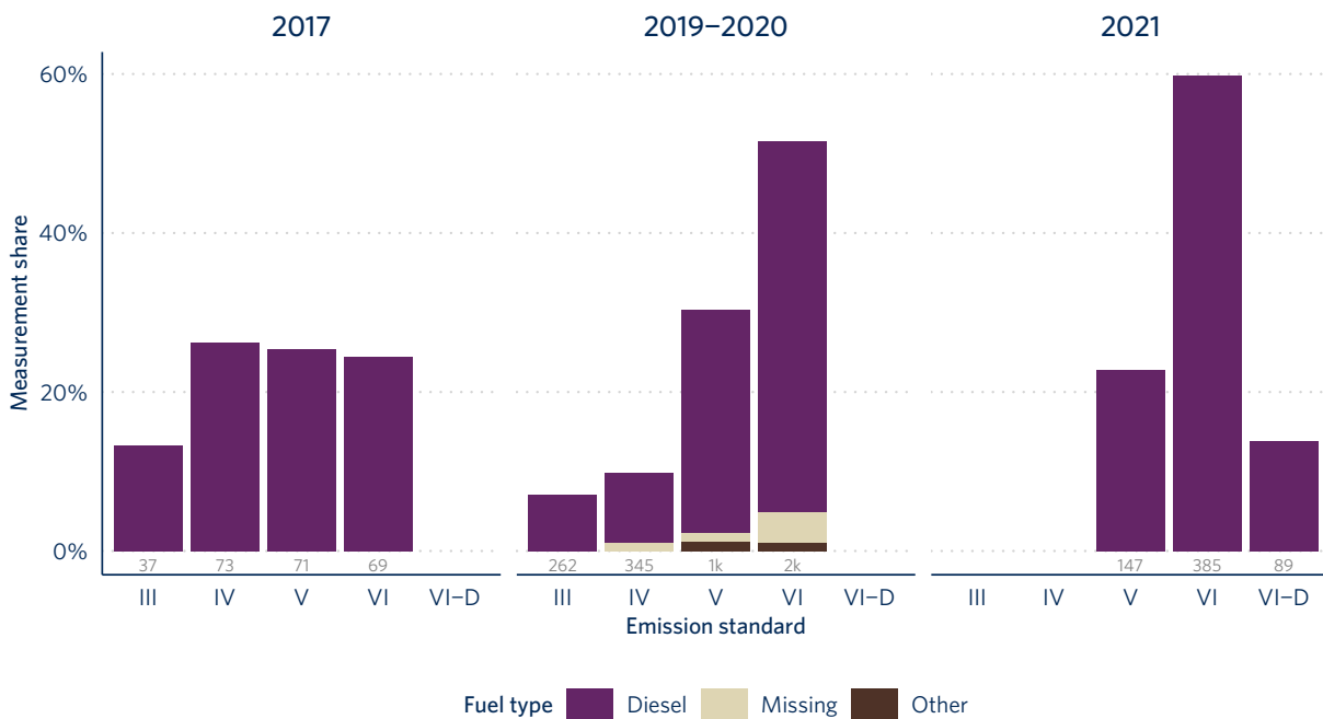
Figure 40. Distribution of fuel types and Euro standards of buses measured in 2017, 2019-2020, and 2021. Only measurements of 30 or more are presented. Measurements with the fuel type “other” are all diesel hybrid buses.
