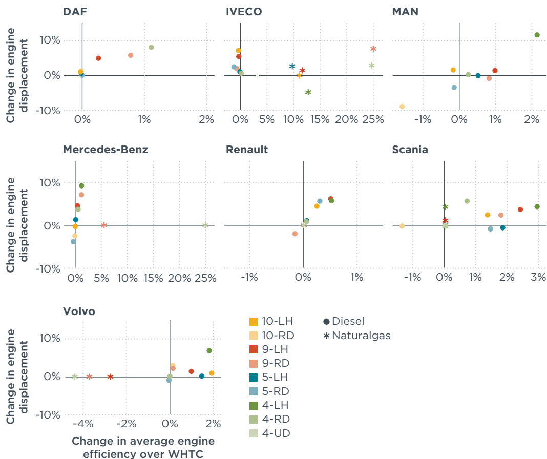
Figure 9. Changes in average engine efficiency over WHTC relative to changes in displacement over the reporting periods 2019 and 2020.
