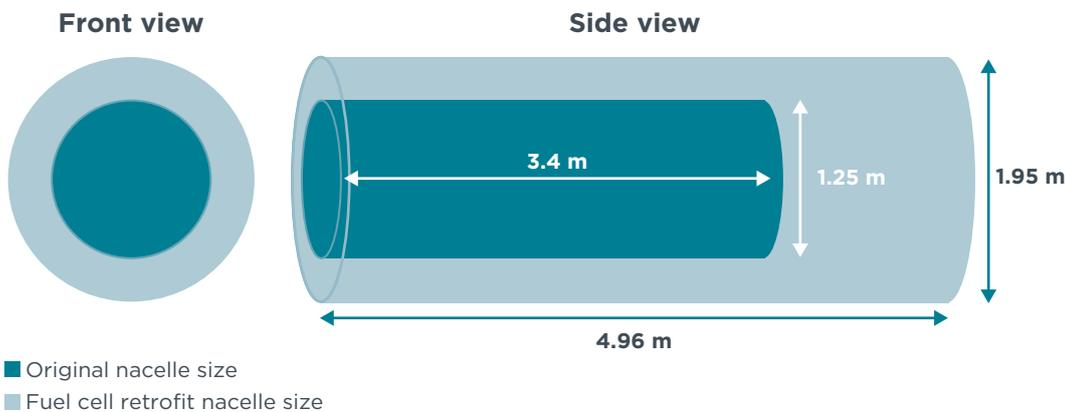
**Figure 2.** Comparison of the nacelle sizes.
