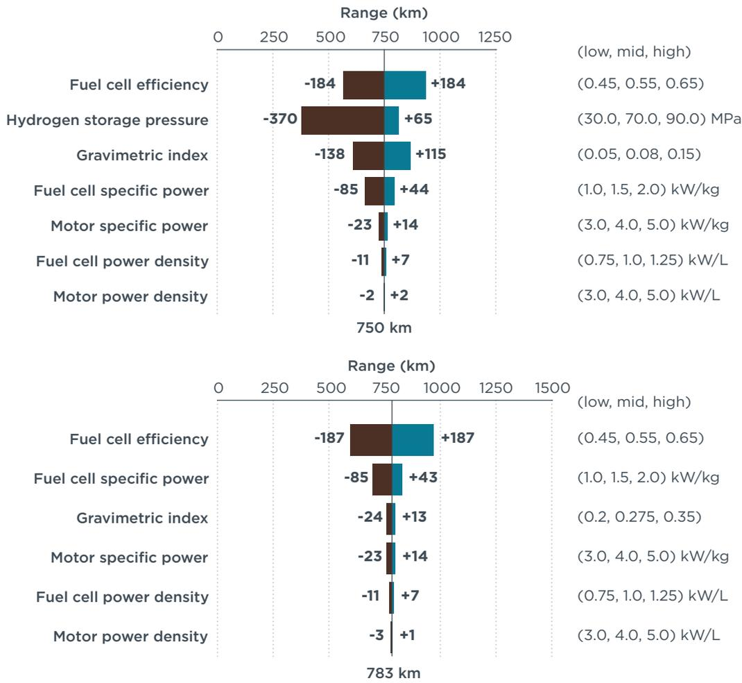
**Figure 12.** Sensitivity analysis of aircraft range. Top: GH<sub>2</sub> aircraft with 50 passengers. Bottom: LH<sub>2</sub> aircraft with 58 passengers.
