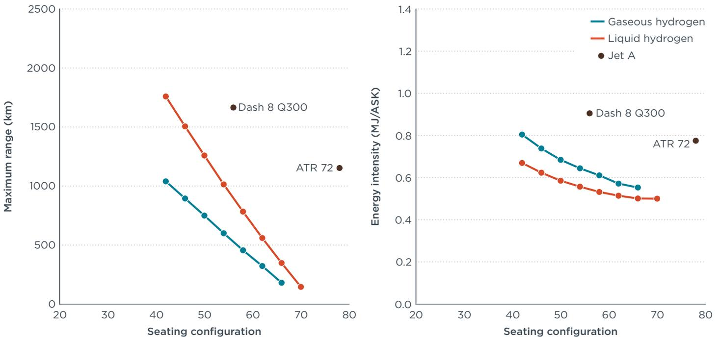
Figure 8. Maximum range (left) and energy intensity (right) of the fuel cell retrofit aircraft.
