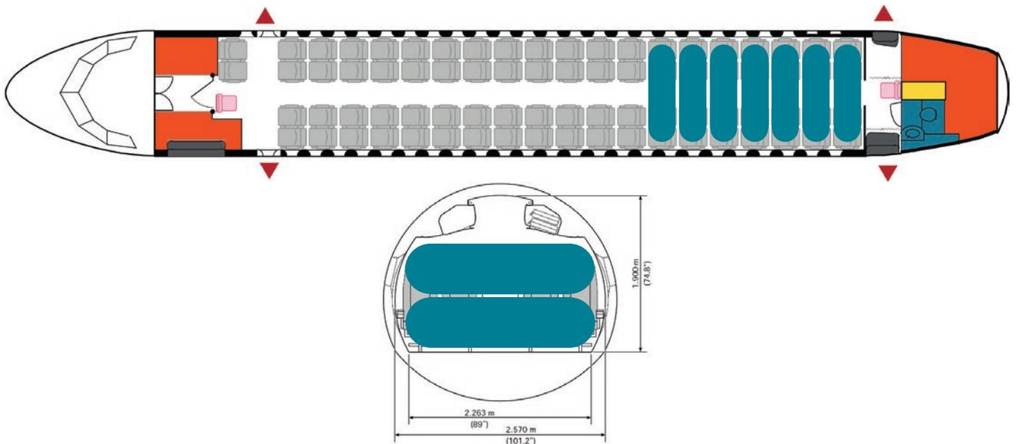
**Figure 3.** Illustrative tank layout of a retrofitted ATR 72 for 50 passengers.
