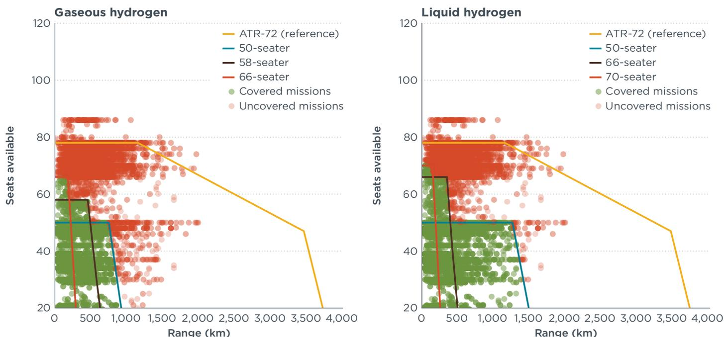
**Figure 9.** Turboprop routes flown in 2019 compared to the payload-range capability of fuel cell aircraft retrofits.
