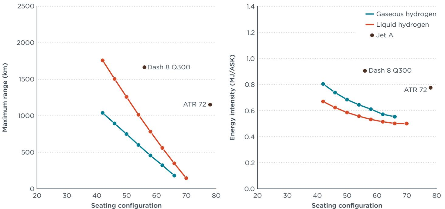
**Figure ES 1.** Maximum range (left) and energy intensity (right) of a fuel cell retrofit aircraft.
