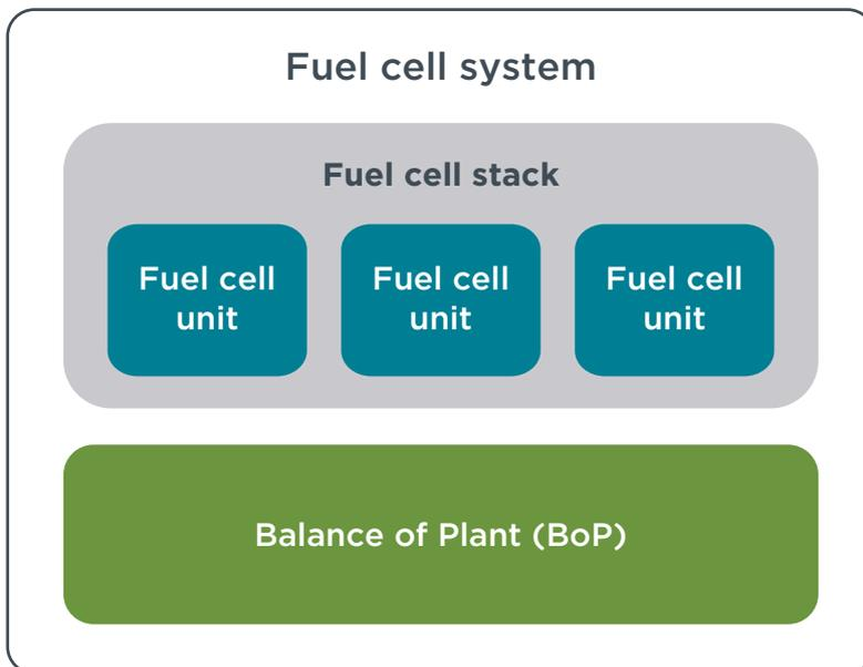
**Figure 1.** Schematic of a fuel cell system.
