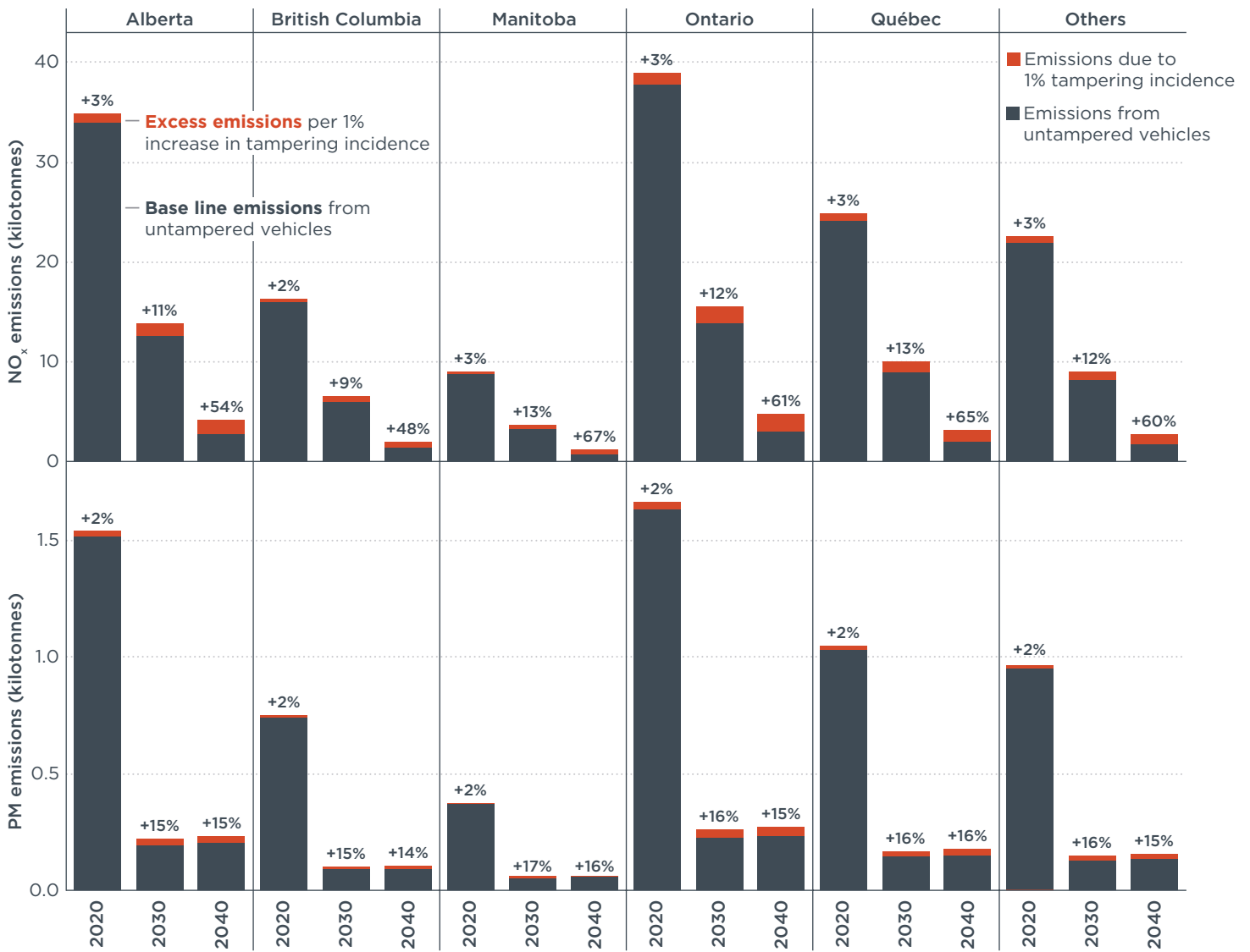
Tailpipe NO x and PM emissions from medium- and heavy-duty vehicles by province in 2020, 2030, and 2040 (kilotonnes). Dark segments show baseline emissions under a scenario without tampering. Light segments indicate the percent increase in emissions associated with a 1% increase in the number of tampered vehicles on the road.
