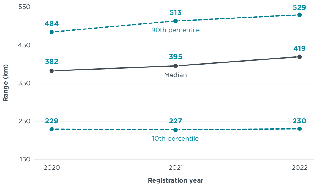
Figure 1 Evolution of the WLTC-defined range for passenger cars registered in the EU, 2020–2022
