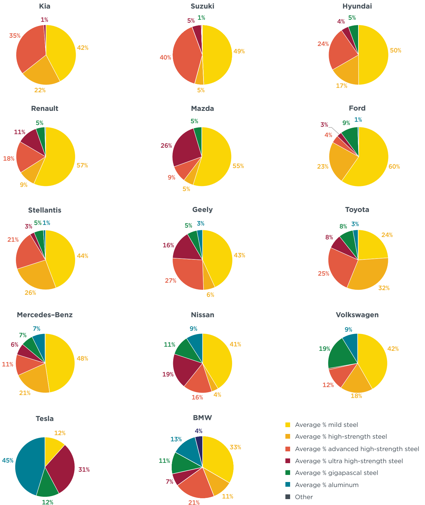
Figure 4 Relative average shares of materials used in the vehicle body, by manufacturer
