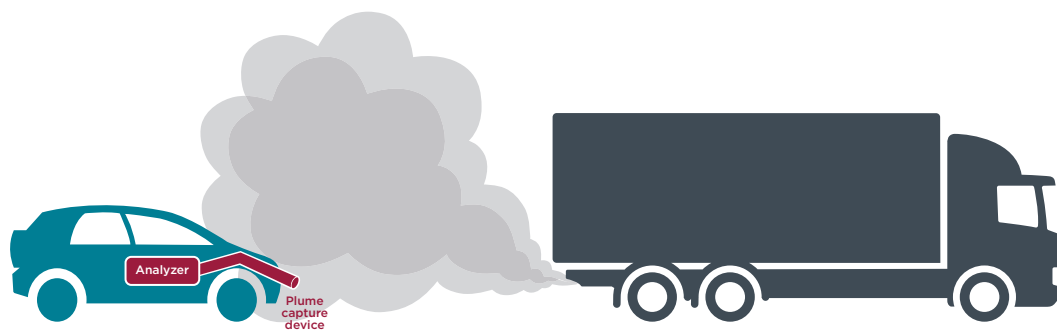
Figure 1. Plume chasing data collection technique
