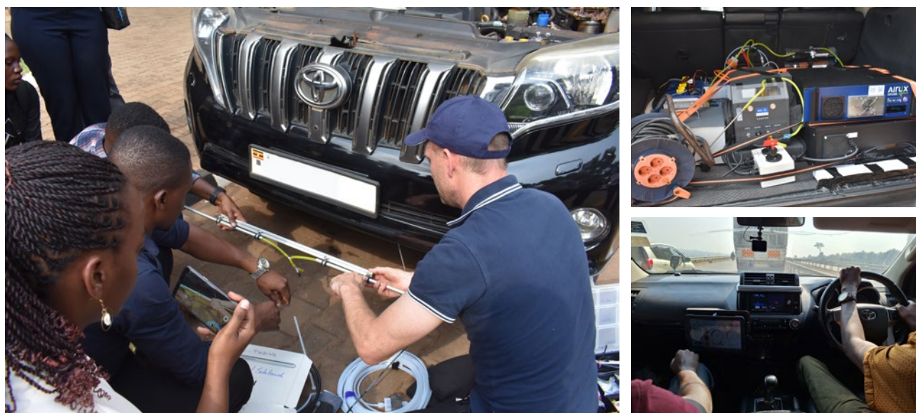
Figure 2. Plume chasing vehicle setup in Kampala
