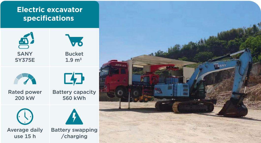
Figure 2.5.1. Specifications and application of the SY375E electric excavator at the mining site in Honghe Prefecture
