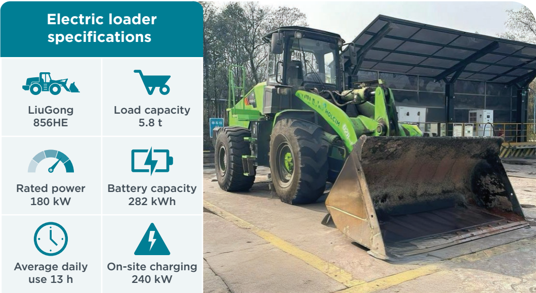
Figure 3.1.1. Specifications and application of 856HE electric loaders in the cement plant in Chengdu
