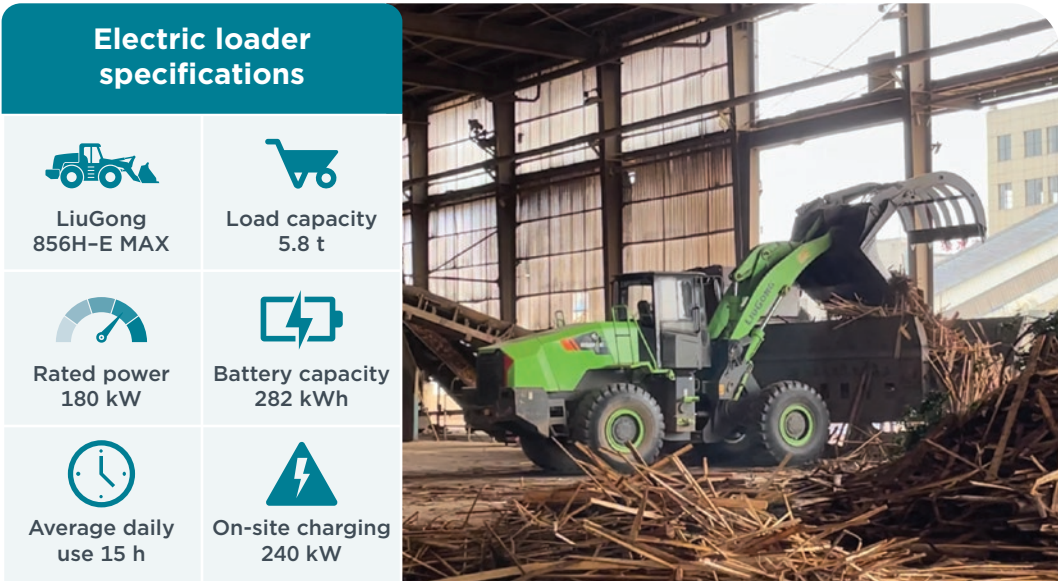
Figure 3.2.1. Specifications and application of 856H-E MAX electric loaders in the Liuzhou biomass power plant
