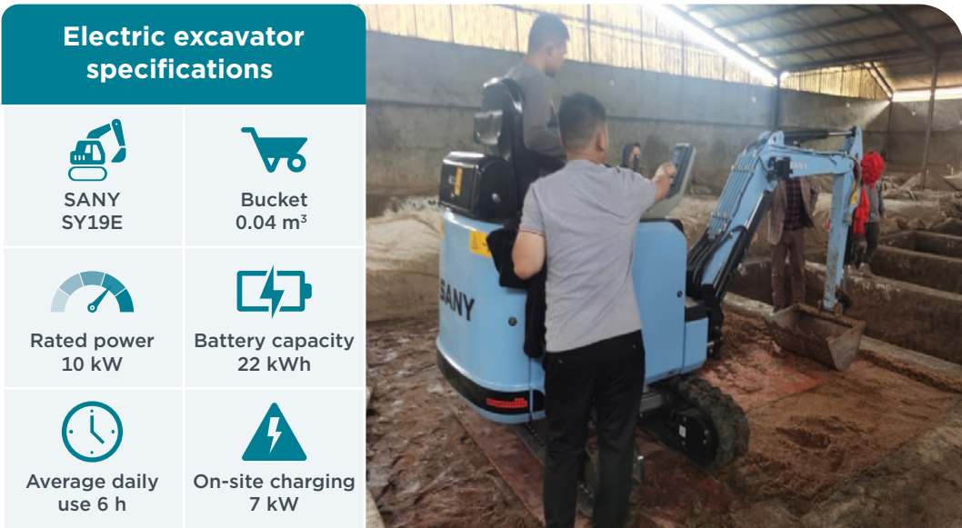
Figure 2.1.1. Specifications and application of the SY19E electric excavator in the Chengdu distillery
