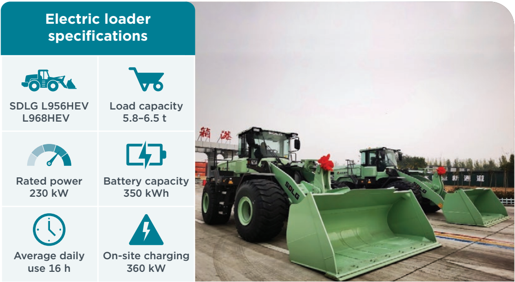
Figure 3.3.1. Specifications and application of L956HEV and L968HEV electric loaders at Liangshan Port
