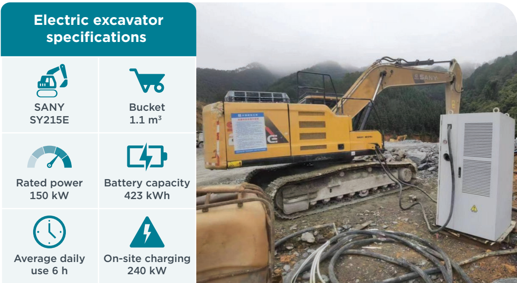
Figure 2.4.1. Specifications and application of the SY215E electric excavator in Xichang tunnel project
