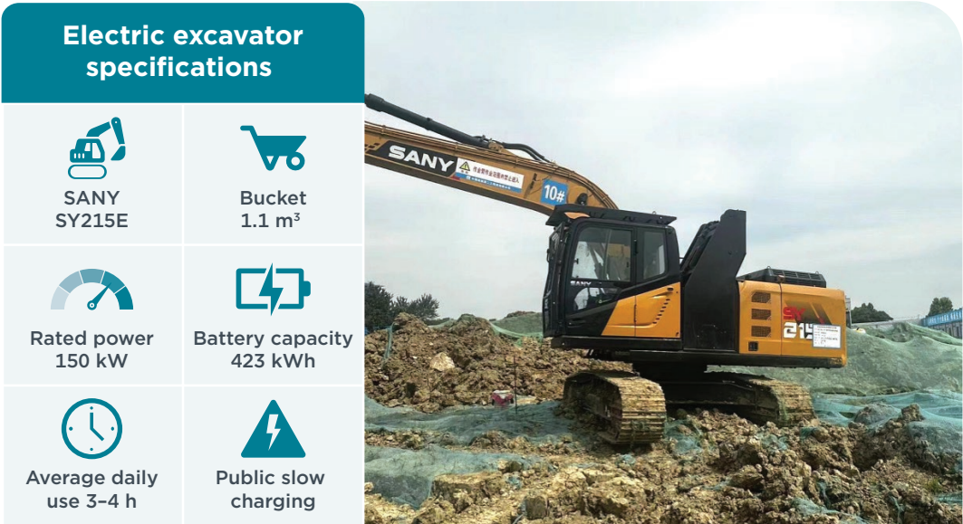
Figure 2.2.1. Specifications and application of the SY215E electric excavator at the building construction site in Wuxi
